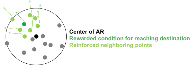
Figure 5.26: Reinforcing neighbors of the rewarded condition within an AR to aid the pathfinding process and also introduce further variability to the stochastic search.
