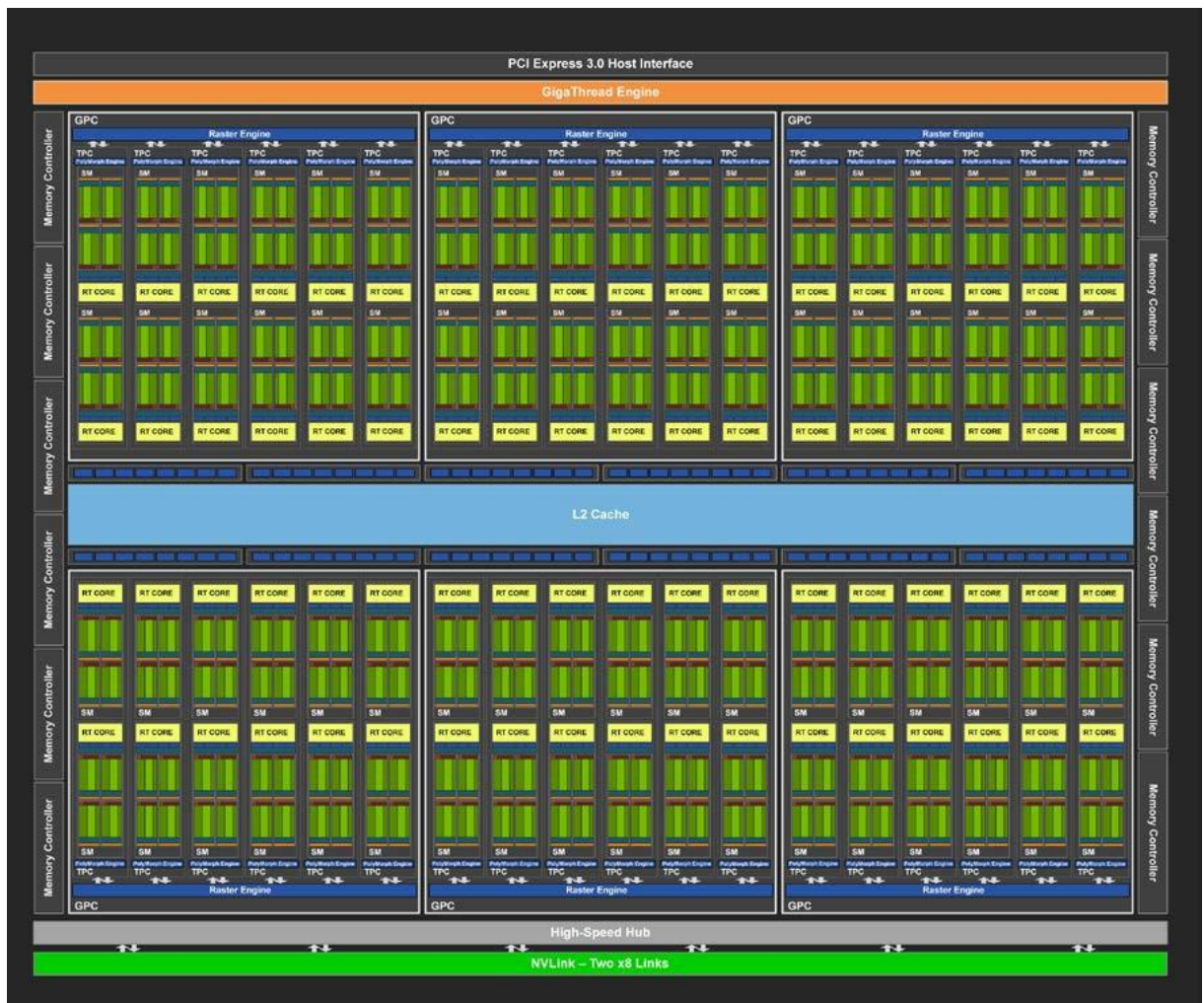
Figure 3: Turing TU102 full GPU with 72 SM units.
