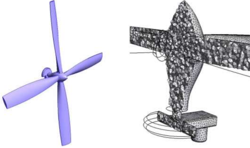
Figure 1. Propeller and its mesh in Gmsh [4].
