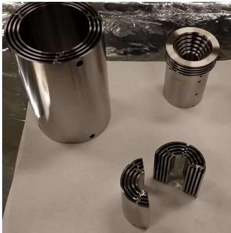
Figure 3.14. The three banks of concentric radiation shields used in the Z-Meter. The upper bank for the ceramic loading shroud (CLS) also serves as the mount for the upper bar shield.
