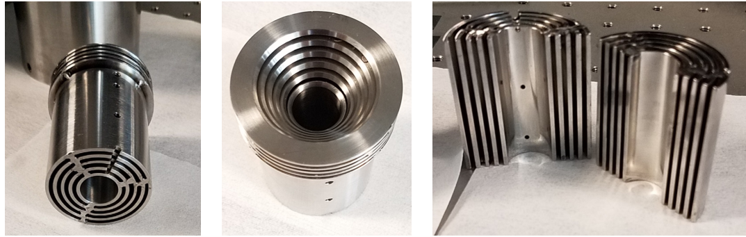
(a) Upper Bar Heat Shield - Bottom View (b) Upper Bar Heat Shield - Top View (c) Lower Bar Heat Shield - Split
