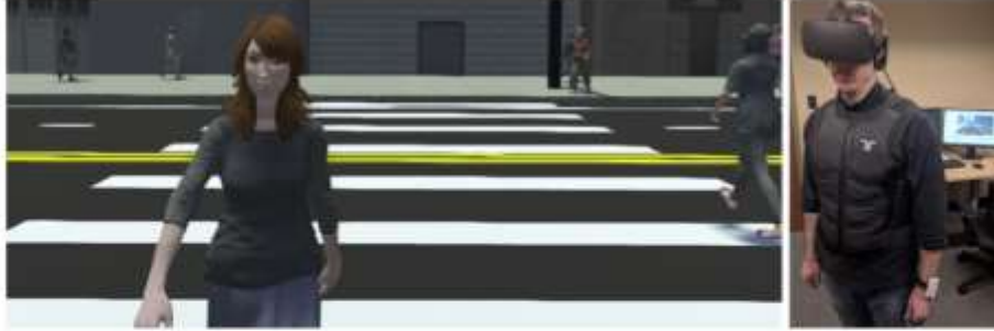
Figure 2: The virtual environment that was used for the purpose of this study (left), participant wearing HMD, haptic vest, and GSR sensor (right).
