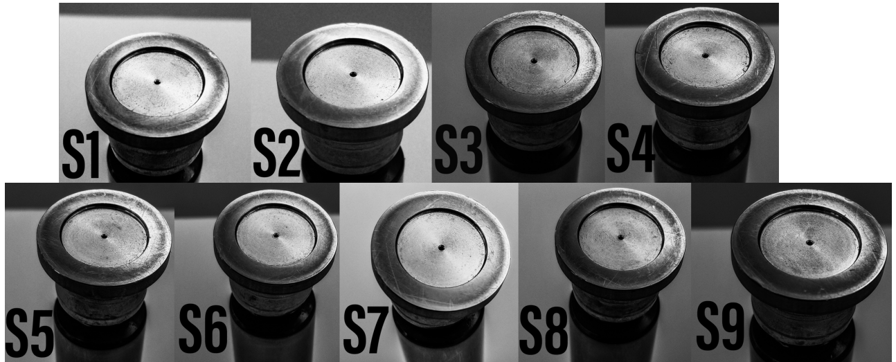
Fig. 5.4.: Similar wear pattern on the slipper surfaces
