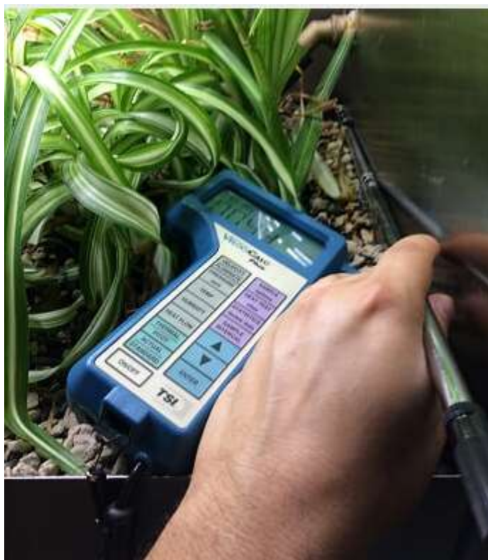
Figure 3.5 Hot Wire Anemometer (TSI VELOCICALC Plus 8386) used to record air velocity readings through the Biowall.
