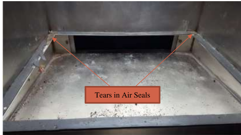
Figure 3.7 Biowall plant shelf with tray removed following Treatment 1. The arrows point to tearing in tray air seals.
