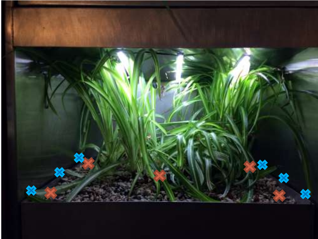
Figure 3.6 Initial air measurement positions per tray indicated with an X. Red). Measurement within the tray. Blue). Measurement outside the tray.
