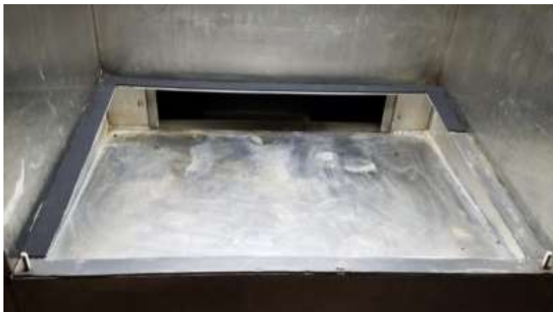
Figure 3.8 Tray 2 following Treatment 2 showing replacement of torn air seal insulation.
