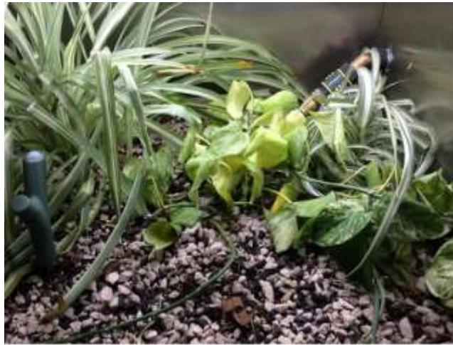
Figure I.1 A plant tray following 14 days of continuous air through the roots shows plants deprived of moisture.
