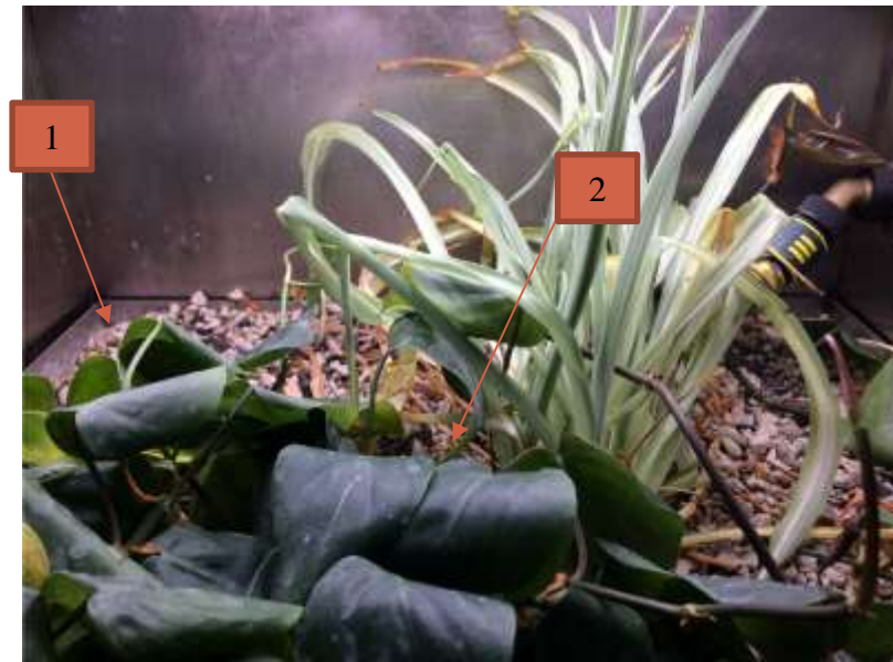
Figure 3.3 Tray 4 at an initial condition shows varying growth medium depths. (1) minimum, (2) maximum growth medium depth.
