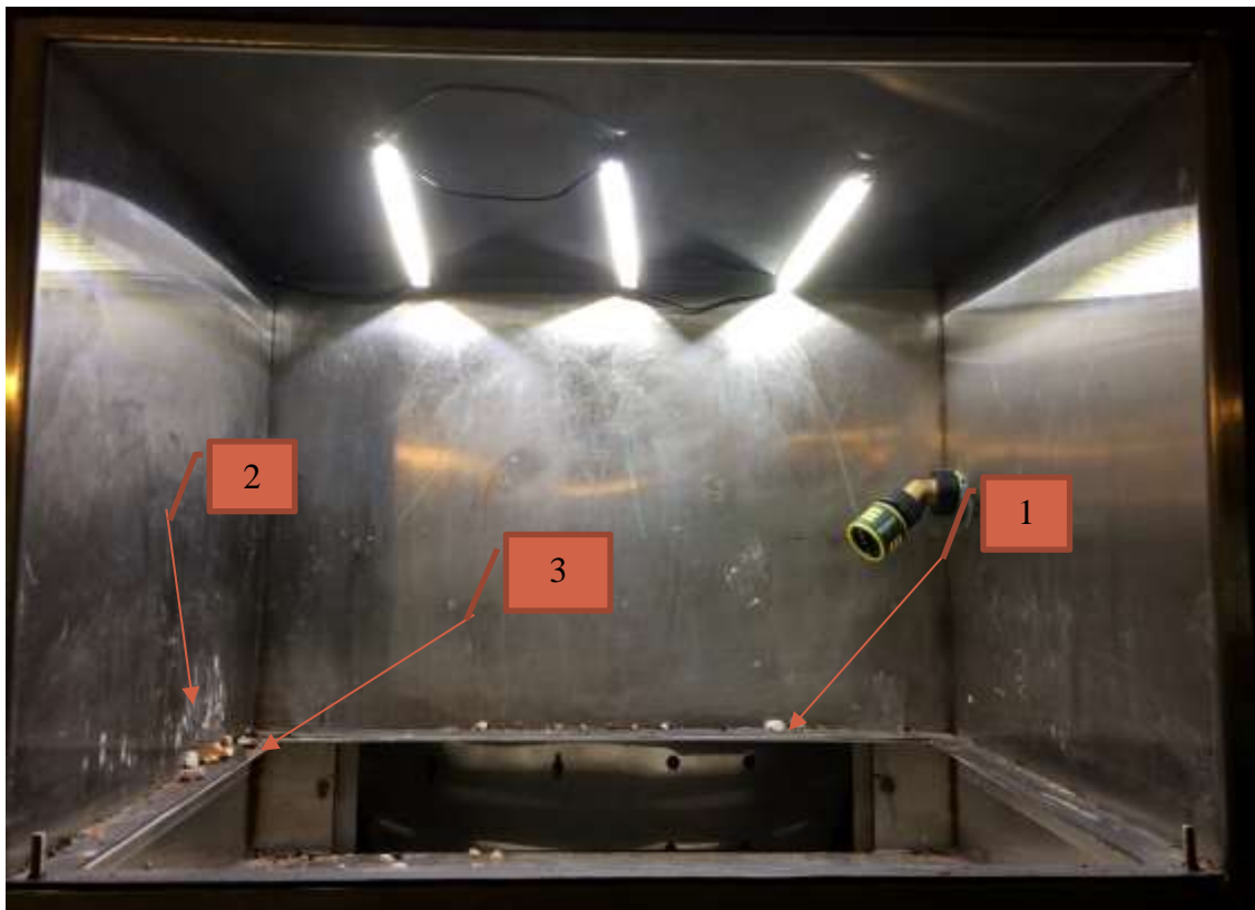
Figure 3.4 Biowall shelf 4 with tray removed: 1). Growstone obstructing air seal. 2). Signs of Growstone wedged against the housing. 3). Damaged/torn air seals.
