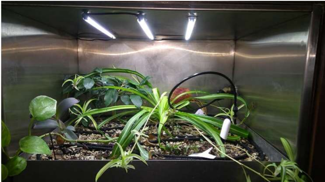
Figure 4.5 Biowall plant tray with optimized irrigation hose configuration.
