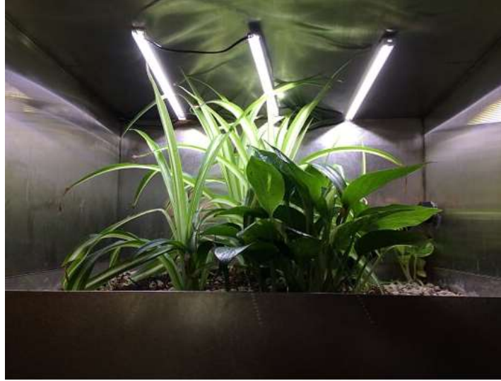
Figure 2.7 A single Biowall plant tray shelf with broad-spectrum plant growth LEDs.
