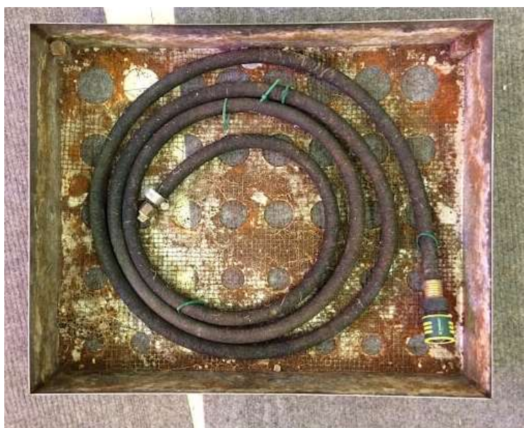
Figure 3.13 Tray 3 with growth medium removed after initial assessment reveals the irrigation soaker hose condition.
