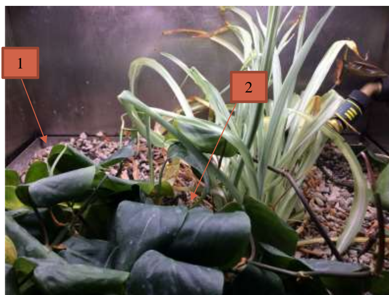
Figure 3.9 Tray 4 during the initial assessment shows that the growth medium within the plant tray has inconsistent depths.
