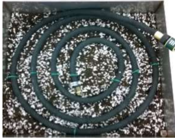
Figure 2.6 Biowall plant tray and soaker hose orientation.
