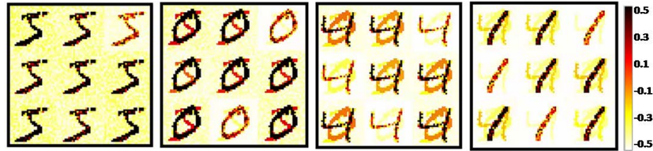
Fig. 5.5. Digit representations learnt with isolated weight decay learning in an SNN with 9 excitatory neurons connected to input layer (28x28 pixels). The input digits are presented sequentially (i.e. dynamic environment with no data-reinforcement). The network is overly plastic and adaptive to the continually changing inputs.
