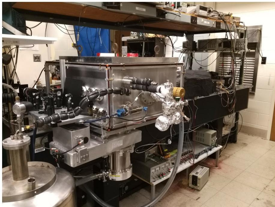
Fig. 3.23. Photo of the vacuum chamber in our laboratory. The turbopump and gate valve can be seen attached to the bottom of the vacuum chamber.
