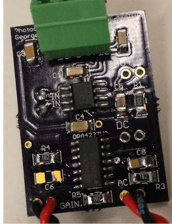
Fig. 4.2. Photograph of the tiny PCB holding the OPA827 TIA and OPA4227 quad op-amp. The PCB is only  $1.4 \times 1.1$  in<sup>2</sup>.
