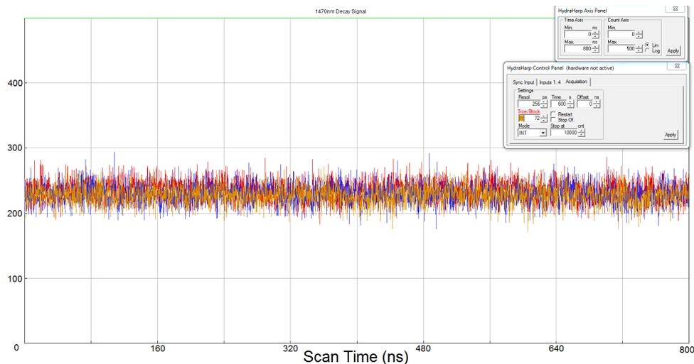
Fig. 6.5. A test of the SPD background photon count while the 1079 nm laser is pulsed through the vapor cell but tuned off-resonance. The SPD is running in gated mode, and triggered asynchronously from the laser pulses. This screen capture of the TCSPC software shows the data from three different runs, each of length 10 minutes. We conclude that the number of background photon counts is very uniform while using the gated-SPD in asynchronous mode.
