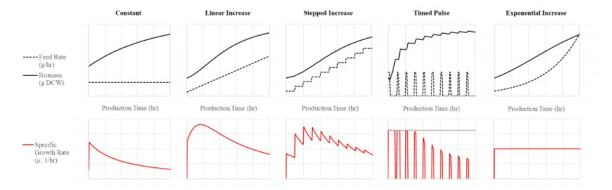
Figure 6: Feed rate with hypothetical Biomass, and growth rate of various feed-forward feeding methods. While the units of these graphs are arbitrary, in the event sufficient data is known correlating growth rate and protein productivity, these trends can be useful for selecting a feeding strategy for investigation. These trends were developed in the Maple computing environment [Maplesoft, 2018]. The equations and code used to create these can be found in Appendix A
