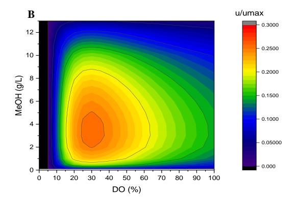
Figure 5: Surface plot of bivariate *Pichia* growth model against methanol and dissolved oxygen;
