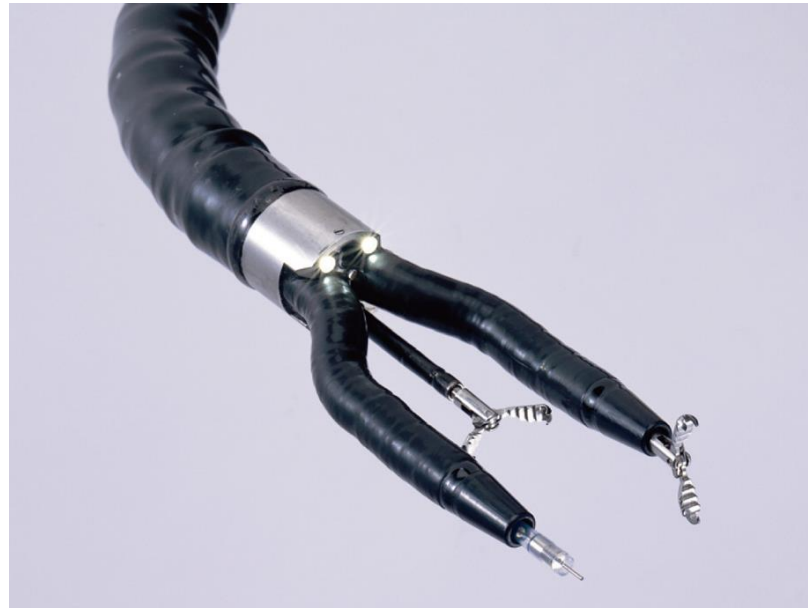
Figure 2.7. 5-DOFs Direct Drive Endoscopic System [22].
