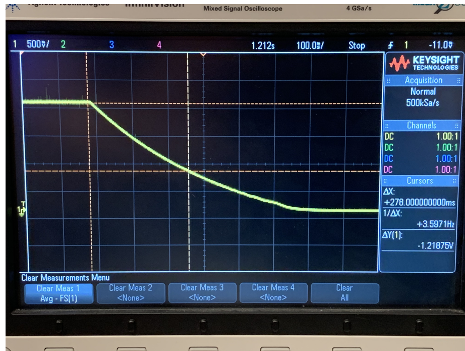
Figure 5.4. Motor Voltage drop after power supply is shut down.
