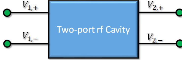
Fig. B.1. A diagram of a two-port cavity with V_{n,+} representing the incident voltage while V_{n,-} is the reflected one.
