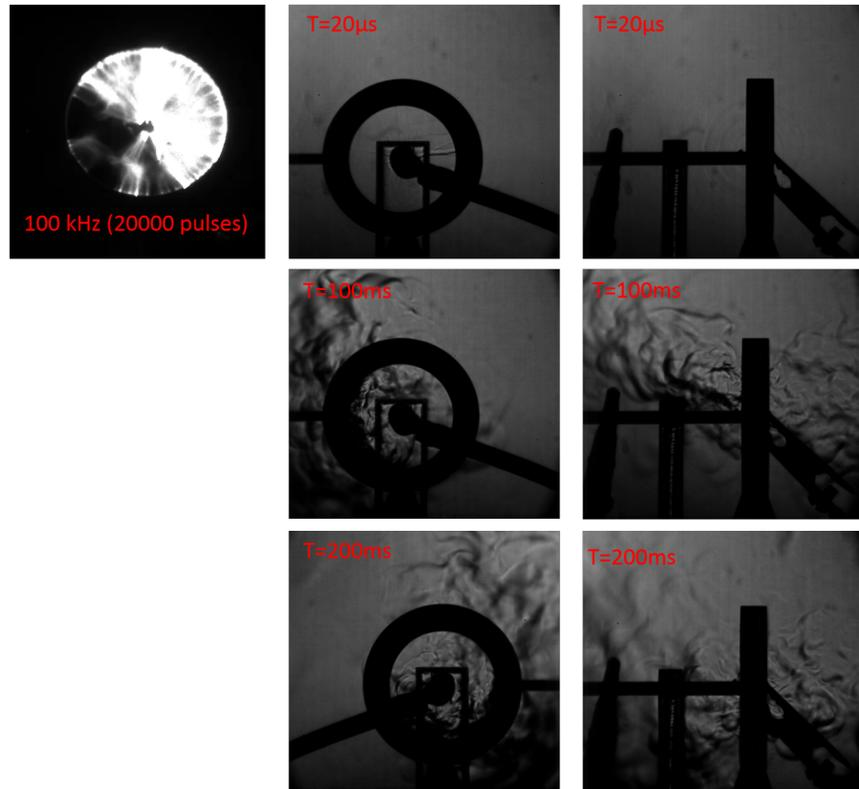
Fig. 3.11.: Long exposure iccd image for a 200ms discharge at 100kHz and gas expansion observed through schlieren at different intervals of time
