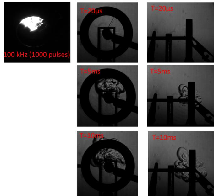
Fig. 3.10.: Long exposure iccd image for a 10ms discharge at 100kHz and gas expansion observed through schlieren at different intervals of time
