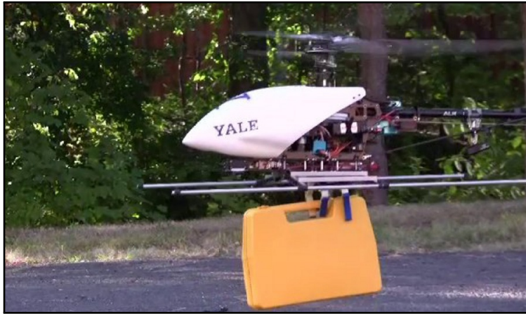
Figure 1.4. : Yale Aerial Manipulator carrying a toolcase [35].
