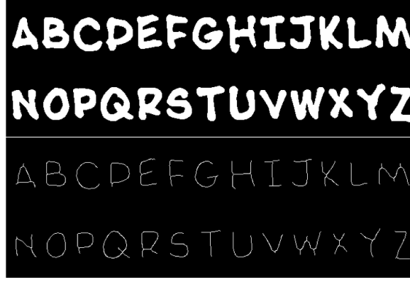
Fig. 4.2.: An example of applying Zhang-Suen thinning algorithm.
