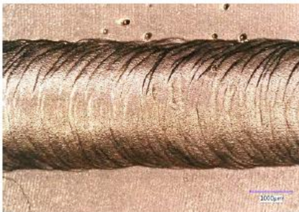
Figure 4.5 Keyence digital microscope images showing the typical appearance of the WPS1 pulsed laser weld.
