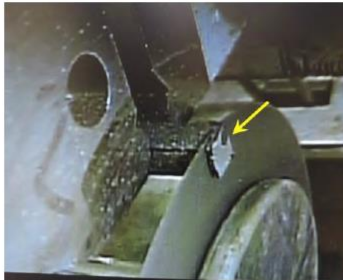
Thin cross sectional slice being cut off weld using ultra thin specialty blade - the thin slice (marked with a yellow arrow) is nearly complete.
