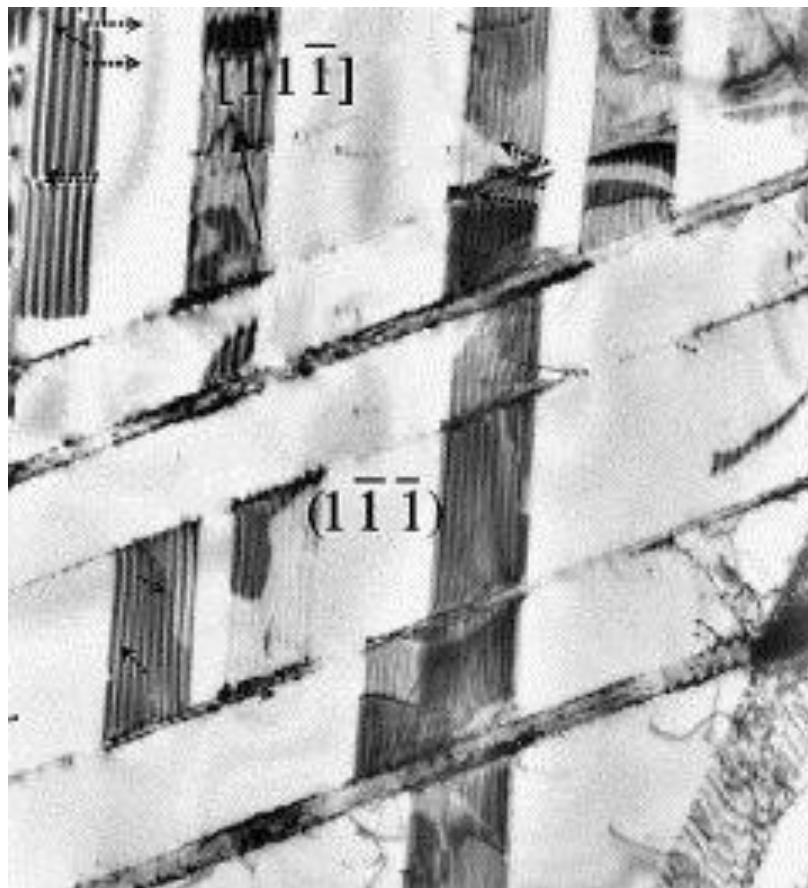
Figure 2.25 Stacking faults of 316LN SS after 8% strain deformation from disk bending at 150 °C [232].
