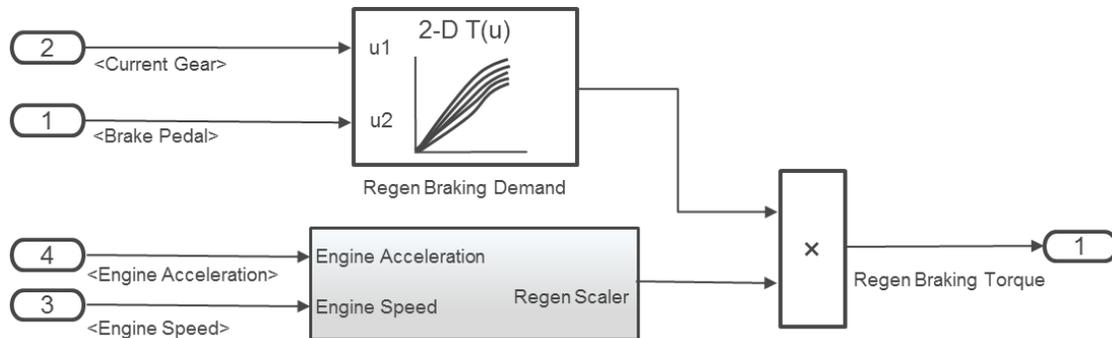
Figure 3.11 Matlab® Simulink® Based Regenerative Braking Logic Implementation
