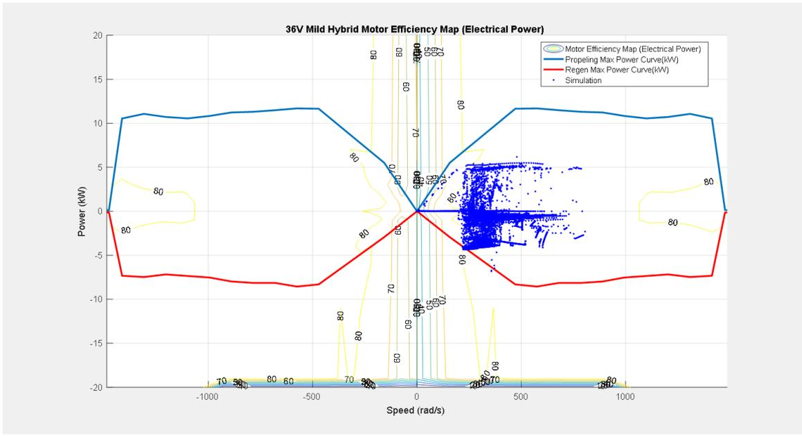
Figure 4.12 36V Mild Hybrid Motor Efficiency Map (Simulated)
