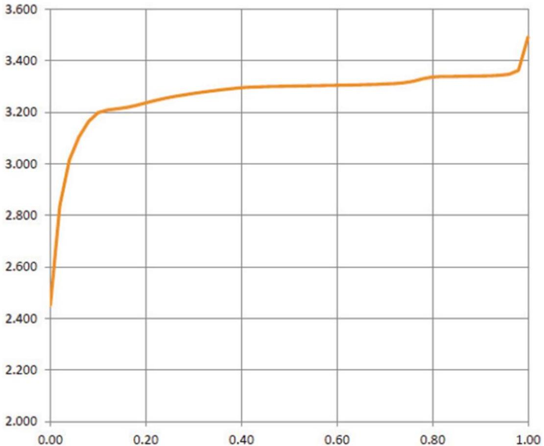
Figure 3.16 Cell Open Circuit Voltage vs. SOC (A123®, 2017)
