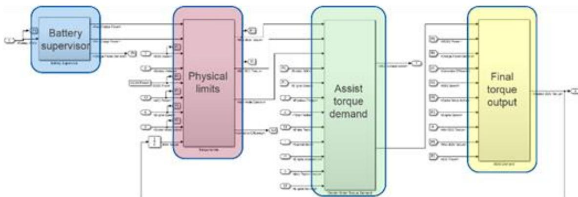
Figure 3.12 Matlab® Simulink® Based Torque Assist Logic
