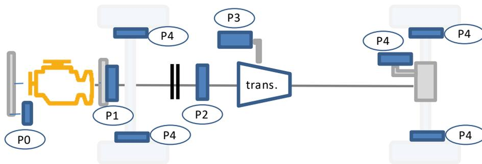
Figure 2.8 Mild Hybrid Electric Vehicle Architecture
