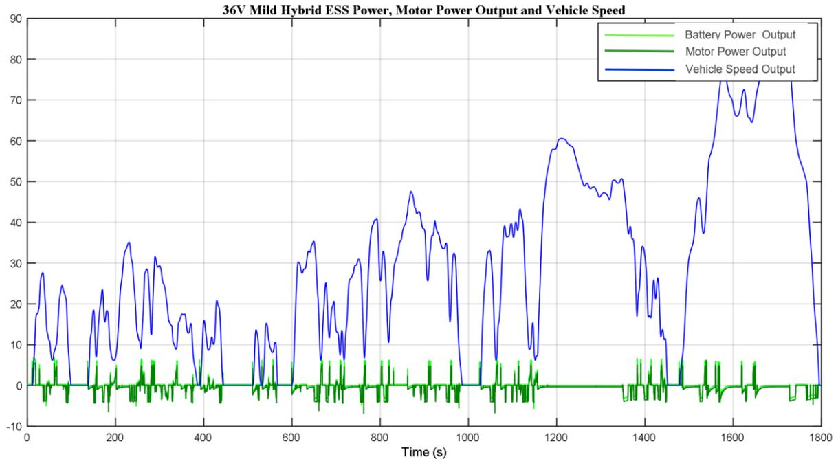
Figure 4.10 36V Mild Hybrid Battery and Motor Electric Power Output vs. Vehicle Speed (Simulated)
