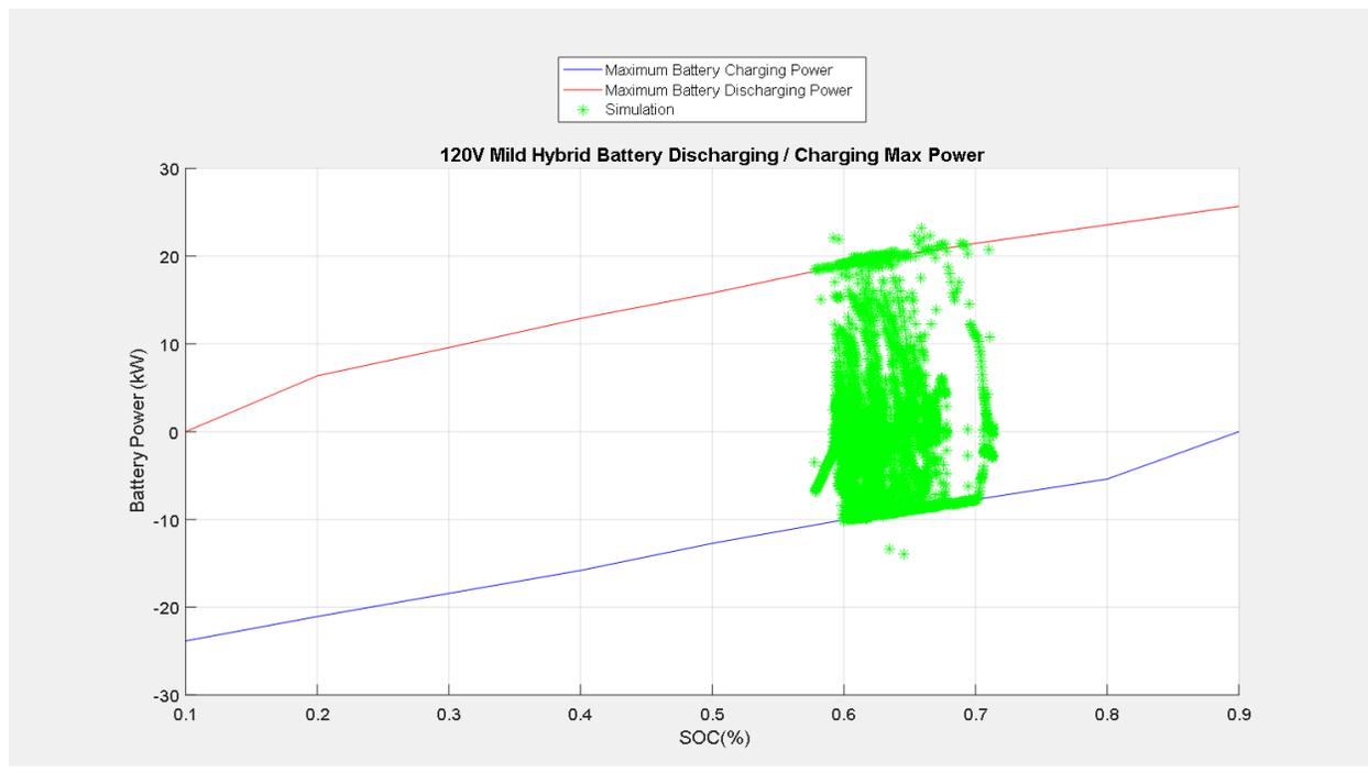
Figure 4.20 120V Battery Discharging / Charging Max Power (Simulated)
