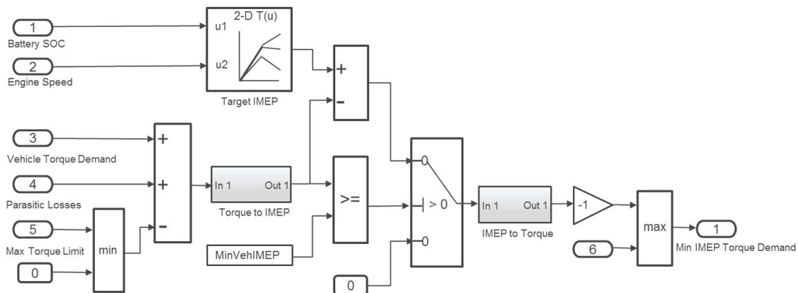
Figure 3.13 Matlab® Simulink® Based Minimum Indicated Mean Effective Pressure (IMEP) Logic
