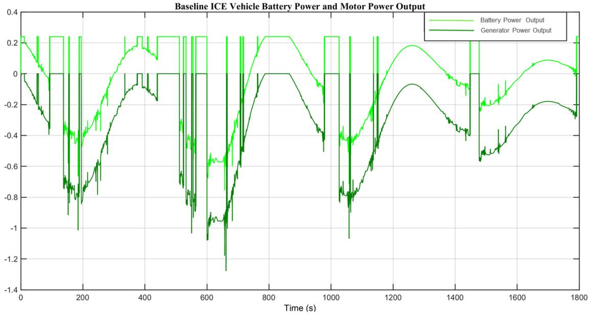
Figure 4.5 Baseline Conventional ICE Vehicle Battery Power Output (Simulated)
