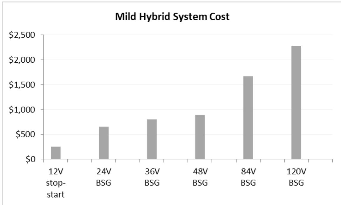
Figure 3.29 Mild Hybrid System Cost Chart
