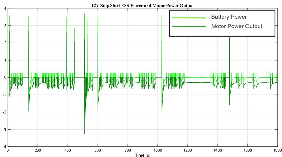
Figure 4.6 12V Stop Start Battery and Motor Electric Power Output (Simulated)
