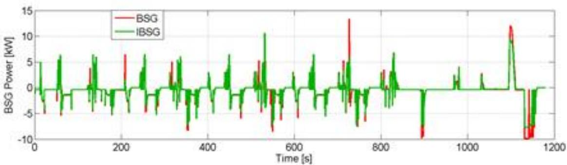
Figure 3.22 Electric Machine Power Output over NEDC Drive Cycle (Simulated)
