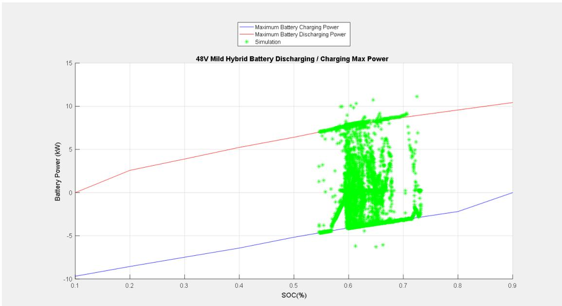
Figure 4.14 48V Battery Discharging / Charging Max Power (Simulated)
