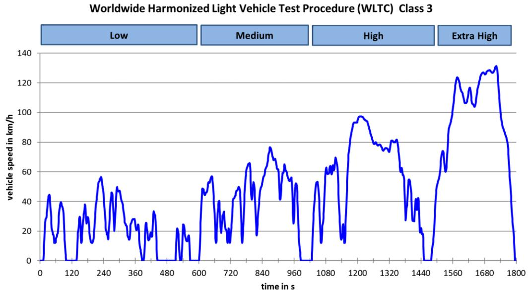
Figure 4.3 Worldwide Harmonized Light Vehicle Test Procedure (UNECE Global technical regulation No 15, 2014)
