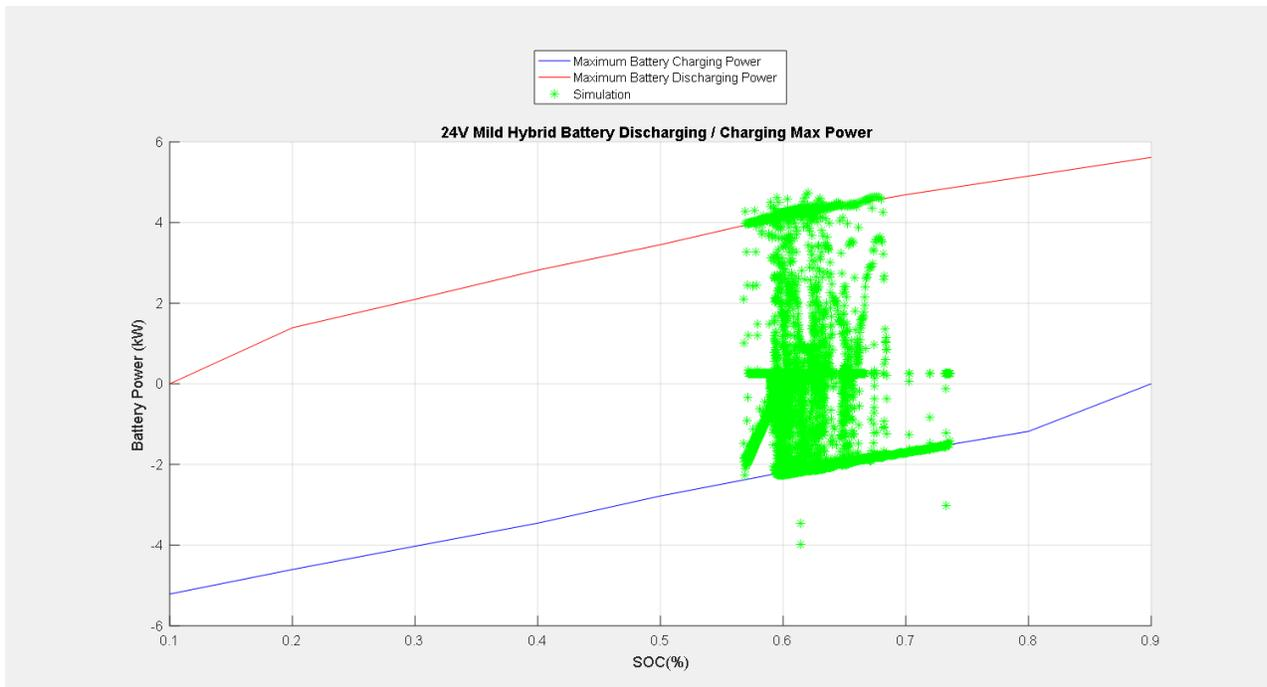
Figure 4.8 24V Battery Discharging / Charging Max Power (Simulated)
