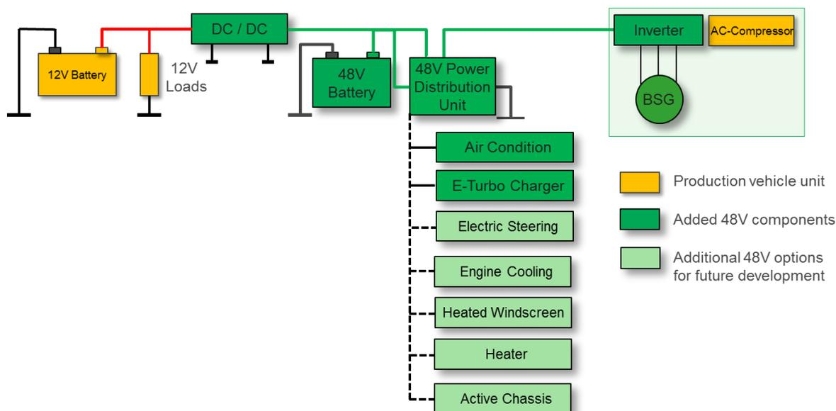
Figure 3.7 48V Demonstration Vehicle System Mechanization Drawing (Delphi Automotive®)
