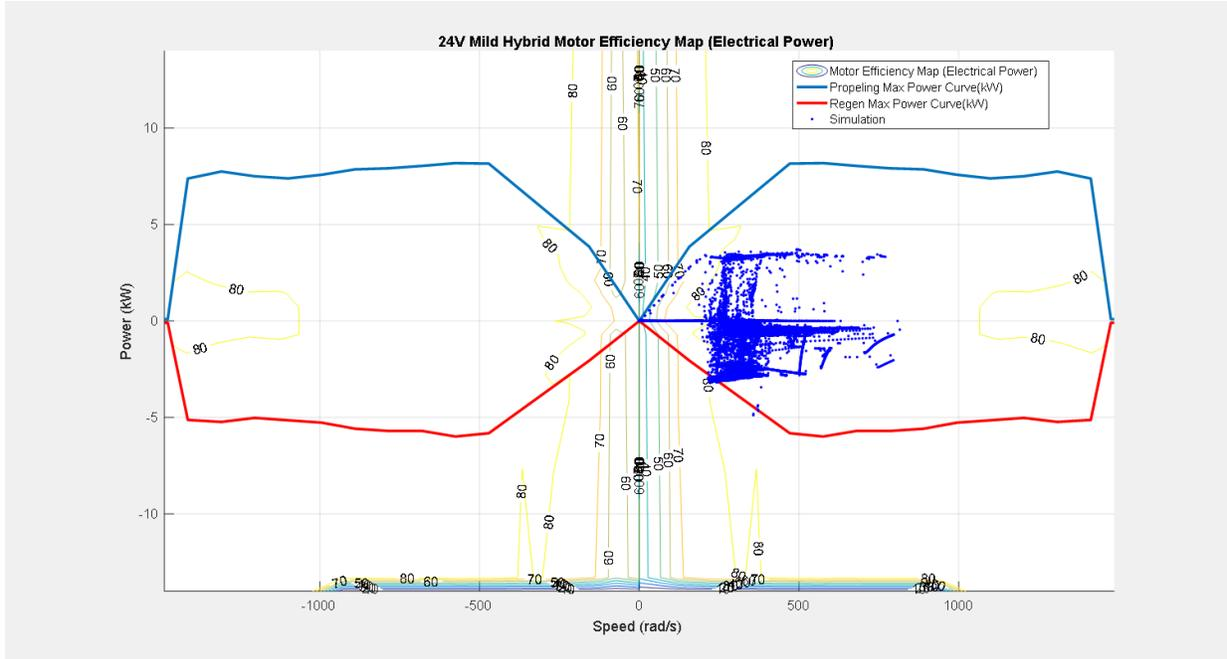
Figure 4.9 24V Mild Hybrid Motor Efficiency Map (Simulated)
