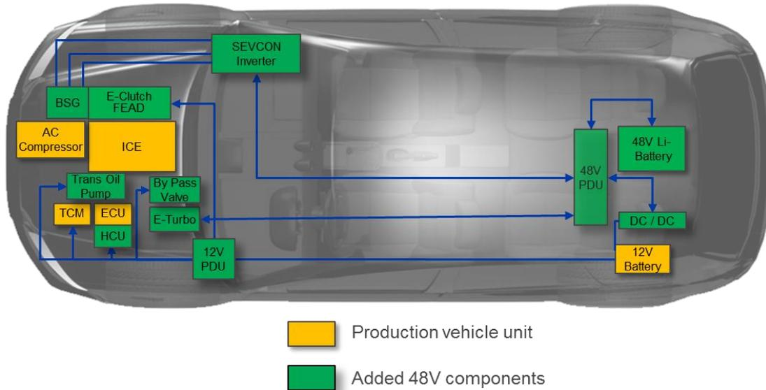
Figure 3.8 48V Demonstration Vehicle Devices Layout (designed by Delphi Automotive®)
