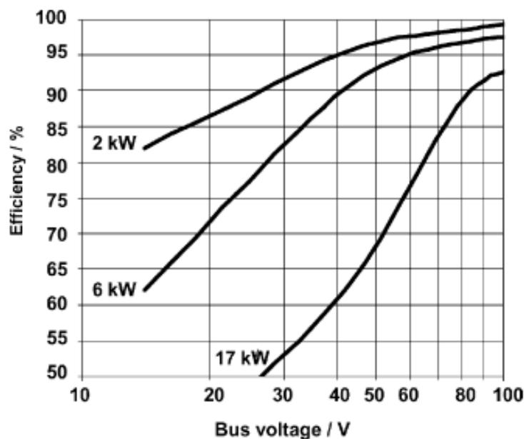
Figure 2.4 Vehicle Bus Voltage versus System Efficiency (1994) Retrieved from <http://auto.mit.edu/cosortium>
