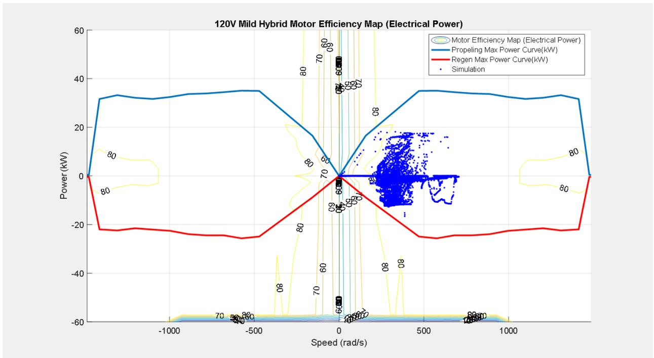
Figure 4.21 120V Mild Hybrid Motor Efficiency Map (Simulated)
