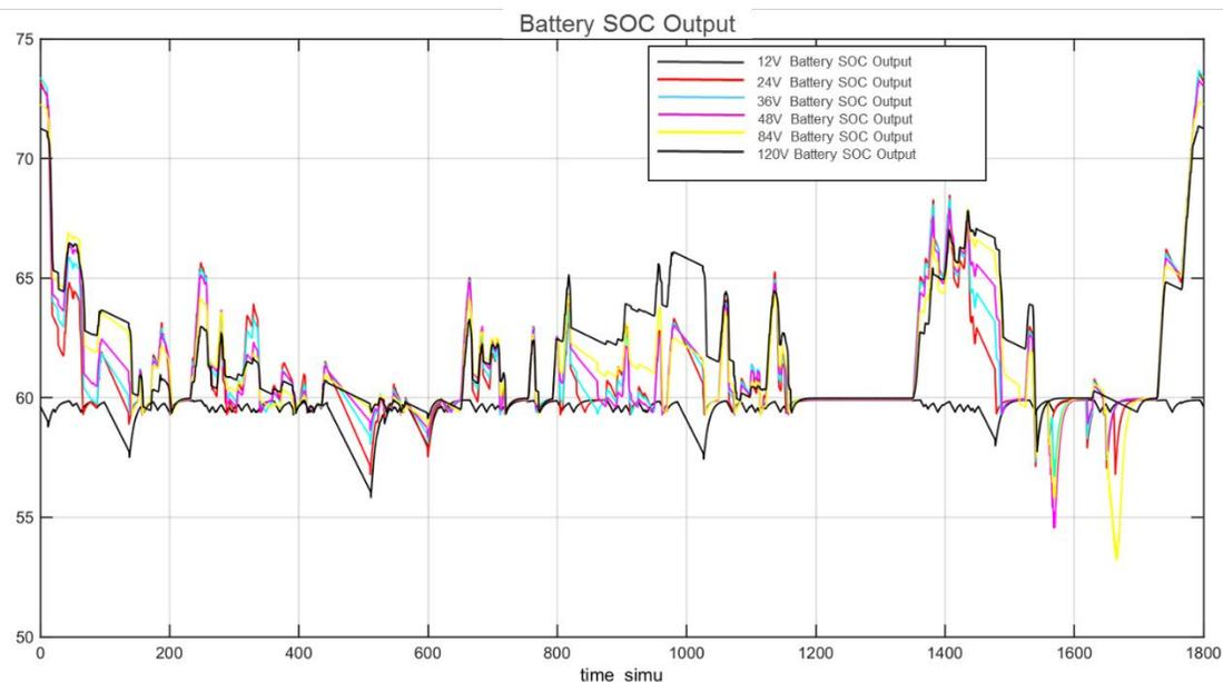
Figure 4.4 Battery SOC over Drive cycle (Simulated)
