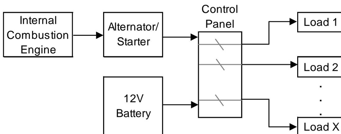
Figure 2.1 Conventional Point to Point Vehicle Electrical System (Denton, 2004)
