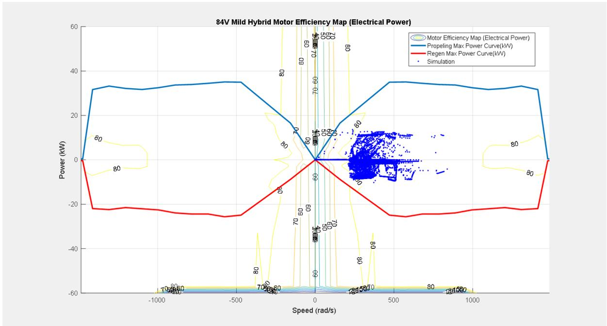
Figure 4.18 84V Mild Hybrid Motor Efficiency Map (Simulated)
