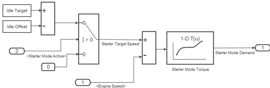
Figure 3.10 Matlab® Simulink® Based Starter Torque Logic
