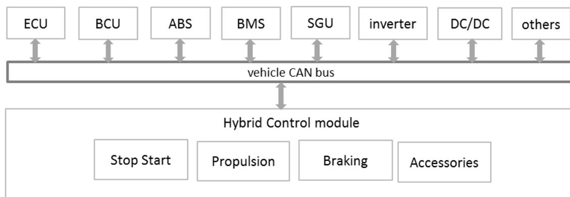
Figure 3.4 Hybrid Control Interface
