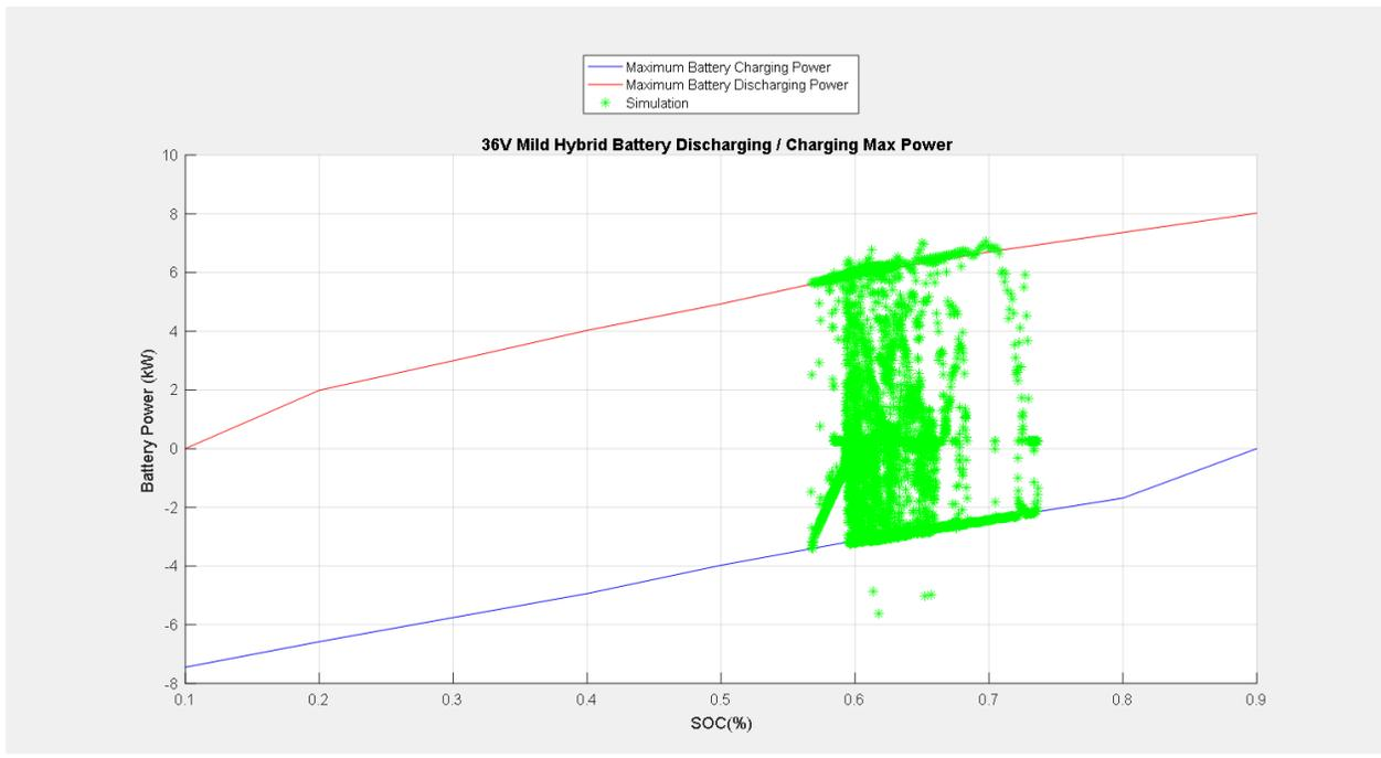
Figure 4.11 36V Battery Discharging / Charging Max Power (Simulated)
