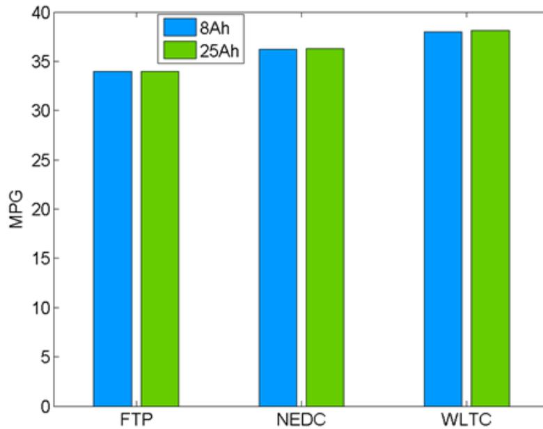
Figure 3.17 Fuel Economy Comparison of 8Ah and 25Ah Batteries (Simulation Results)
