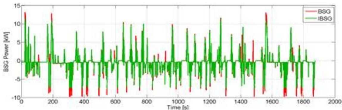
Figure 3.21 Electric Machine Power Output over FTP Drive Cycle (Simulated)
