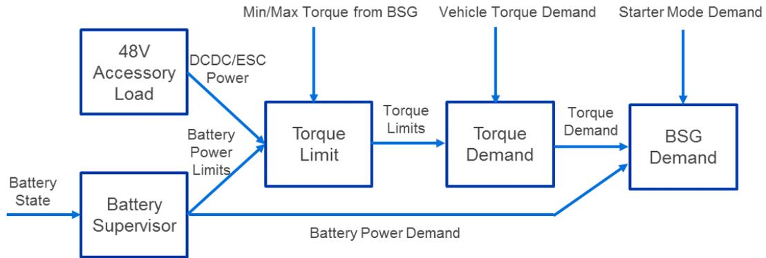
Figure 3.9 Belt Starter Generator Torque Demand Logic
