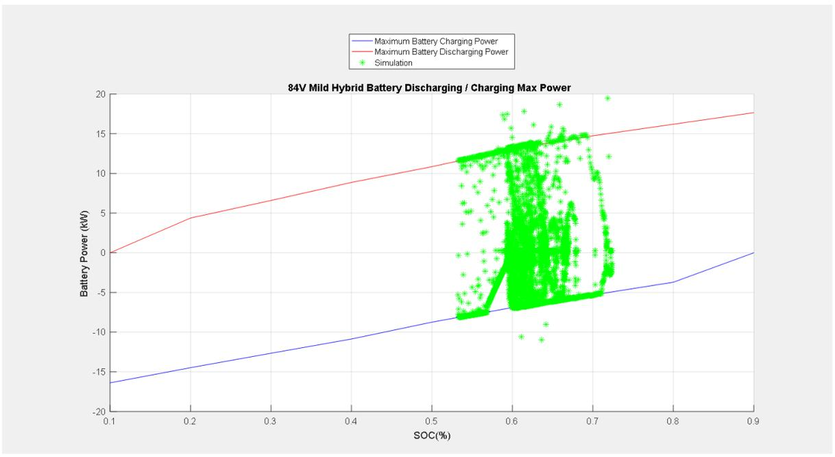
Figure 4.17 84V Battery Discharging / Charging Max Power (Simulated)
