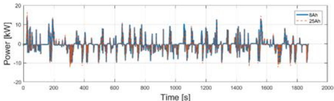
Figure 3.19 BSG Power Profiles over FTP Drive Cycle (Simulated)
