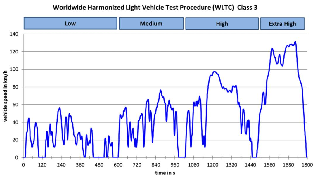
Figure 3.3 Worldwide Harmonized Light Vehicle Test Procedure (UNECE Global technical regulation No 15, 2014)
