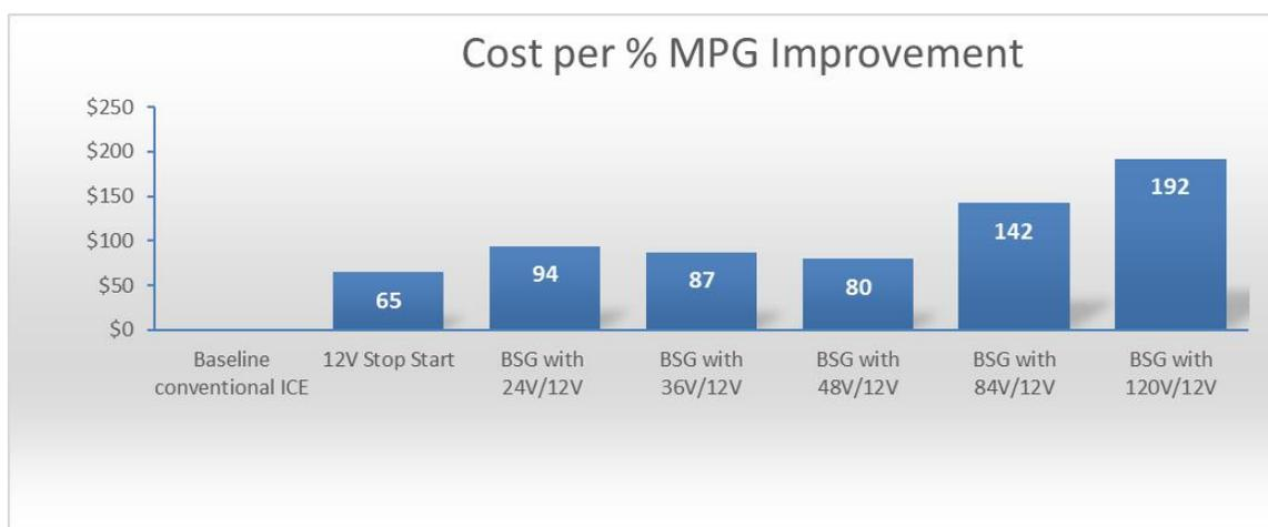
Figure 4.23 System Cost per % MPG Improvement
