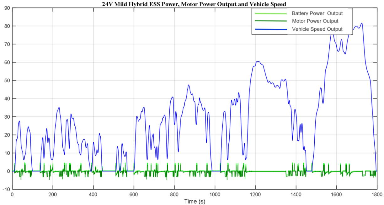
Figure 4.7 24V Battery and Motor Electric Power Output vs. Vehicle Speed (Simulated)
