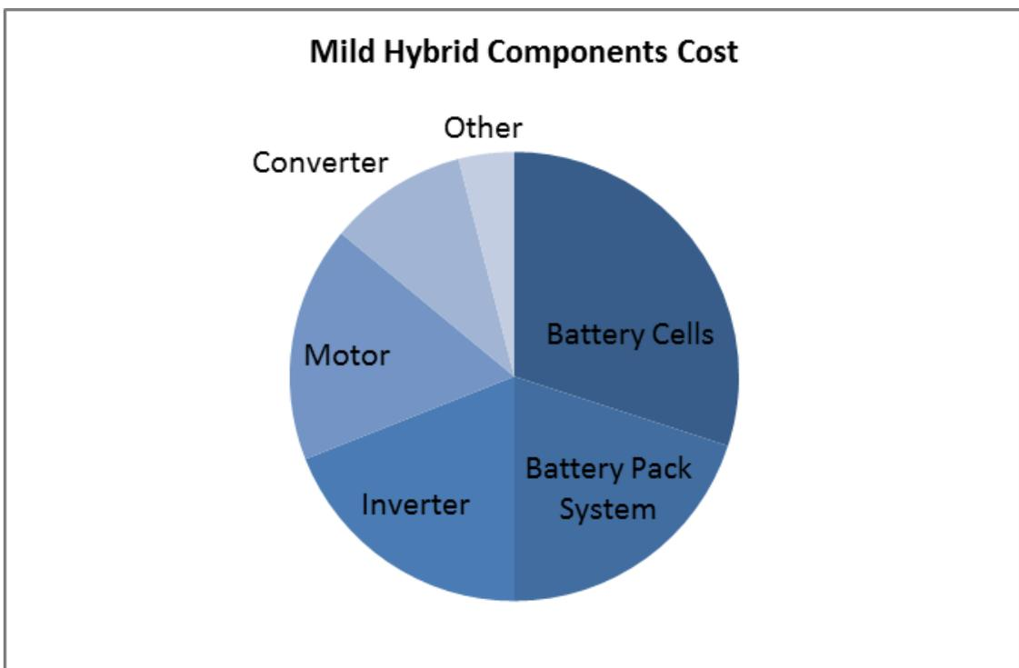
Figure 3.28 Mild Hybrid Component Cost (Delphi Automotive®)
