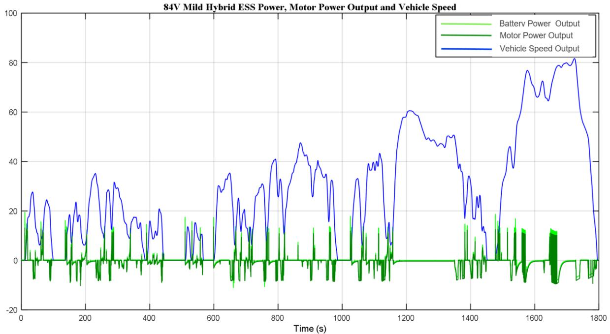
Figure 4.16 84V Mild Hybrid Battery and Motor Electric Power Output vs. Vehicle Speed (Simulated)
