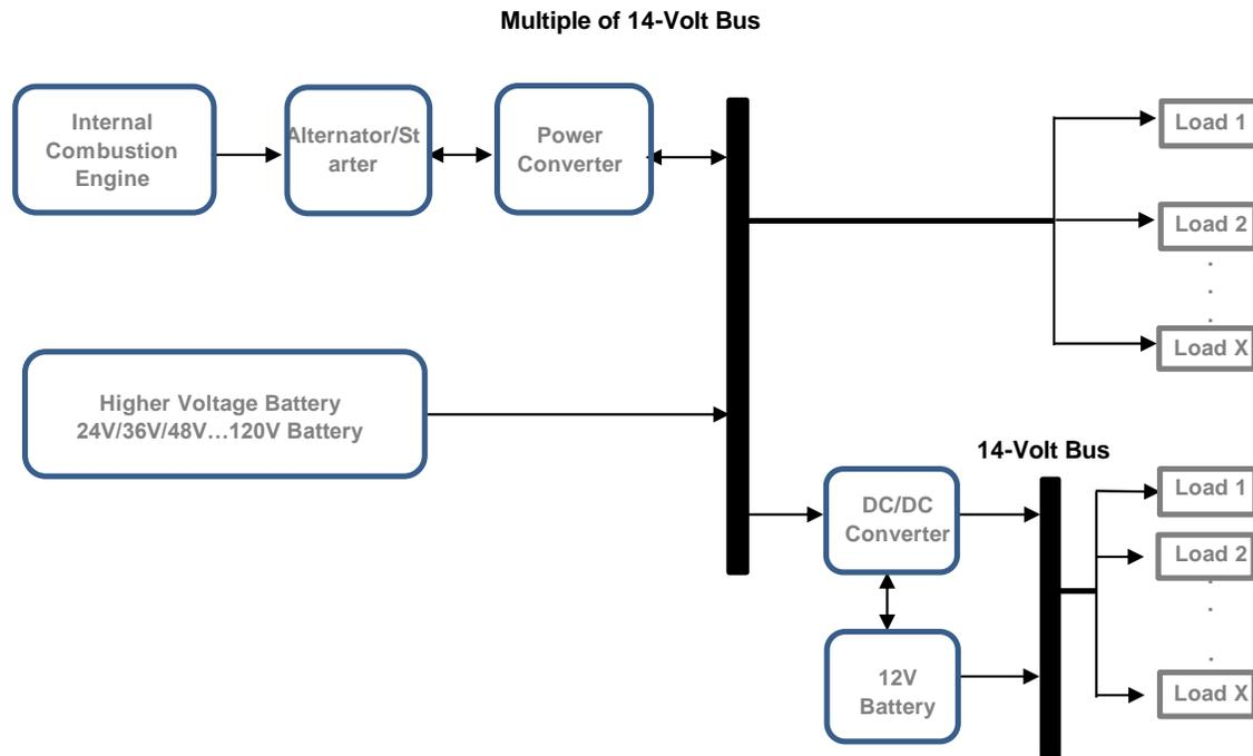
Figure 2.7 Dual Voltage Vehicle Electrical Architecture
