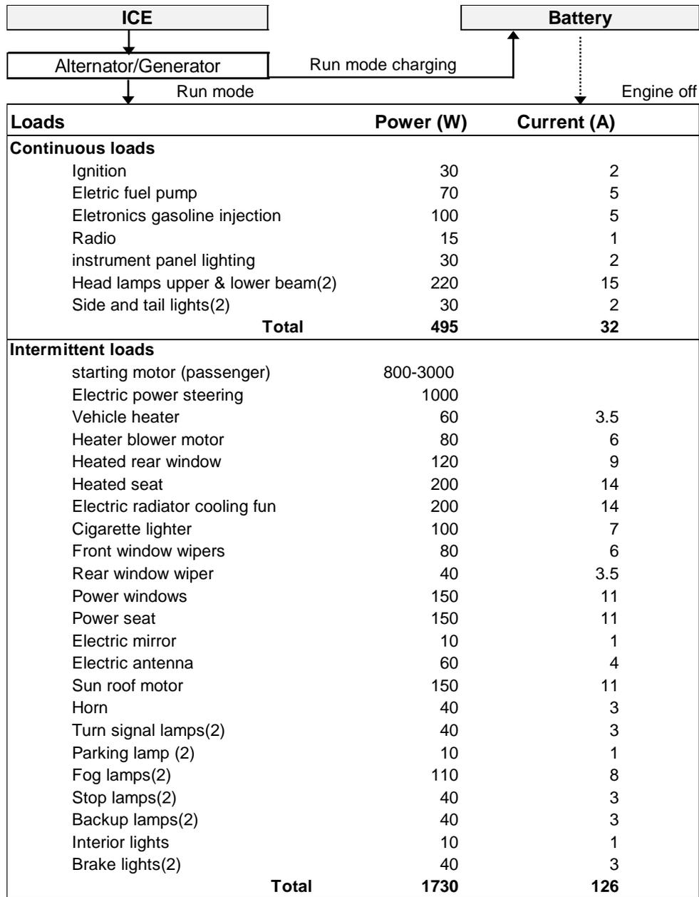
Figure 2.2 Vehicle Electrical Loads (Kassakian, 1996, Brost, 2001)
