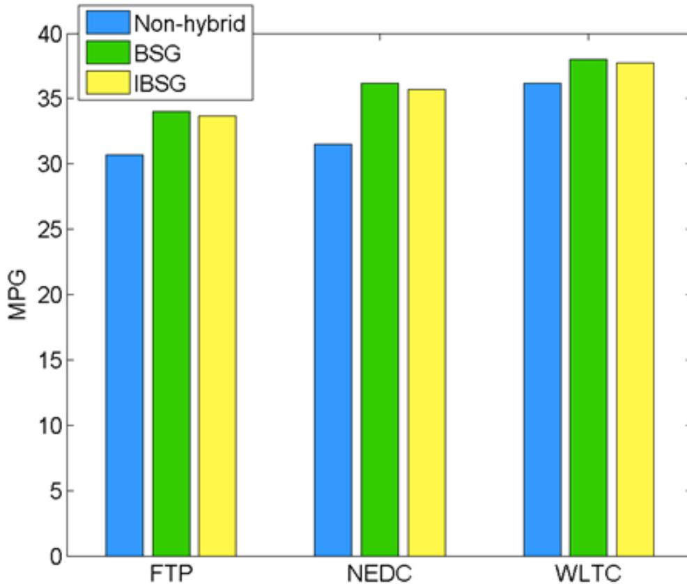
Figure 3.20 Electric Machine Fuel Economy Improvement Comparison (Simulation Results)
