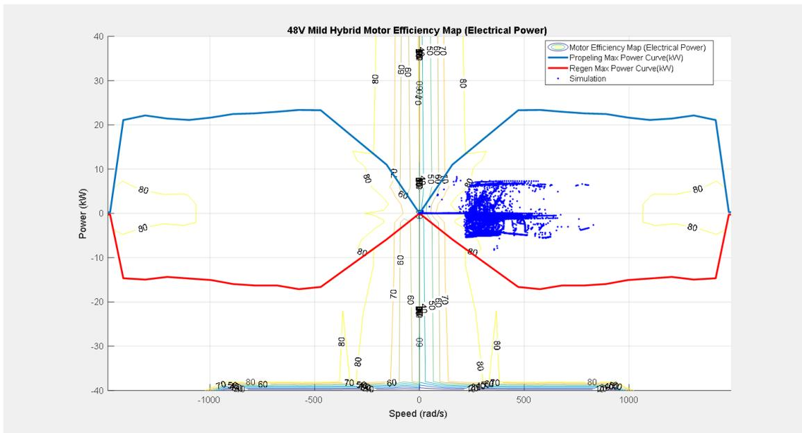
Figure 4.15 48V Mild Hybrid Motor Efficiency Map (Simulated)
