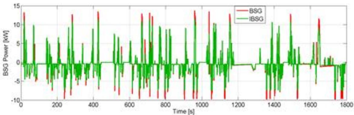
Figure 3.23 Electric Machine Power Output over WLTC Drive Cycle (Simulated)
