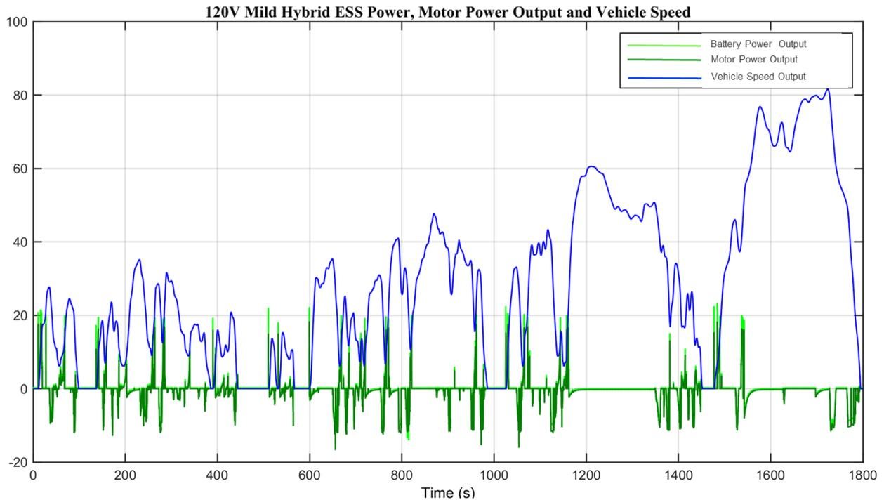
Figure 4.19 120V Mild Hybrid Battery and Motor Electric Power Output vs. Vehicle Speed (Simulated)
