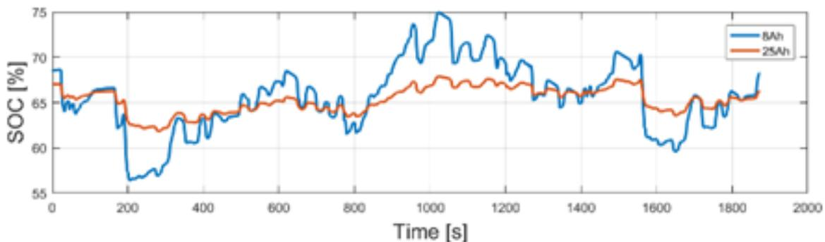
Figure 3.18 Battery SOC over FTP Drive Cycle (Simulated)
