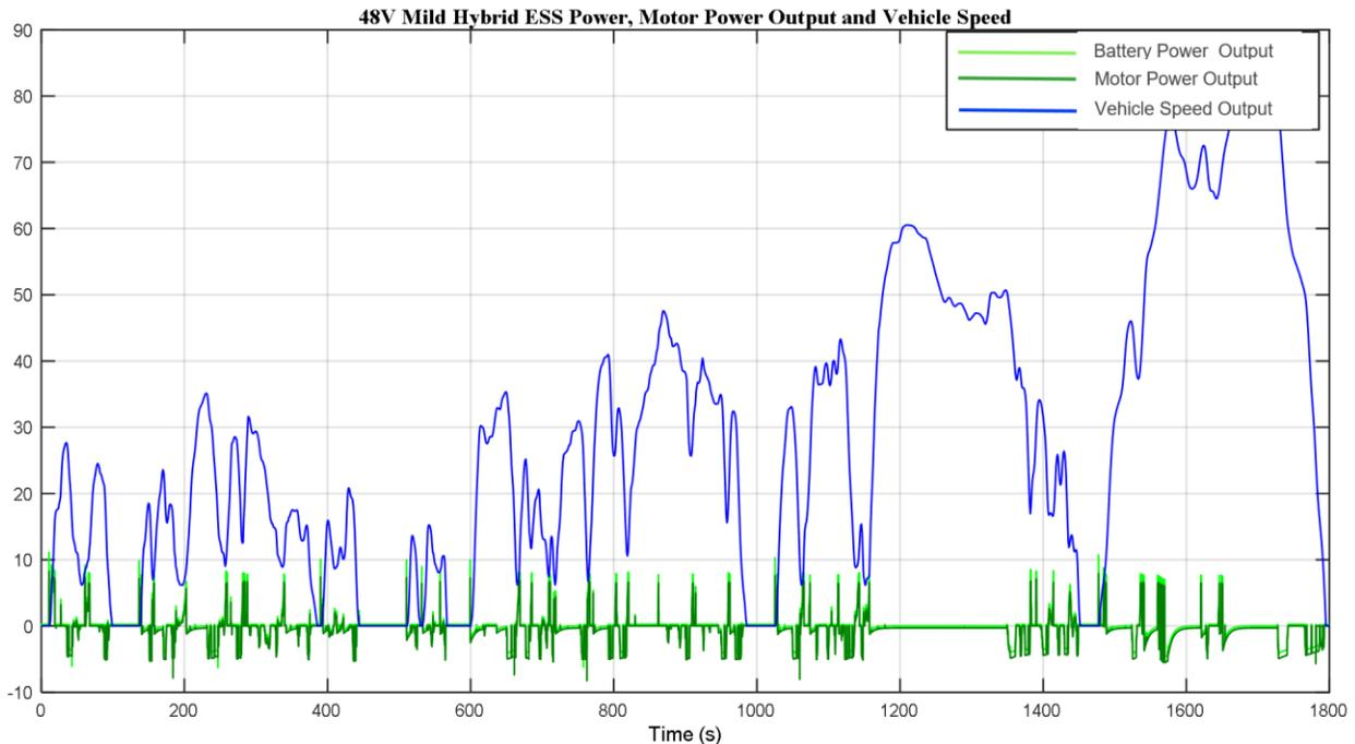
Figure 4.13 48V Mild Hybrid Battery and Motor Electric Power Output vs. Vehicle Speed (Simulated)
