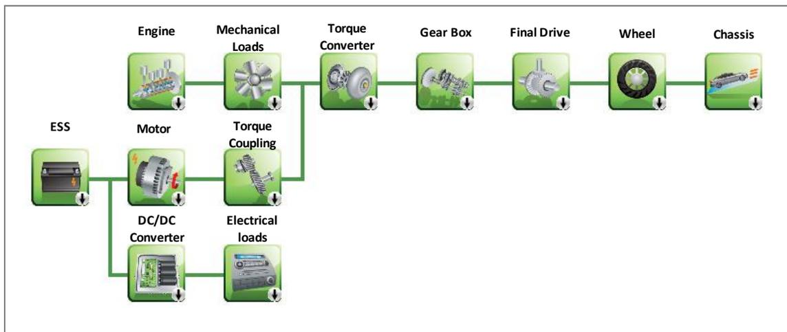
Figure 3.2 Autonomie Parallel BSG Vehicle Propulsion Architecture
