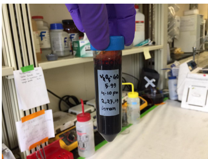
Fig. 3.3. Dark red V_2O_5/GO after 2 weeks of aging bringing about the formation of completed network of V_2O_5 hydrogel.
