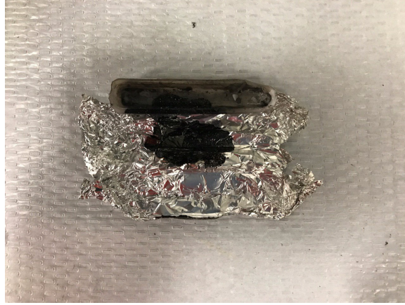
Fig. 2.10. Annealed electro-spun V_2O_5/GO + PVA (0.25g) at 400 °C .
