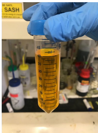
Fig. 2.2. Yellowish HVO_3 solution, which brings about V_2O_5 formation.
