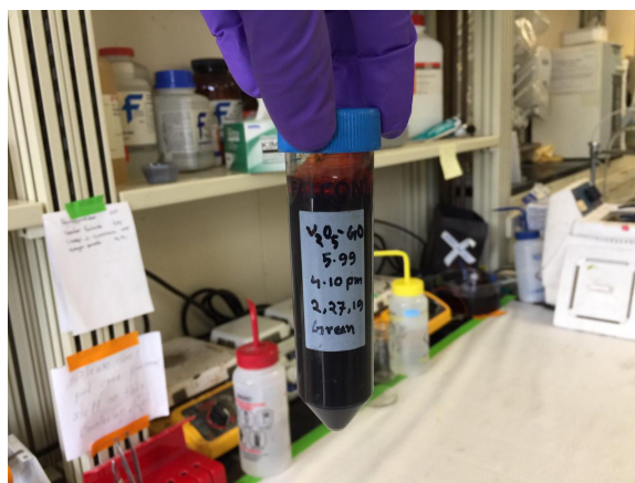
Fig. 2.4. Dark red 2 weeks old V_2O_5/GO : signifying the completion of the formation of a 3D network of V_2O_5 hydrogel.
