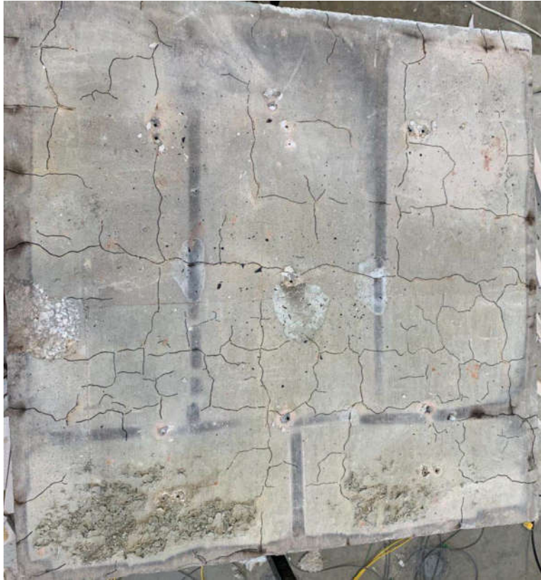
Figure 4-12. Map of Cracks for D-80-1600
