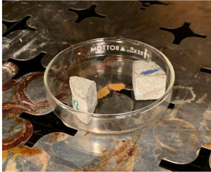
Figure 3-20. Oven Dry Process of SEM Specimen Preparation
