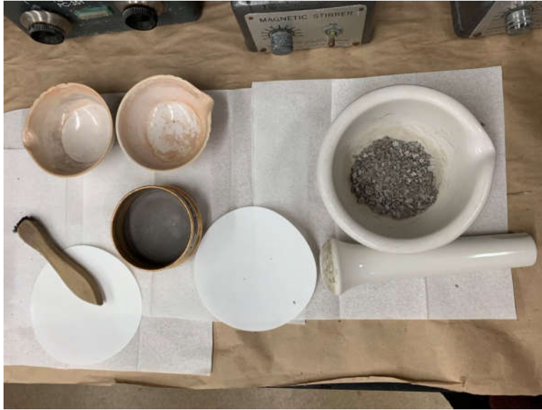
Figure 3-27. Grinding Process for DSC Sample Preparation
