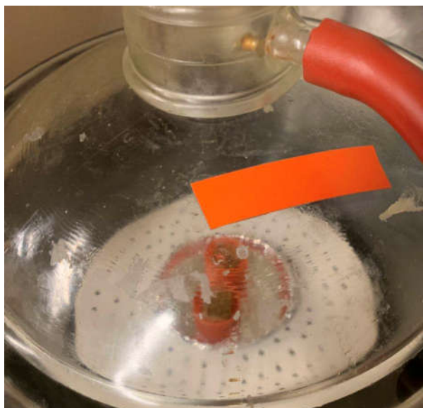
Figure 3-22. Vacuum Process for SEM Specimen Preparation
