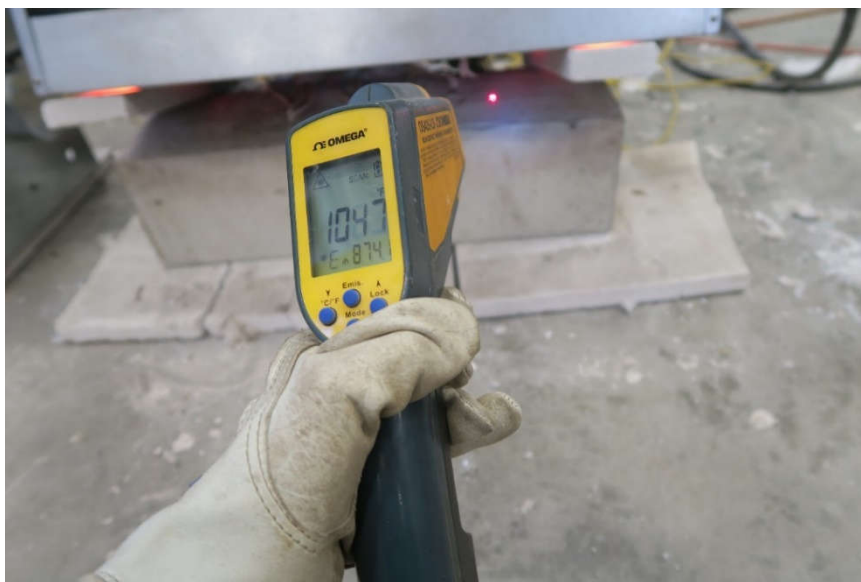
Figure 3-11. Surface Temperature Verification by Handheld Temperature Indicator
