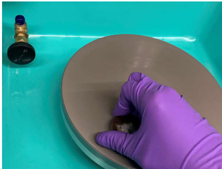
Figure 3-25. Lapping Process for SEM Specimen Preparation
