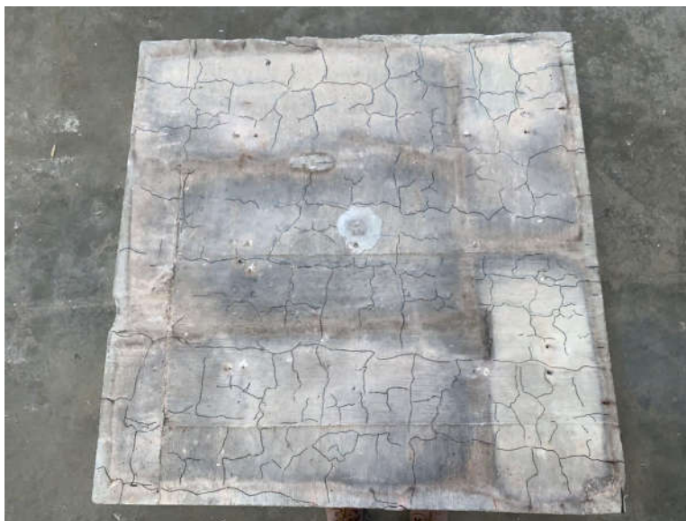
Figure 4-5. Map of Cracks for D-40-1100
