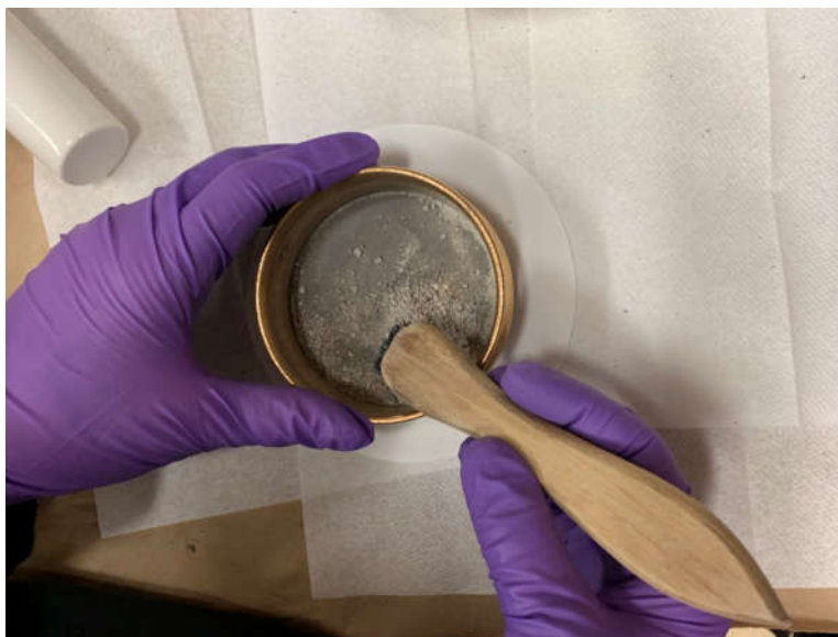
Figure 3-28. Sieving Process for DSC Sample Preparation
