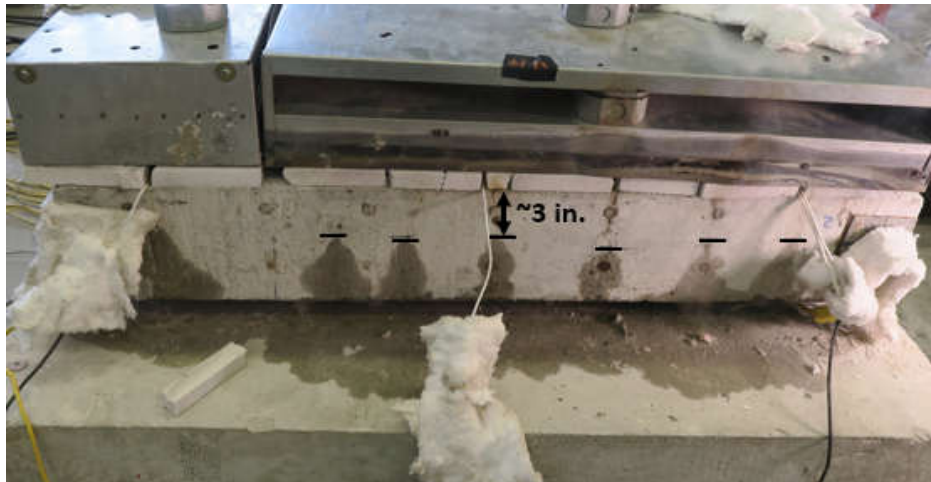
Figure 4-10. Locations of Sweeping Moisture at One Side of D-80-1600
