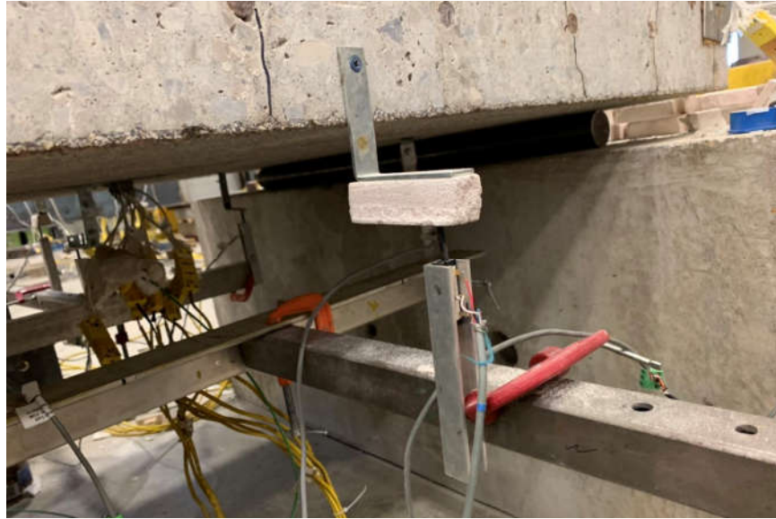
Figure 3-17. Example of Protection of Displacement Transducers
