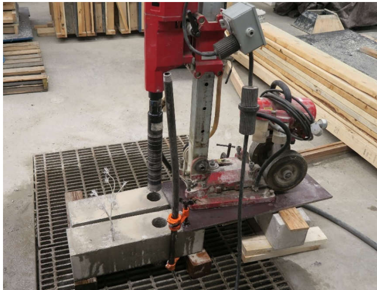
Figure 3-7. Drilling Process after the Curing Process of Small Beam
