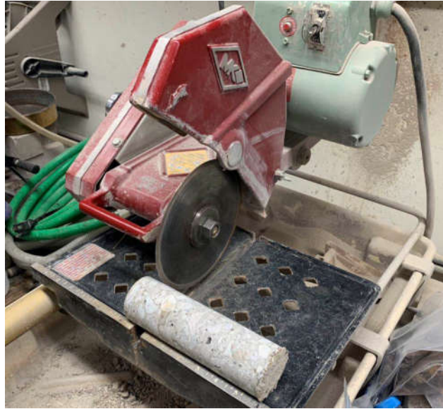
Figure 3-19. Cutting Process of SEM Specimen Preparation
