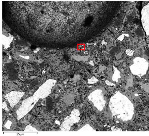
Figure 4-30. EDS Identification of CH of Unheated Sample at Exposed Surface
