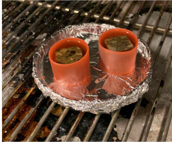
Figure 3-23. Oven Drying Process for SEM Specimen Preparation
