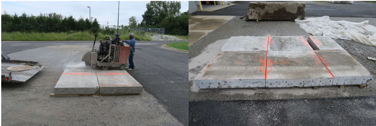
Figure 3-4. Deck Specimens Cut from the Original Deck Sections
