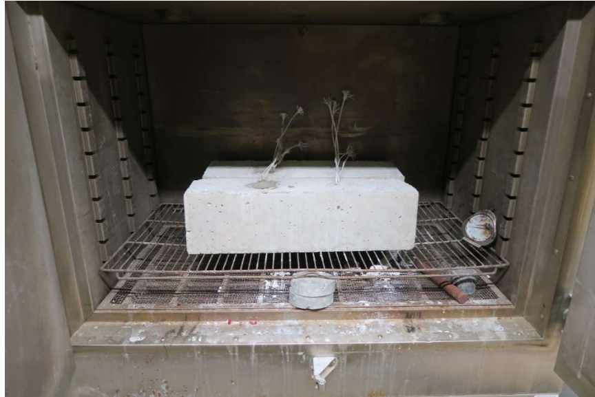
Figure 3-9. Oven-Dry Process for Small Beam
