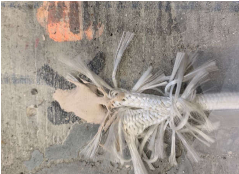
Figure 3-14. Surface Thermocouple Covered by High Temperature Cement
