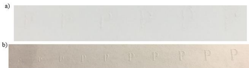
Figure 34: Screen printing of radiative cooling paint pattern onto a) barium sulfate coated art paper and b) commercial printer paper.
