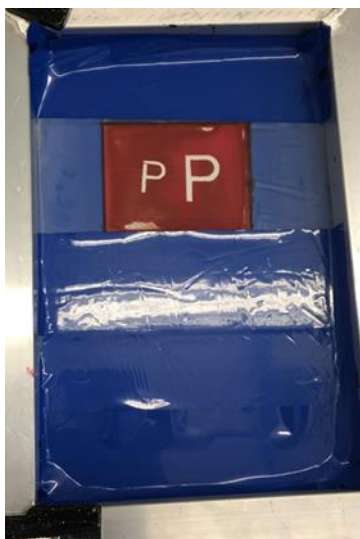
Figure 31: Screen printing setup for processing of radiative cooling paint samples.
