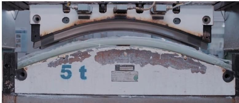
Figure 1.19 - Compression molding press [21]
