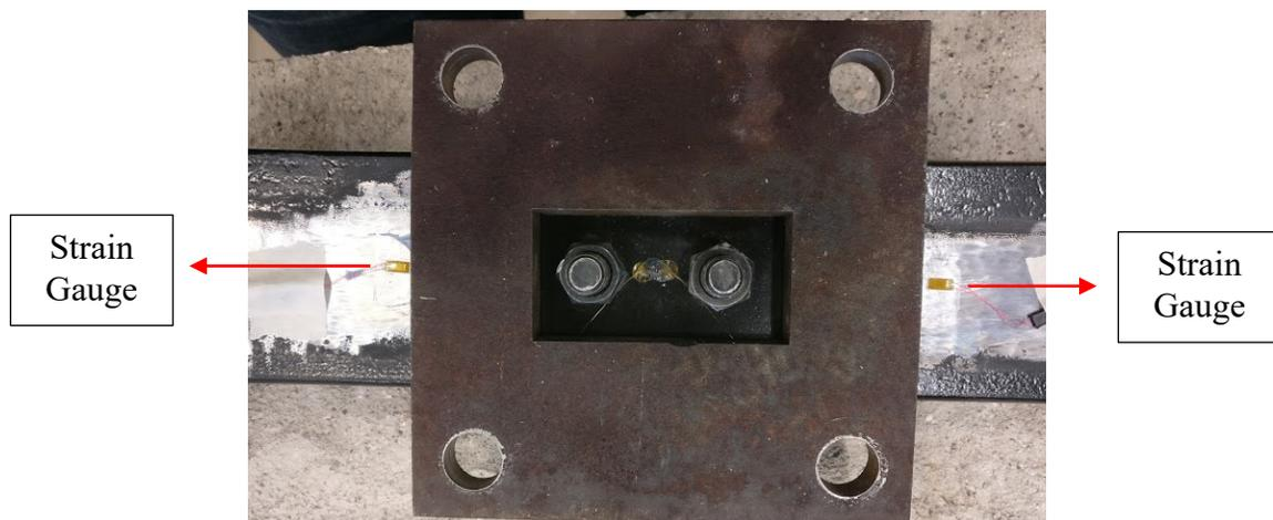
Figure 4.19 - Location of strain gauges on the main leaf
