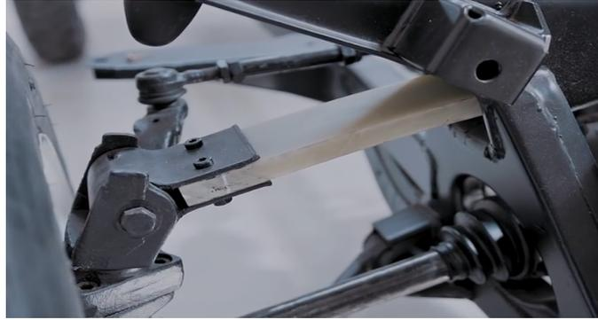
Figure 1.20 - Attachment of leaf spring using metal fasteners [21]
