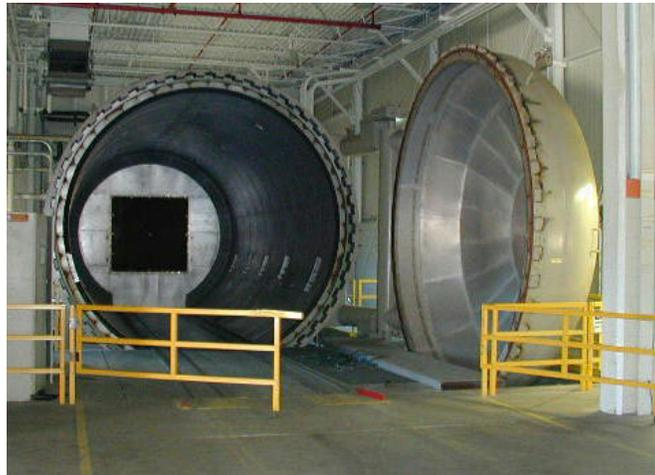
Figure 1.3 - Large size autoclave
