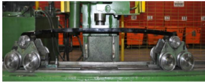
Figure 1.12 - Fatigue and stiffness testing jig for composite leaf spring [12]
