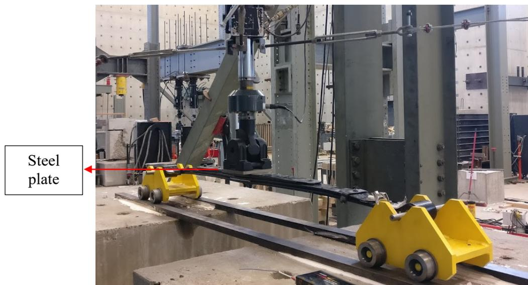
Figure 4.8 - Deflection of spring in unclamped condition
