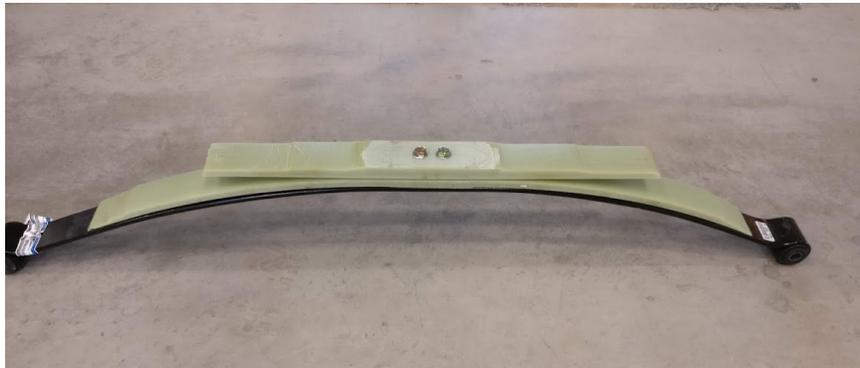
Figure 3.15 - Leaf spring assembly after replacing cracked third leaf
