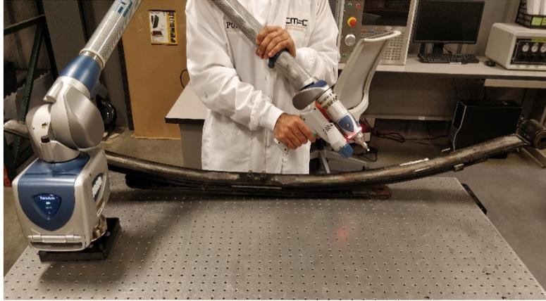
Figure 3.6 – Laser scanning the geometry of leaf spring
