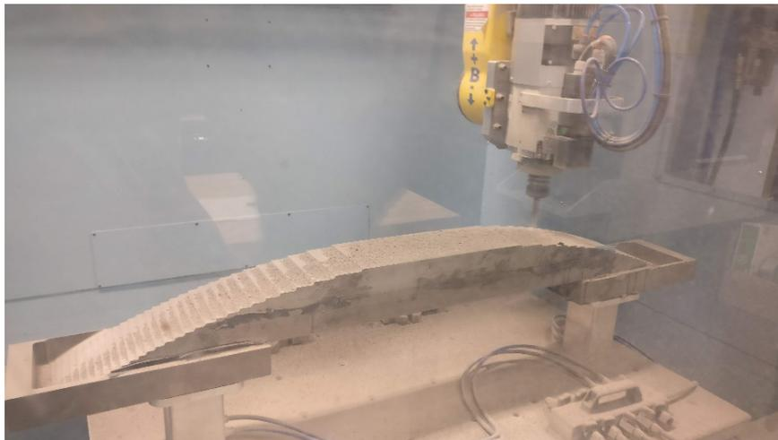
Figure 3.7 - Machining of the tooling board
