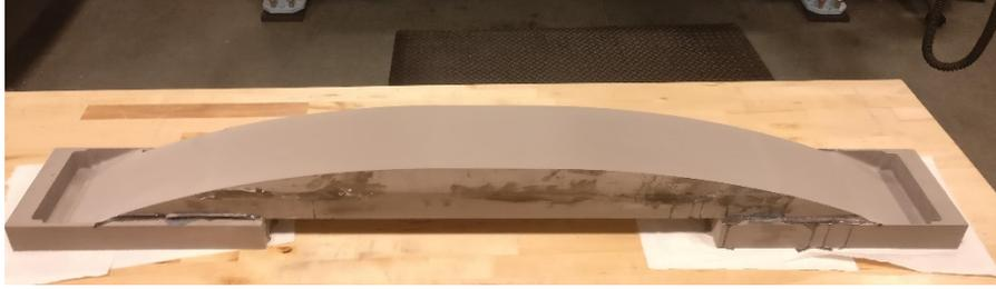
Figure 3.8 - Machined tool for layup
