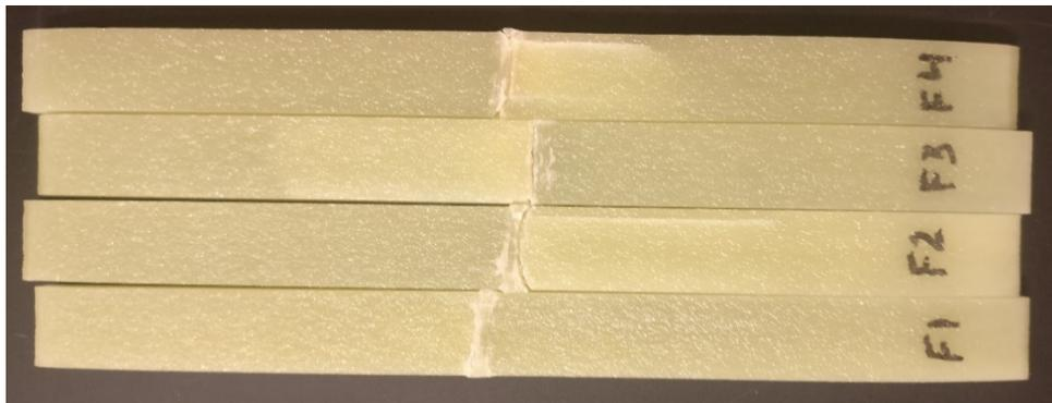
Figure 4.29 - Top view for failure of specimens in cyclic loading, Aspect Ratio 10
