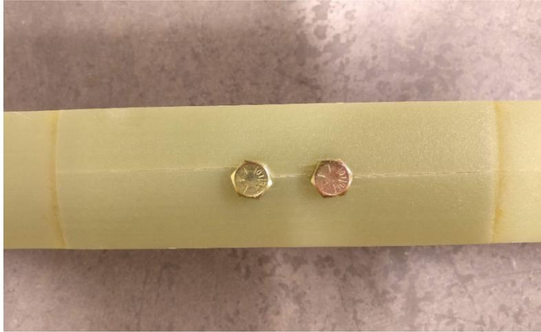
Figure 3.11 - Cracking of composite 3<sup>rd</sup> leaf
