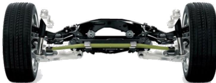
Figure 1.17 - Transverse composite leaf spring for Volvo XC90 [20]
