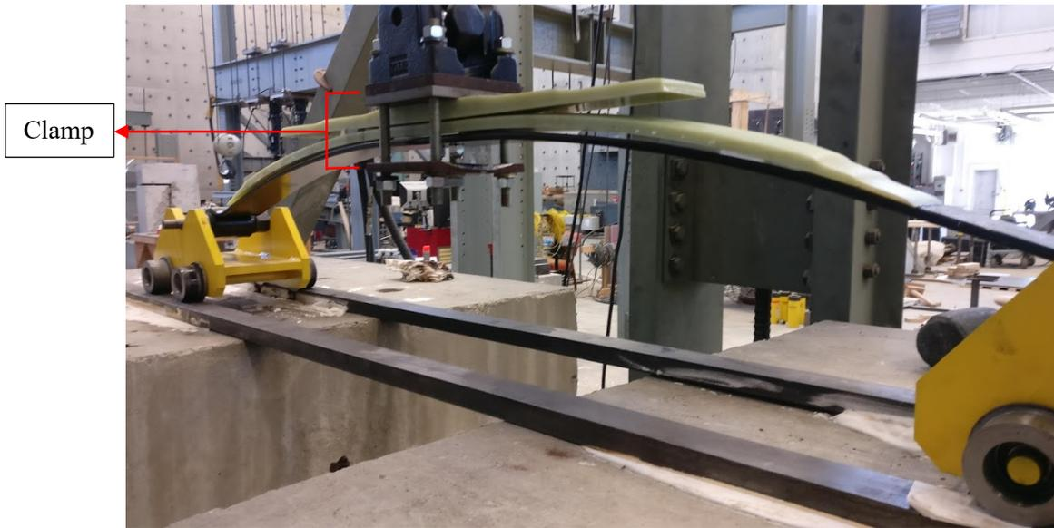
Figure 4.9 - Loading of composite spring in unclamped and clamped condition
