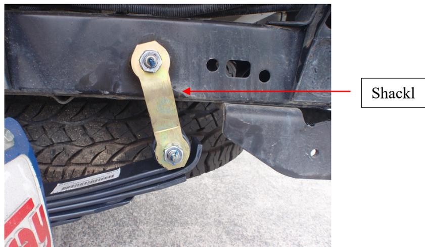
Figure 1.6 - Shackle attachment at one end of the leaf spring [7]
