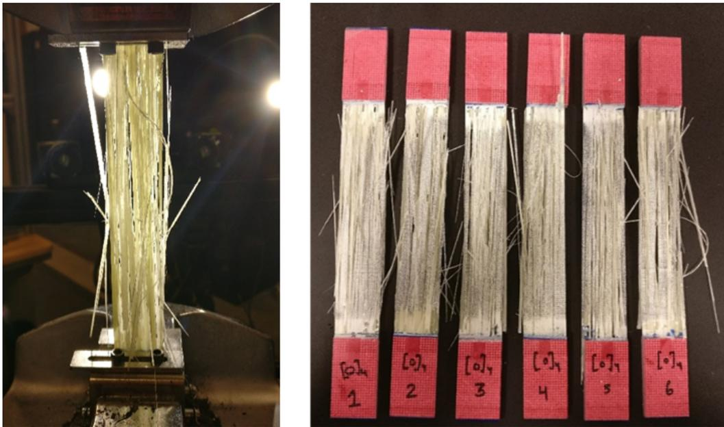
Figure 4.4 - Failure of specimens from loading in 1 direction
