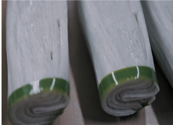
Figure 1.18 - Use of rolled prepregs for leaf spring compression molding [21]
