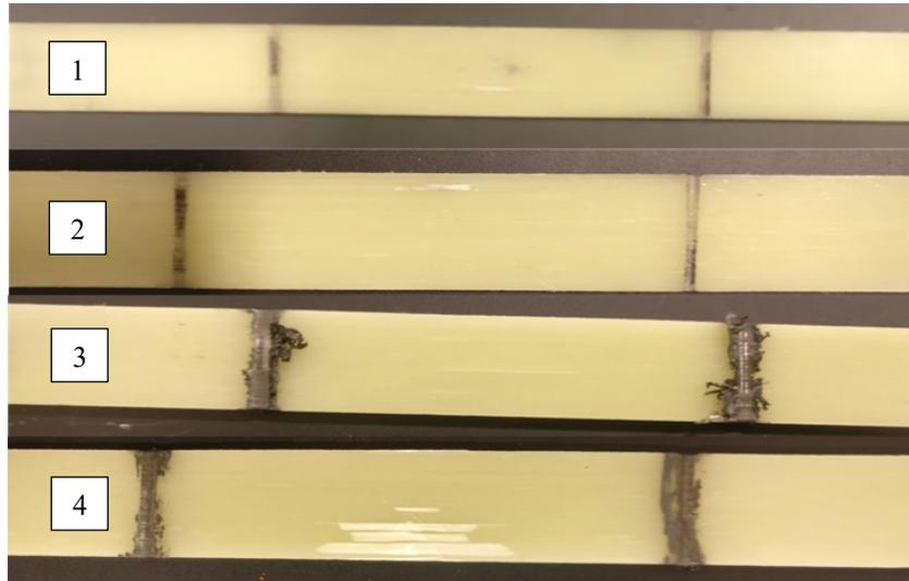
Figure 4.37 - Bottom view of specimens after cyclic loading, Aspect Ratio 30
