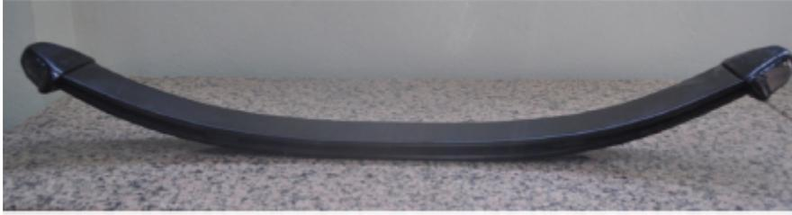
Figure 1.11 – Steel prototype spring [12]
