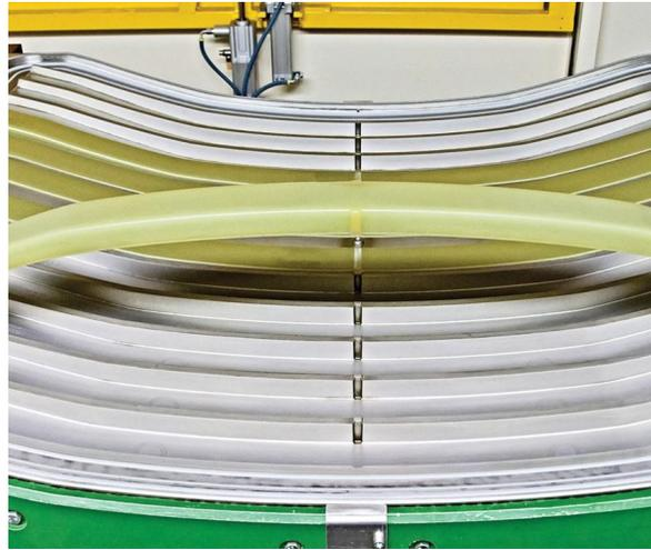
Figure 1.16 - Multicavity tool for resin transfer molding of leaf springs [19]
