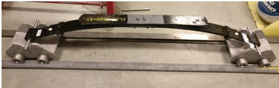
Figure 3.4 - Fixture and leaf spring assembly
