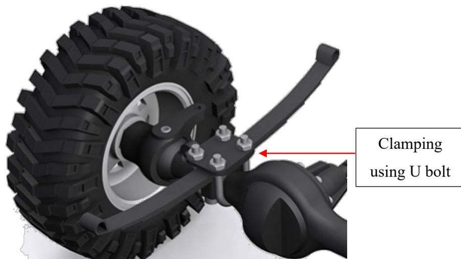
Figure 2.3 - U bolt assembly used for clamping leaf spring to axle
