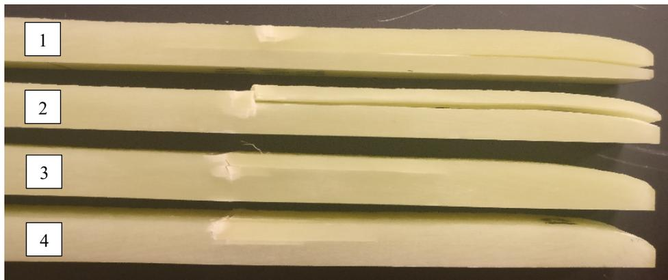
Figure 4.28 - Side view for failure of specimens in cyclic loading, Aspect Ratio 10
