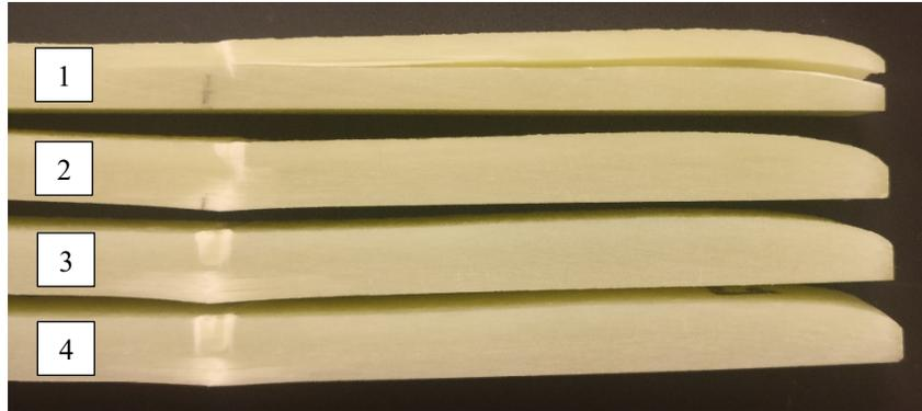
Figure 4.22 - Side view of samples failed quasi-statically, Aspect Ratio 10
