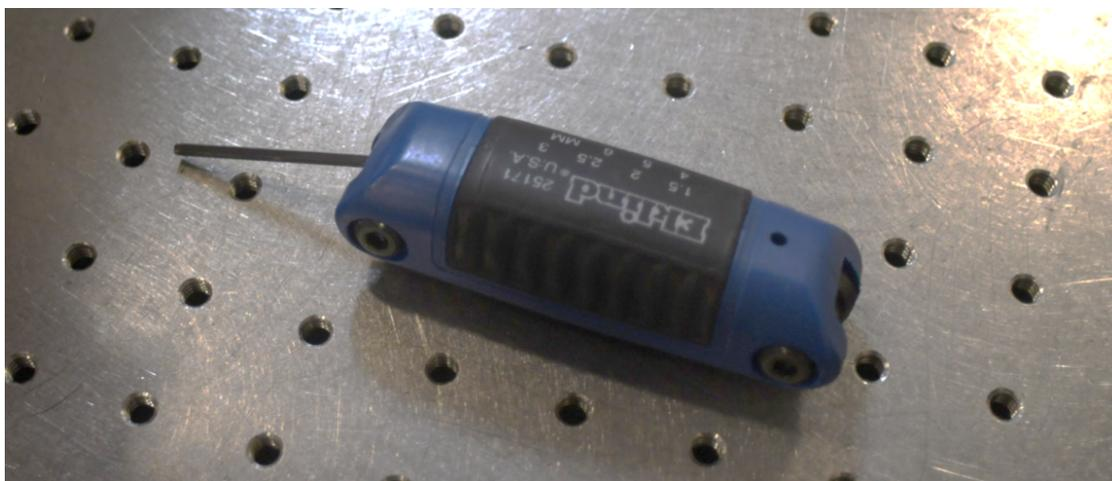
Figure 3.8: This is the metric Allen Key, for tightening the two screws on the Thor Labs dove-tail mounting plate. It is your friend. **Do not lose it.**
