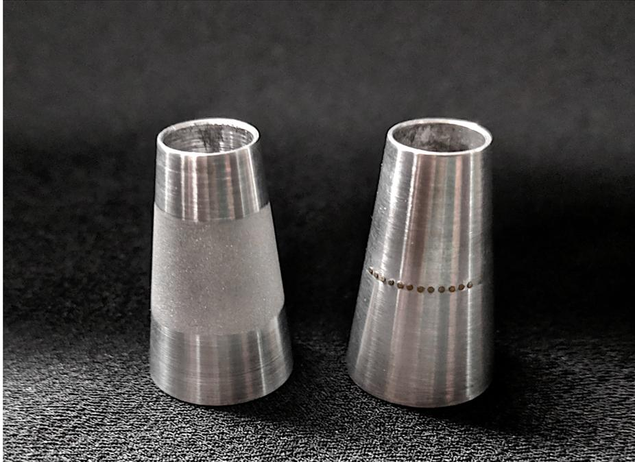
**Figure 2.7.** A photograph of the two roughness inserts used in the present experiments: Sandblasted (left) and RIM (right).
