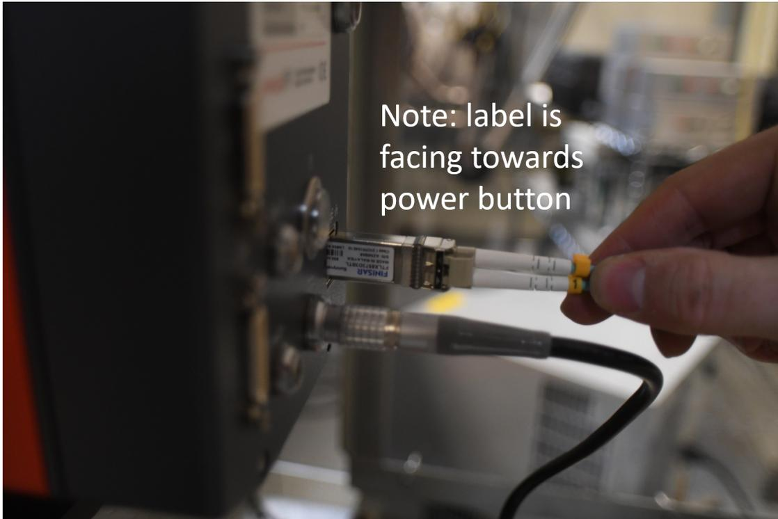
Figure 3.11: The proper orientation for inserting the fiber optic cable into the camera. Note that the white label on the GigE adapter is oriented toward the power button (toward the user as well).
