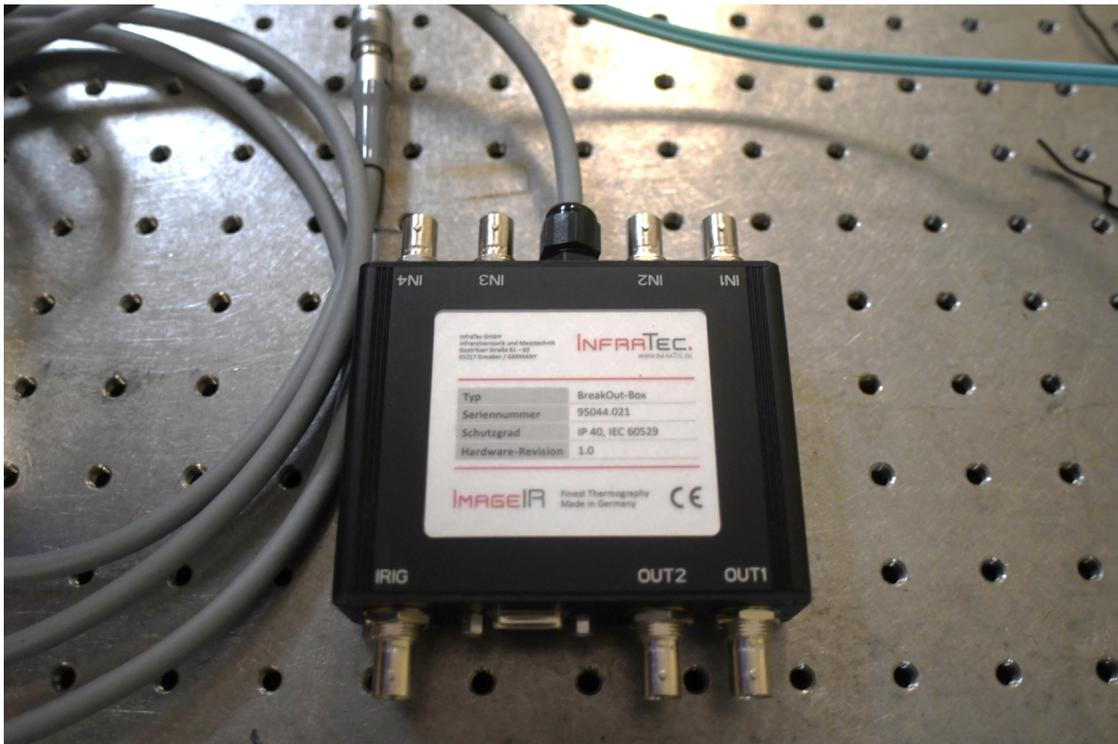
Figure 3.12: The trigger input box and cable.
