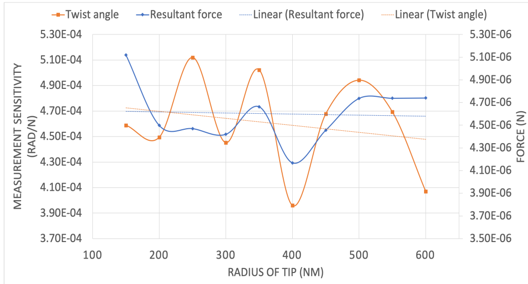
Figure 4.23 The twist angle and force with varied radius of tip design A on cantilever A with hard sample
