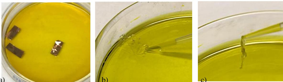
*Figure 4.2 Single PMMA spin coat on graphene before and after Cu etch (a) PMMA on graphene on Cu when first put in Cu etchant, (b) Single PMMA coat on graphene after Cu etch, (c) Handling film resulted in it crumpling up on itself making incapable of transfer*
