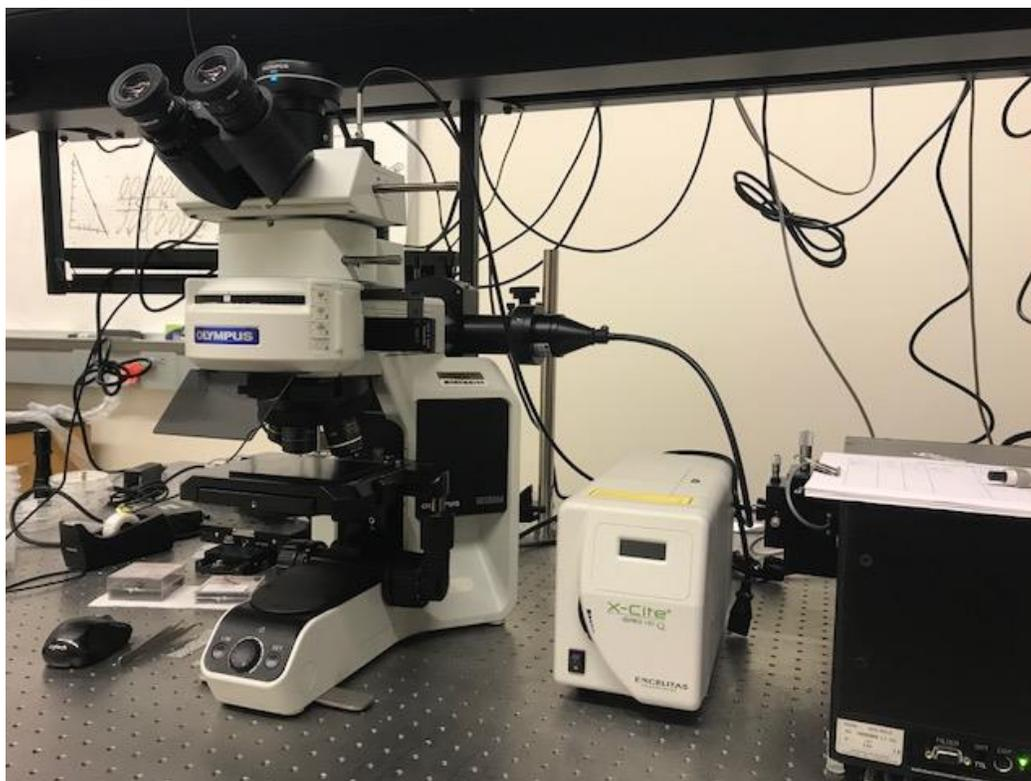
*Figure 3.5 Olympus BX53M System Microscope, X-Cite Series 120, and Spectra Pro HRS - 300*
