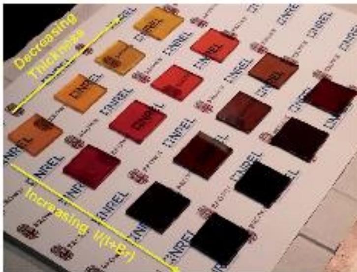
*Figure 2.2 Zhou et al. (2015) Varying perovskite spin coating speeds can control color*
