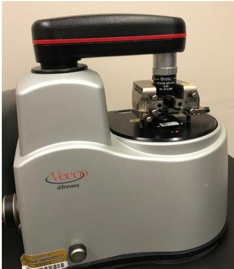
*Figure 3.2. Veeco Innova AFM Microscope Used*
