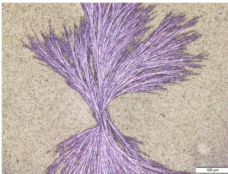
*Figure 4.41 Trial 5 first sign of degradation of sample A at 48 hours of 80% humidity exposure*
