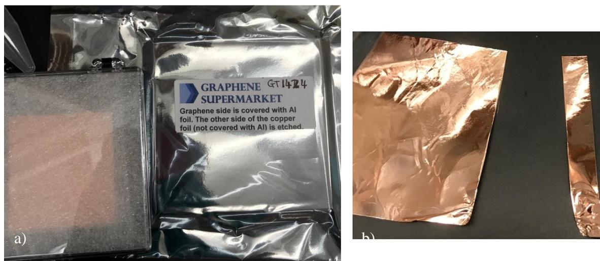
Figure 3.8 – CVD Graphene on copper foil used in Trials 4 – 6 successfully transferred to MAPBI<sub>3</sub>; (a) CVD graphene from Graphene Supermarket in original encasement, (b) CVD monolayer graphene on Cu foil (face up)
