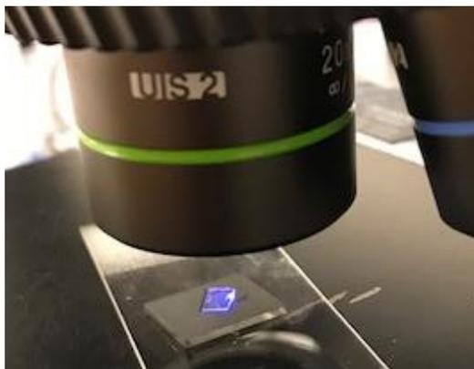
*Figure 3.9 UV Light Illuminating PET Substrate on MAPbI<sub>3</sub>*
