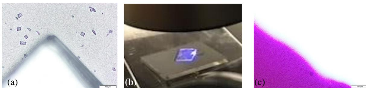
*Figure 4.1 PET/Graphene Lamination on MAPbI<sub>3</sub>, scale bars are 100 $\mu$ m (a) Brightfield image of edge of PET/Graphene on MAPbI<sub>3</sub> (b) Entire sample during PL imaging; UV light illuminates PET substrate (c) PL image at edge of PET/Graphene on MAPbI<sub>3</sub>*
