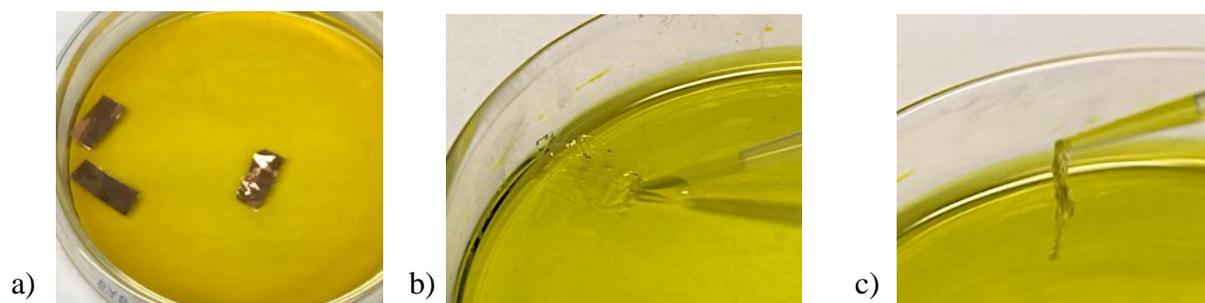
*Figure 3.11 Single PMMA spin coat on graphene before and after Cu etch (a) PMMA on graphene on Cu when first put in Cu etchant, (b) Single PMMA coat on graphene after Cu etch, (c) Handling film resulted in it crumpling up on itself making incapable of transfer*
