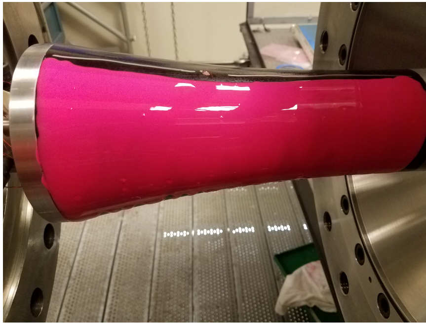
Figure 2.27. The oil applied to the suction model before a run.
