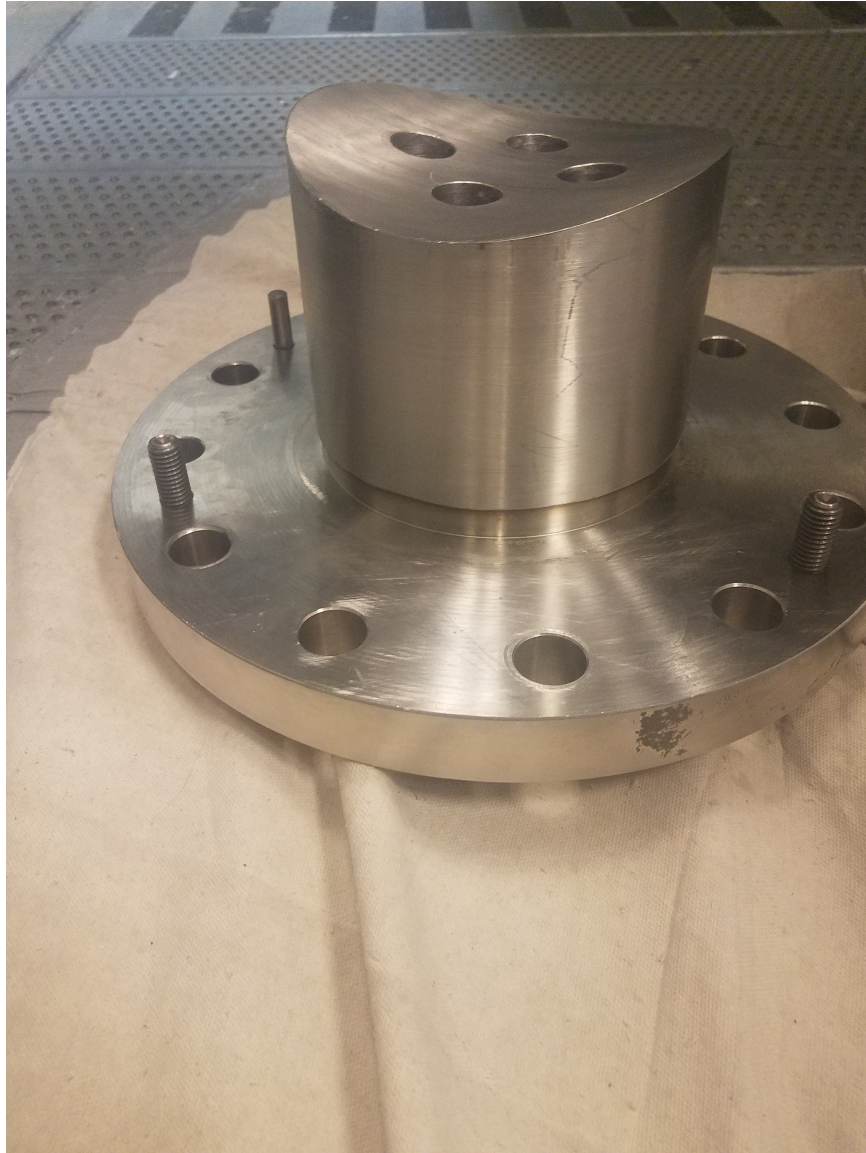
Figure E.2. 6-inch, stainless steel plug typically installed in the side of the BAM6QT just downstream of the sting support.
