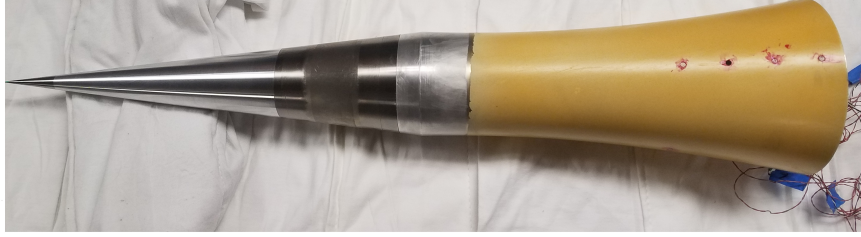
Figure 2.24. The suction model painted with temperature-sensitive paint (yellow region).
