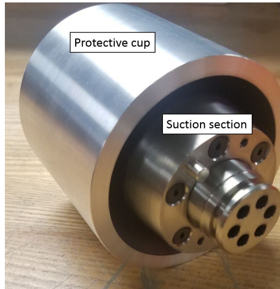
Figure 2.17. Protective shield for use in load testing the welds on the perforated skins. Installed in the cup is Suction Section 1.
