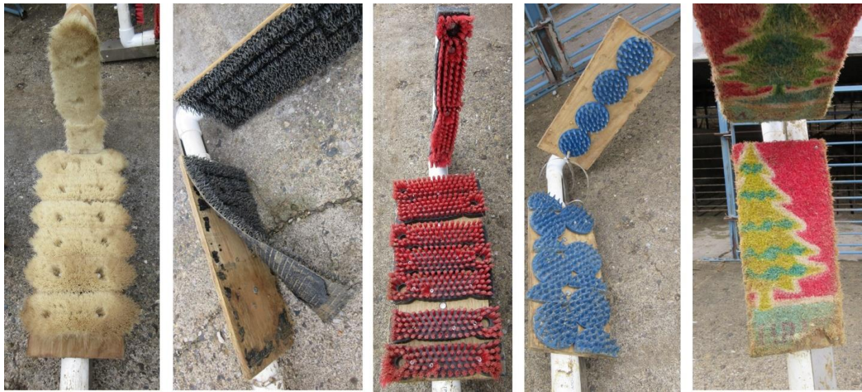
Figure 2.12. Pictures of the scratch posts after they were pulled from the pens at the end of the experiment. From left to right, post and damage done: 1) the white brushes at the bottom of the post were dirty, 2) the plastic mat was mostly unattached from the board at the bottom, 3) the red brushes had a little wear at the bottom, the bottom brush's bristles had been chewed on, 4) blue plastic combs were a little dirty, and 5) the colorful coir fiber mat was a little dirty and was missing a small chunk at the bottom.
