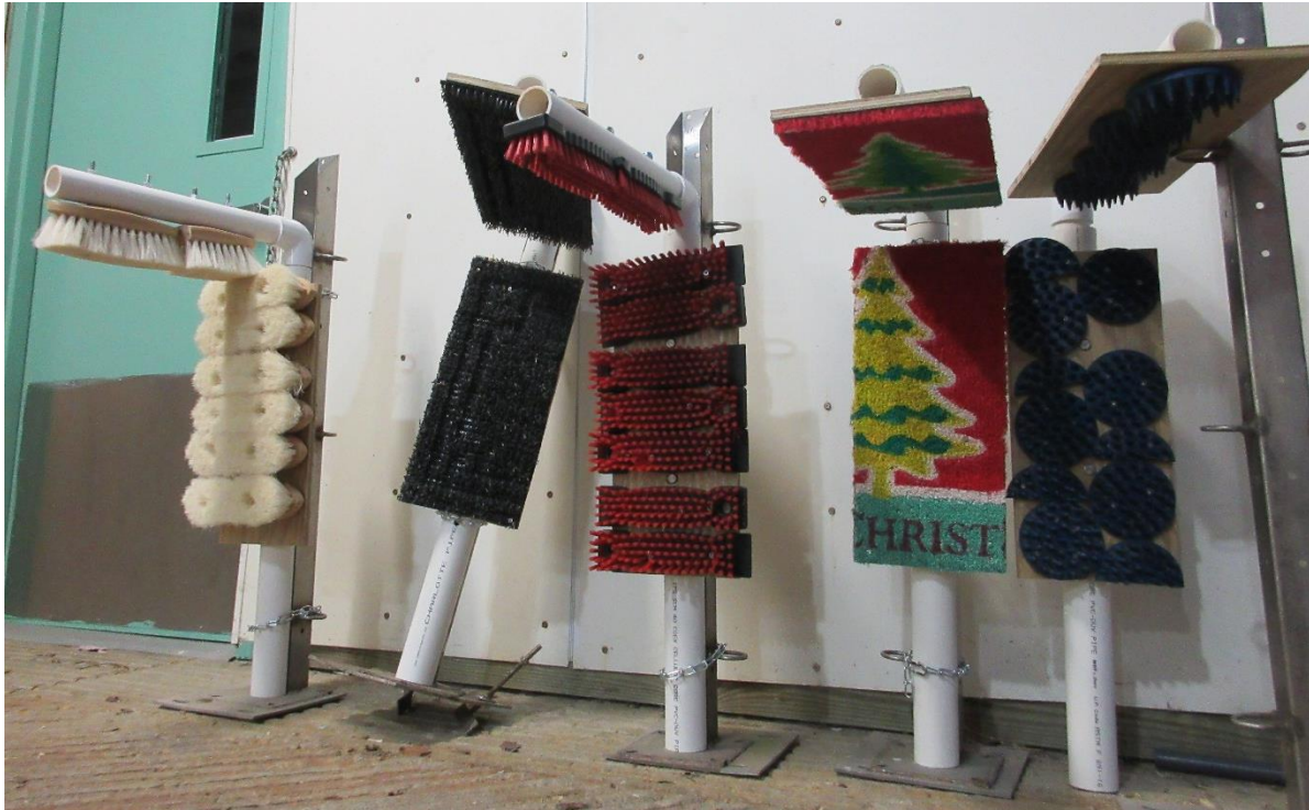
Figure 2.2. Five scratch post enrichments were created using polyvinyl chloride pipe (PVC), nuts, bolts, chain, screws, and different scratching materials for Exp. 1. Left to right, materials used were: 1) white, soft, long-bristled brushes (5.08 cm bleached tampico, Decker Manufacturing Co., Keokuk, IA); 2) black, short-bristled, astro-turf-like mat (45.72 cm x 76.20 cm, Clean Machine Metro Entrance Mat, Grass Worx, St. Louis, MI); 3) red, hard, short-bristled brush (3.18 cm recycled fiber bristles, Libman, Arcola, IL); 4) coir, hard, short-bristled mat (45.72 cm x 72.20 cm, Meijer, Inc., Grand Rapids, MI); and 5) blue, plastic, large-round-bristled combs (Oster Equine Care Series, Boca Raton). They were made in an L shape so that the top arm of the post could move up and down.
