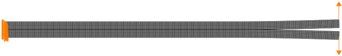
Fig. 5.2. Finite element model for the DCB specimen.
