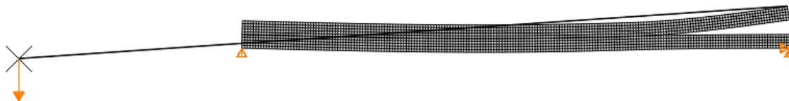
Fig. 5.6. Sample finite element model for a MMB specimen.
