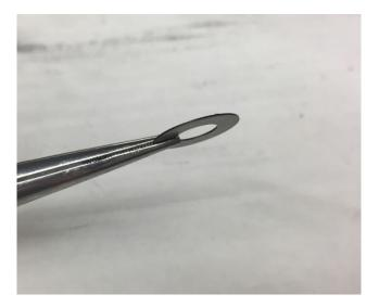
Fig. 6.1 A positive temperature coefficient device retrieved after disassembly from an overcharged 18650 Li-ion cell.
