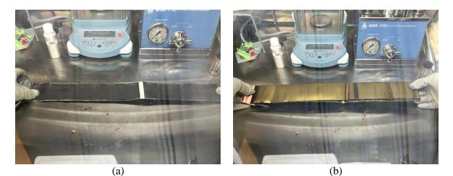
Fig. 6.10 Electrodes from a fresh cell subjected to the Overcharge test. (a) Cathode, and (b) anode.
