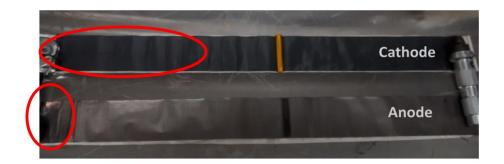
Fig. 5.11 Dried electrodes sheet after external short test.
