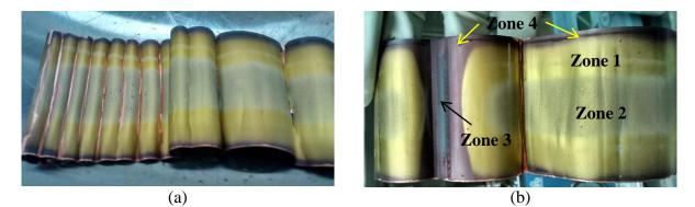
Fig. 5.22 DPA of Cell R20. Close up to the graphite electrode. (a) Electrode near to the center of the cell. (b) Different zones found in the electrode.
