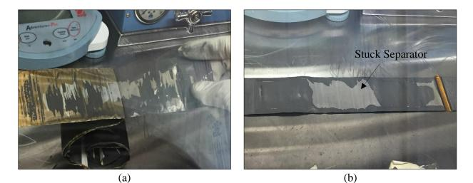
Fig. 6.12 (a) Cathode material coming out of the electrode and getting stuck on the separator. (b) Melted separator stuck on the cathode material.
