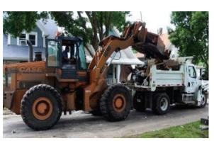
(a) Self-loader truck Figure 2-3 Types of debris collection equipment
