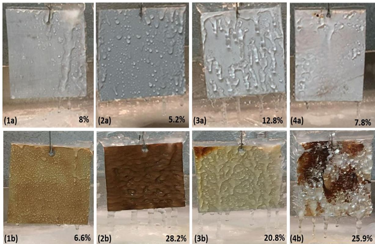
*Figure 3.5 Ice accumulation test images of the unaged and heat aged test panels. (1a & 1b) smooth fluoro coating, (2a & 2b) silicone epoxy coating, (3a & 3b) silica-filled fluoro coating and (4a & 4b) fluoro silane aerosol coating.*
