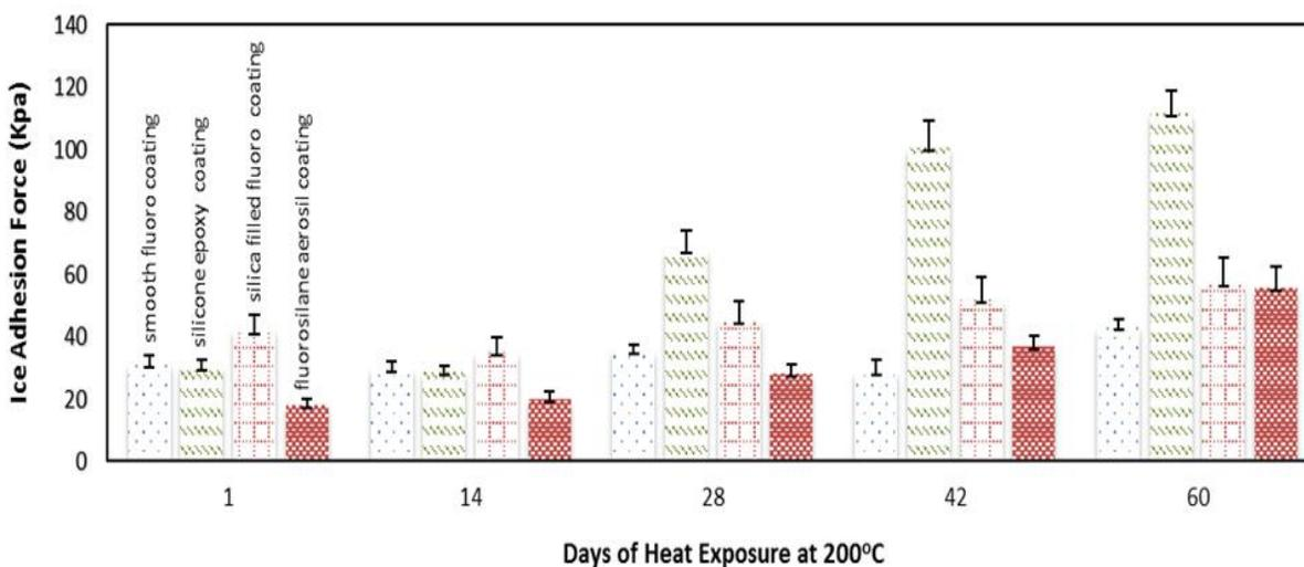
*Figure 3.6. Ice adhesion force of the coatings tested at frequent intervals during heat ageing study at 200 °C.*
