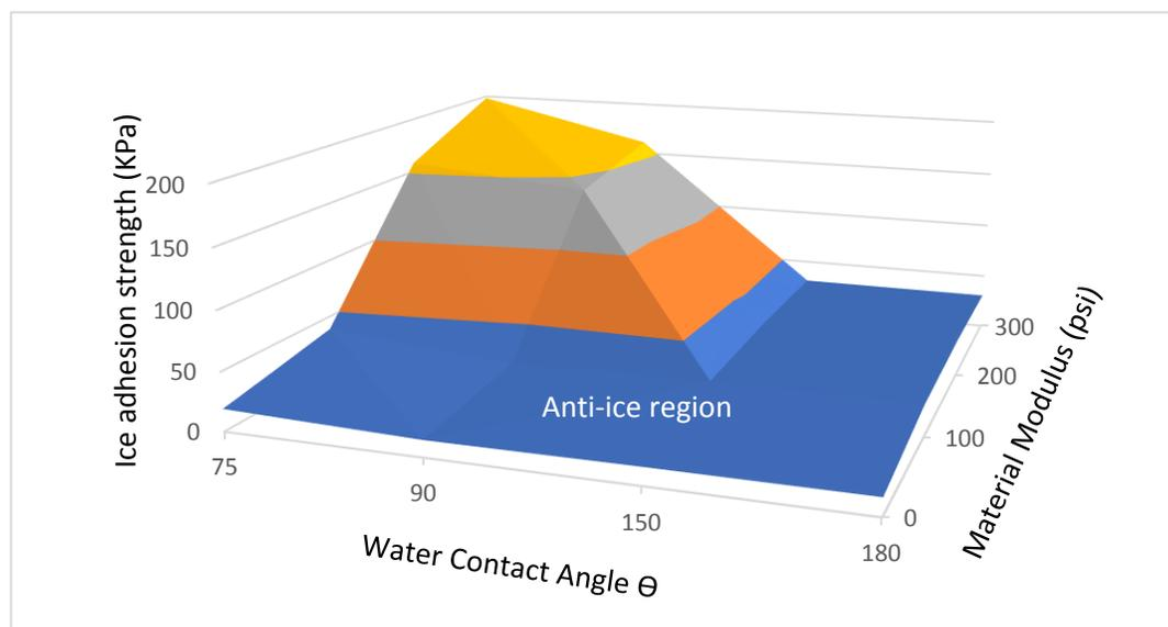
Figure 4.9. Schematic representation of material design space to ice achieve low ice adhesion
