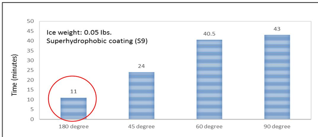
Figure 5.7. Time taken to accumulate 0.05 lbs. weight on superhydrophobic surfaces with sample placement angle ( $180^\circ$ ,  $45^\circ$ ,  $60^\circ$  and  $90^\circ$ ) against water spray direction
