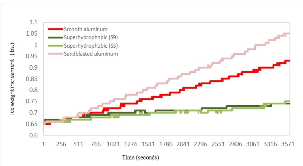
Figure 5.3. Ice accumulation weight increase data of superhydrophobic coatings
