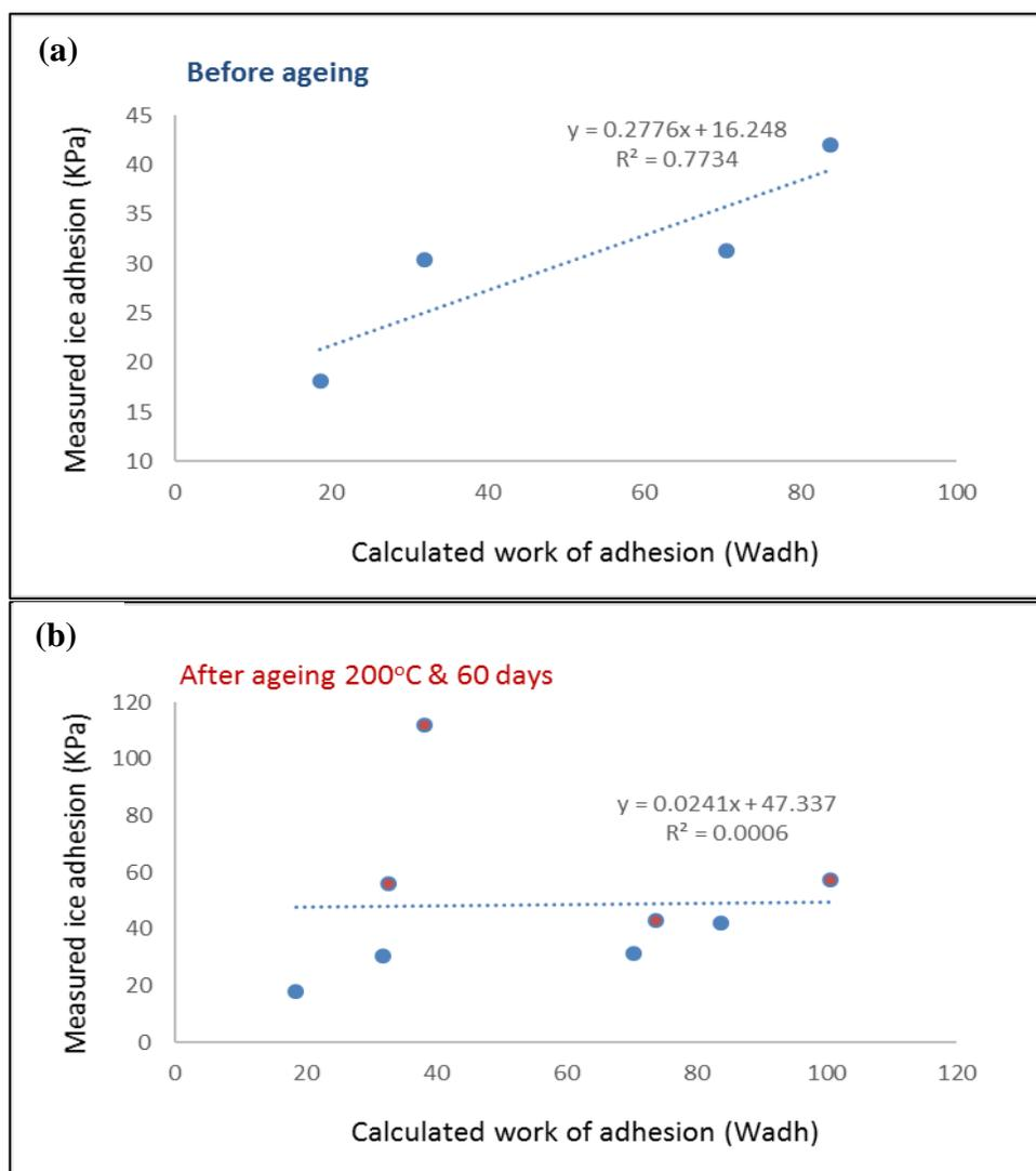
Figure 3.7. (a) Calculated work of adhesion of unaged coated panels, (b) Calculated work of adhesion of unaged and aged coated panels
