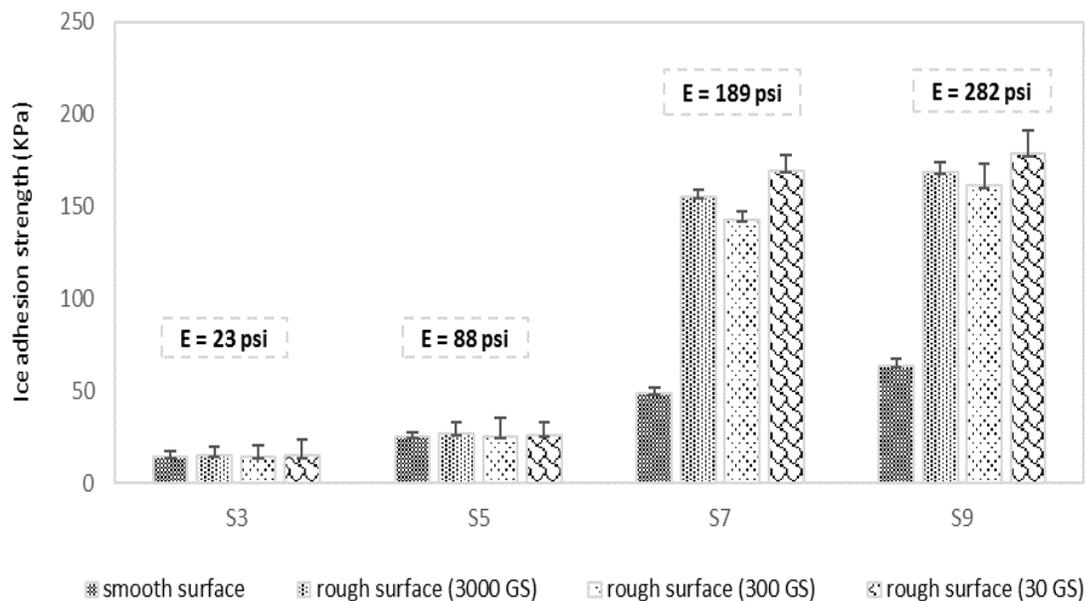
*Figure 4.5. Ice adhesion strength of low to high modulus (S3, S5, S7, and S9 respectively) silicone coatings with smooth and rough surfaces; Elastic modulus (E) values are mentioned inside the graph*
