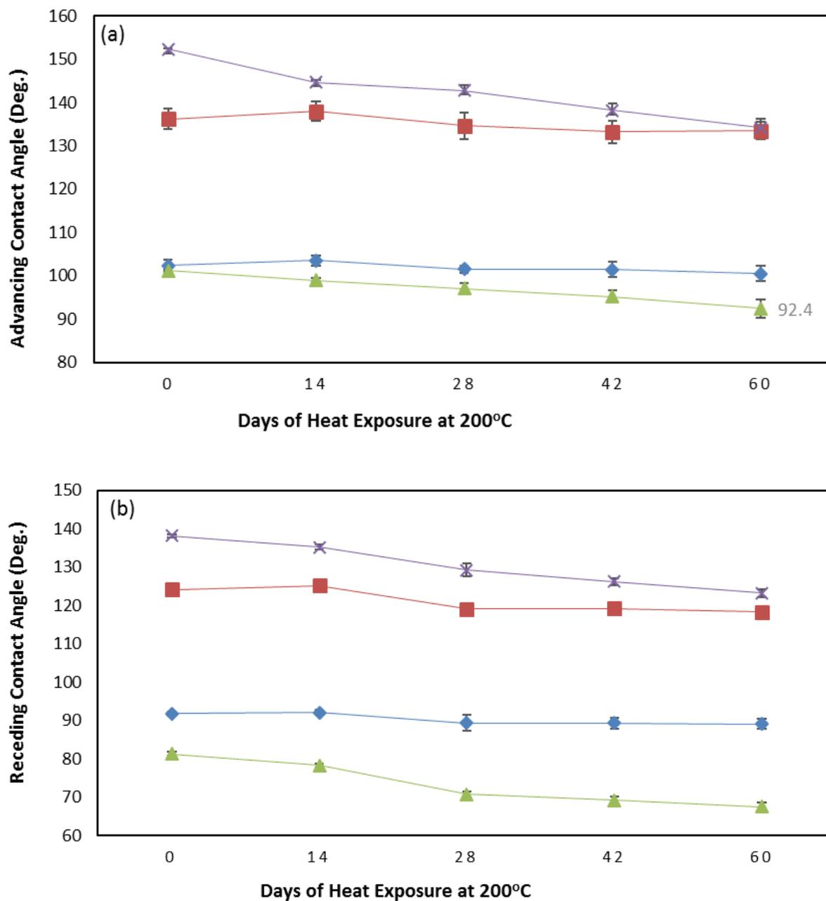
Figure 3.3. Water contact angle test data of coated test panels. (a) advancing contact angle and (b) receding contact angle. ♦ smooth fluoro coating, ▲ silicone epoxy coating, ■ silica-filled fluoro coating and x fluorosilane aerosol coating
