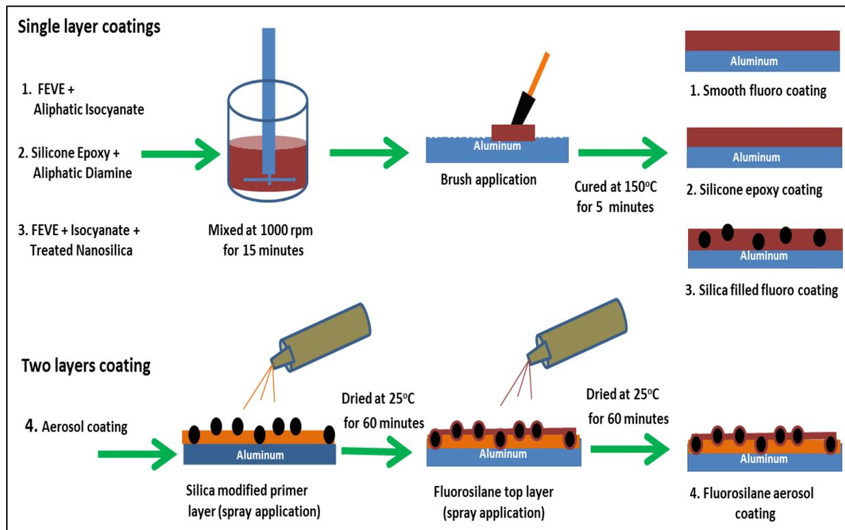
Figure 3.1. Schematic representation of coated test panel preparation steps.
