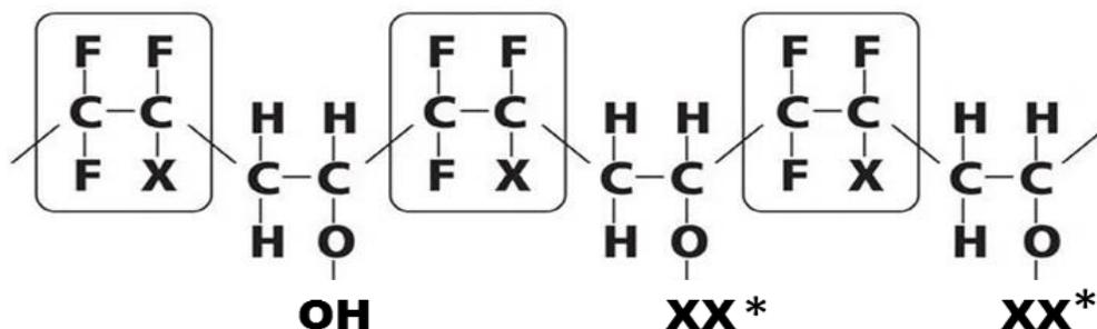
Figure 2.1. Chemical Structure of Fluoro-Ethylene-Alkyl-Vinyl-Ether (FEVE),
