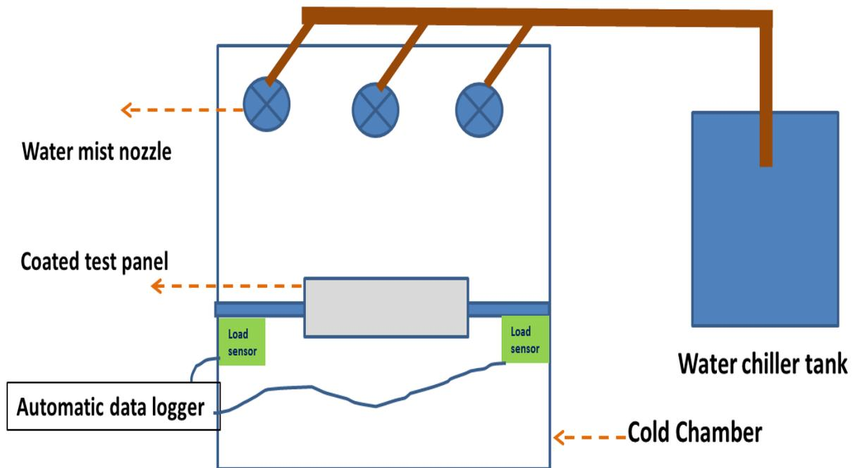
Figure 2.3. Schematic representation of automated ice accumulation measurement set-up
