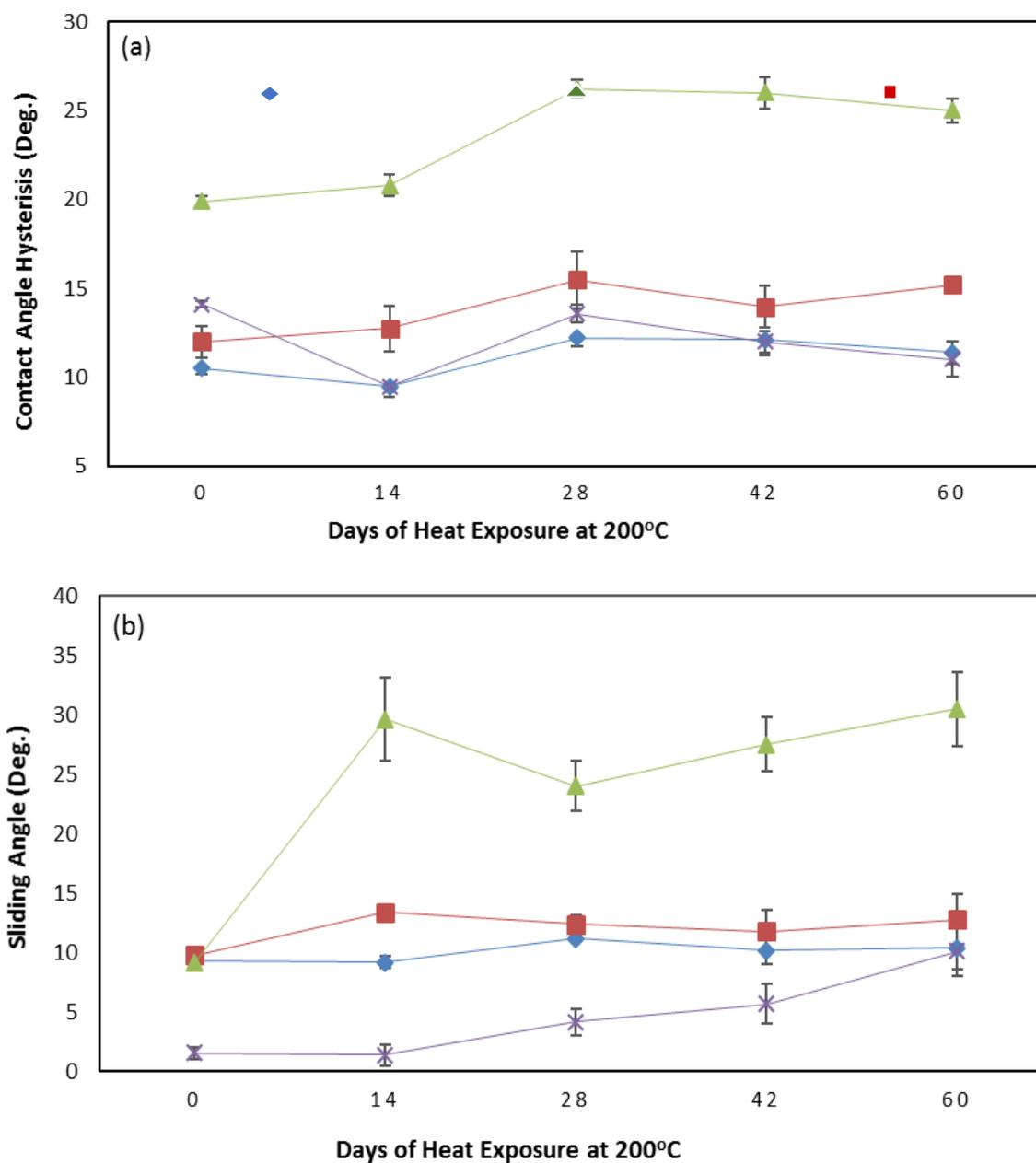
Figure 3.4. Water contact angle test data of coated test panels. (a) contact angle hysteresis and (b) water sliding angle. ◆ smooth fluoro coating, ▲ silicone epoxy coating, ■ silica-filled fluoro coating and × fluorosilane aerosol coating
