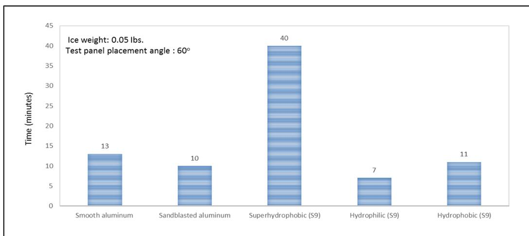
Figure 5.8. Time taken to accumulate 0.05 lbs. weight on all the test panels with sample placement angle of  $60^\circ$  against water spray direction
