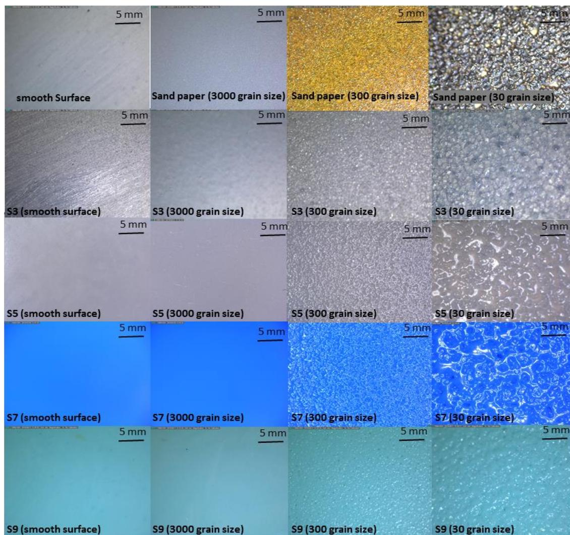
Figure 4.4. Optical images of sand paper and silicone samples
