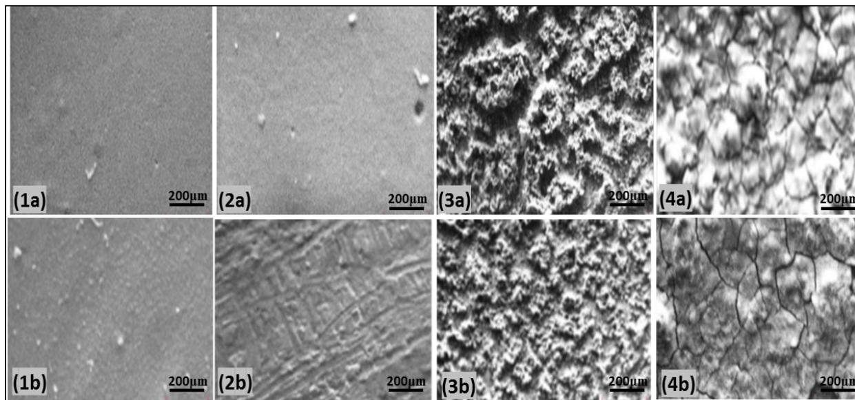
Figure 3.2. SEM images of the unaged (top images) and heat aged (bottom images) coated test panels for 200°C for 60 days; (1a & 1b) smooth fluoro coating, (2a & 2b) silicone epoxy coating, (3a & 3b) silica-filled fluoro coating and (4a & 4b) fluorosilane aerosol coating.
