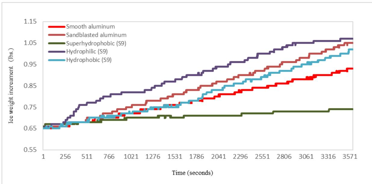
Figure 5.5. Ice accumulation weight increase data of high modulus (288 psi) coatings
