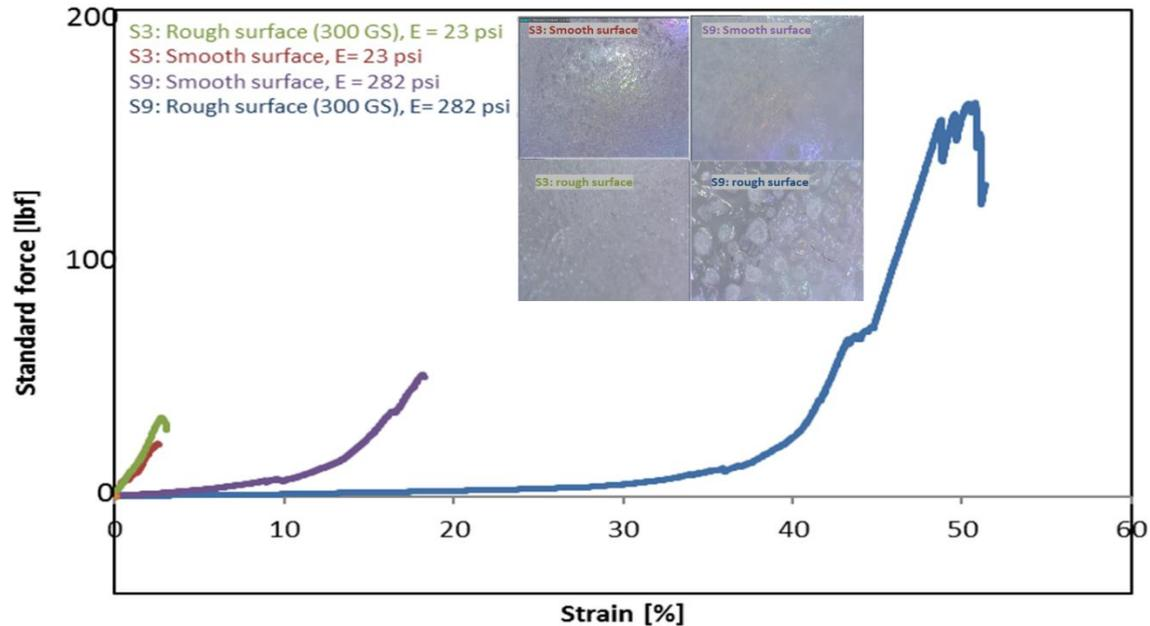
Figure 4.6. Ice adhesion test stress – strain curve and images of the ice after the test
