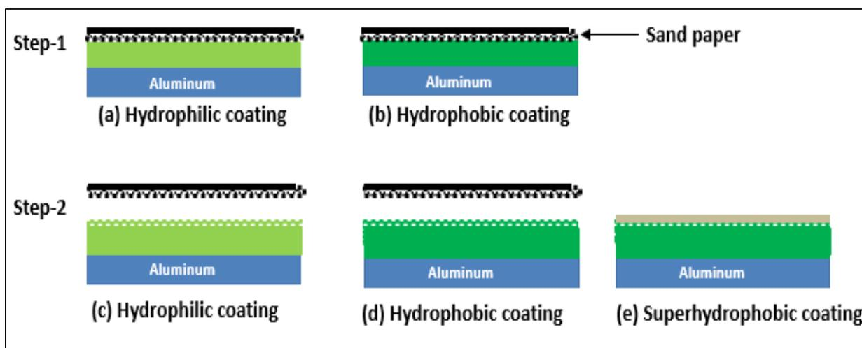
Figure 4.2. Illustration of rough surface test panels preparation steps
