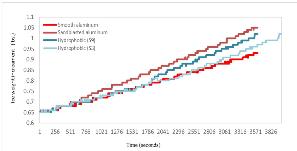
Figure 5.2. Ice accumulation weight increase data of hydrophobic coatings
