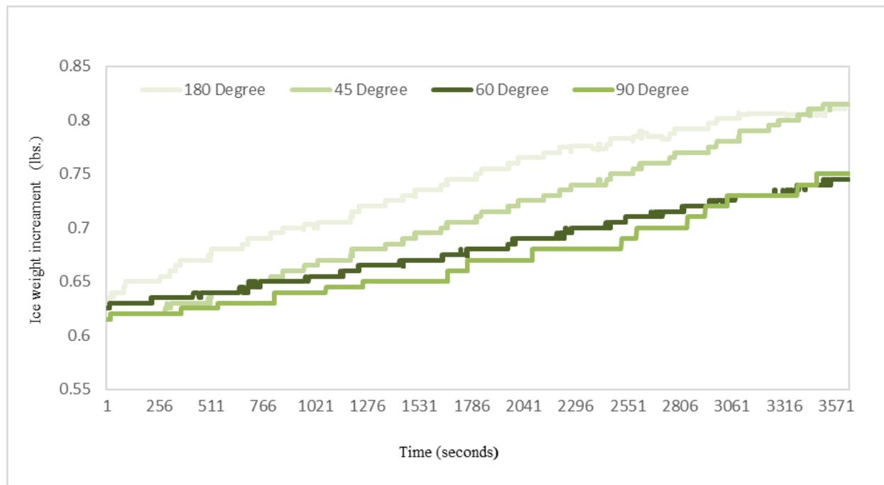
*Figure 5.6. Ice accumulation weight increment of different sample placement angle (180°, 45°, 60° and 90°) against water spray direction*
