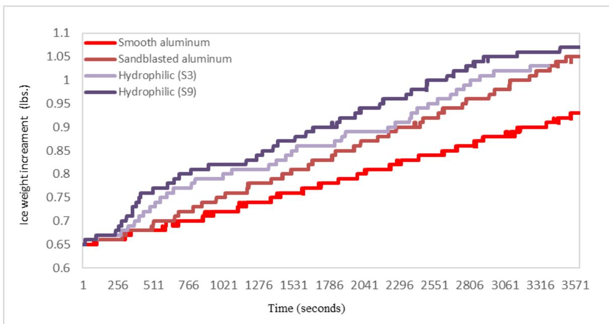
Figure 5.1. Ice accumulation weight increase of hydrophilic coatings
