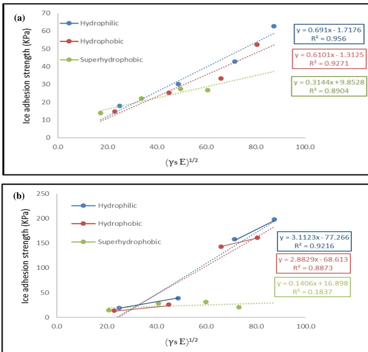
Figure 4.8. (a). Baier's adhesion plot for smooth surfaces, (b). Baier's adhesion plot for rough surfaces
