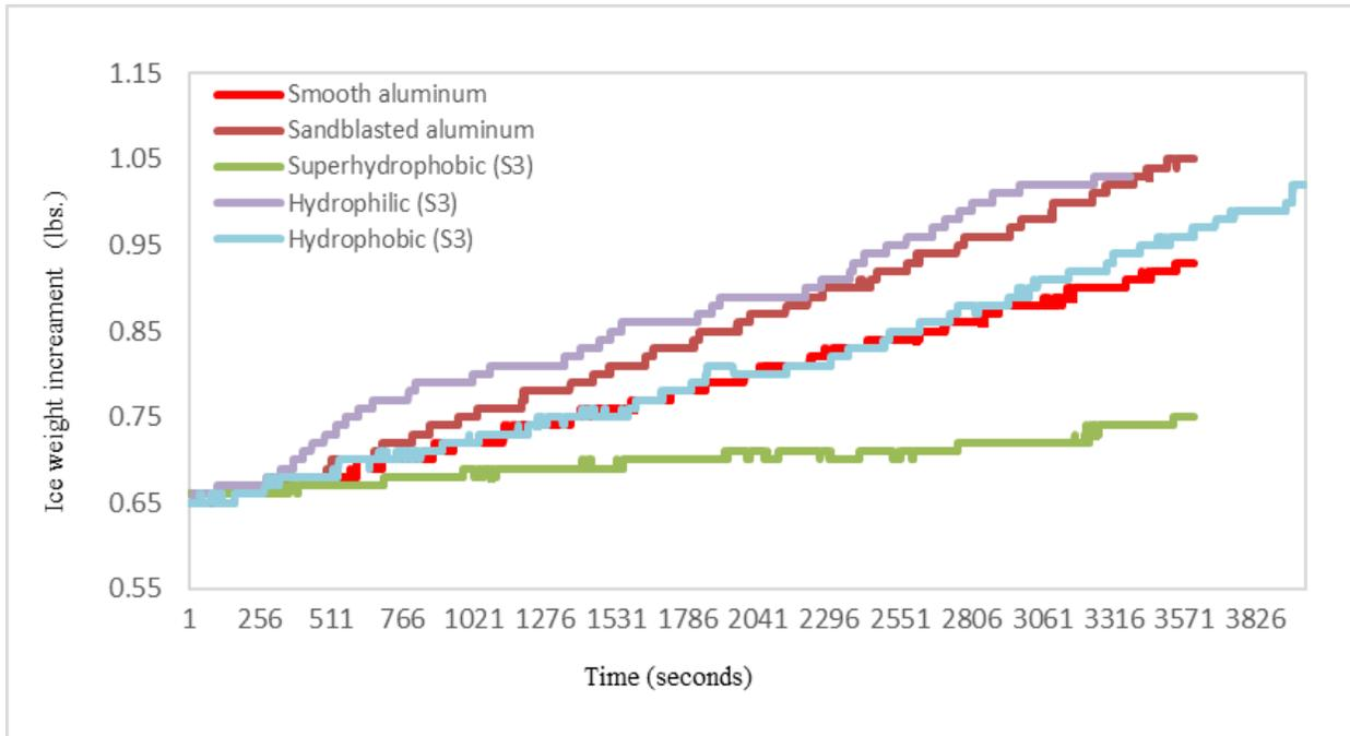
Figure 5.4. Ice accumulation weight increase data of low modulus (23 psi) coatings
