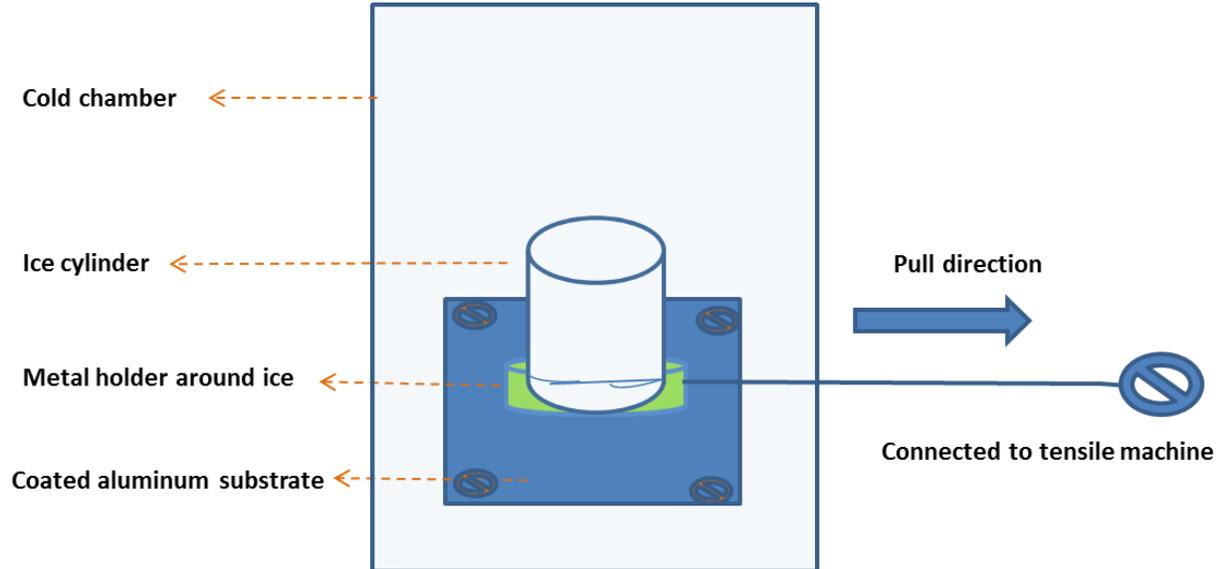
*Figure 2.2. Schematic representation of ice adhesion strength test set-up*
