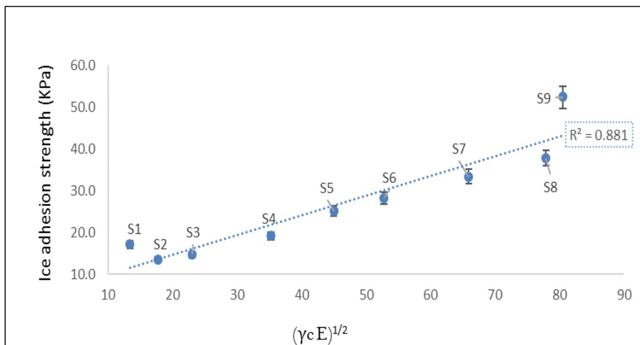
Figure 4.3. Combination influence of coating modulus and surface energy to ice adhesion strength
