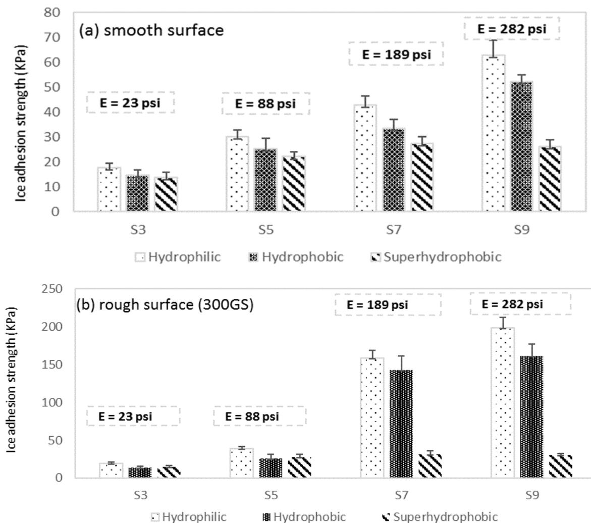
Figure 4.7. (a) Ice adhesion strength of smooth hydrophilic, hydrophobic and superhydrophobic surfaces, (b). Ice adhesion strength of rough hydrophilic, hydrophobic and superhydrophobic surfaces
