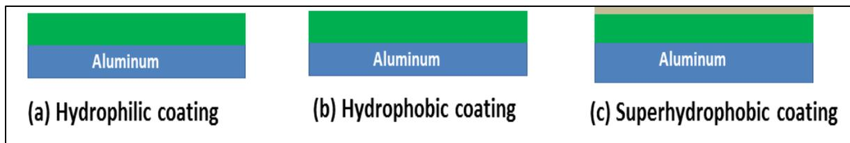
Figure 4.1. Illustration of smooth surface test panels
