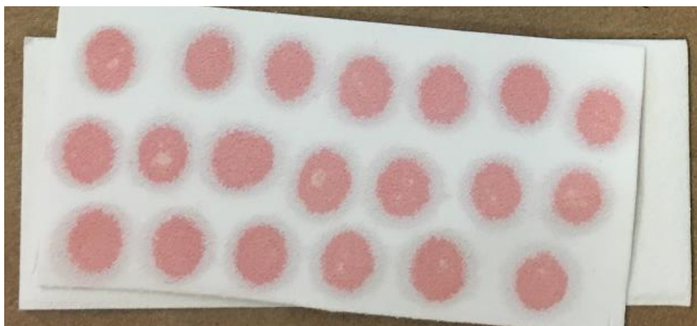
Figure 6.5 Plasma separation with VPM.
