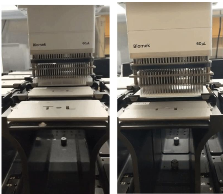
Figure 1.2. Pintool dips into well plate (left), prints onto PTFE plate (right).
