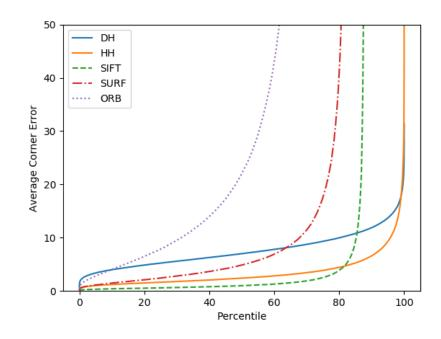
Fig. 4.9.: Sorted ACE for Occlusion  $\alpha = 0.4$ . This figure depicts performance of each method using sorted ACE values, by least to greatest. ORB is the only method significantly impacted by occlusions affecting 40% of the pixels in the warped patch. ORB exceeds an ACE of 50 for nearly half the dataset as a result, while the other methods remain near their levels at ideal conditions.
