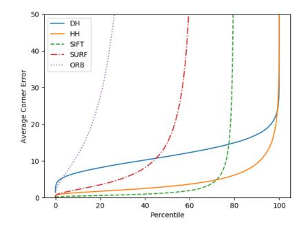
Fig. 4.10.: Sorted ACE for Occlusion  $\alpha = 0.6$ . This figure depicts performance of each method using sorted ACE values, by least to greatest. With over half of the warped patch removed due to occlusion, SIFT has the lowest ACE for nearly 80% of the dataset. The deep learning methods also experience relatively little change compared to ideal conditions. The impact on ORB is the most significant, as ORB is now viable for less than 20% of the dataset.
