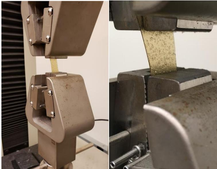
**Figure 16.** Tensile test specimen under traction.
