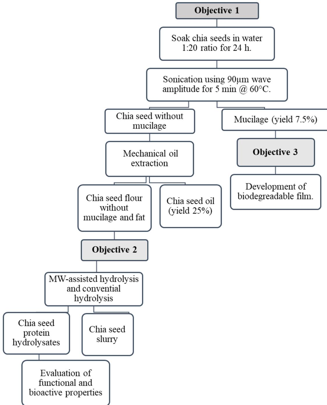
**Figure 1.** Flowchart for the development of chia seed protein hydrolysates.
