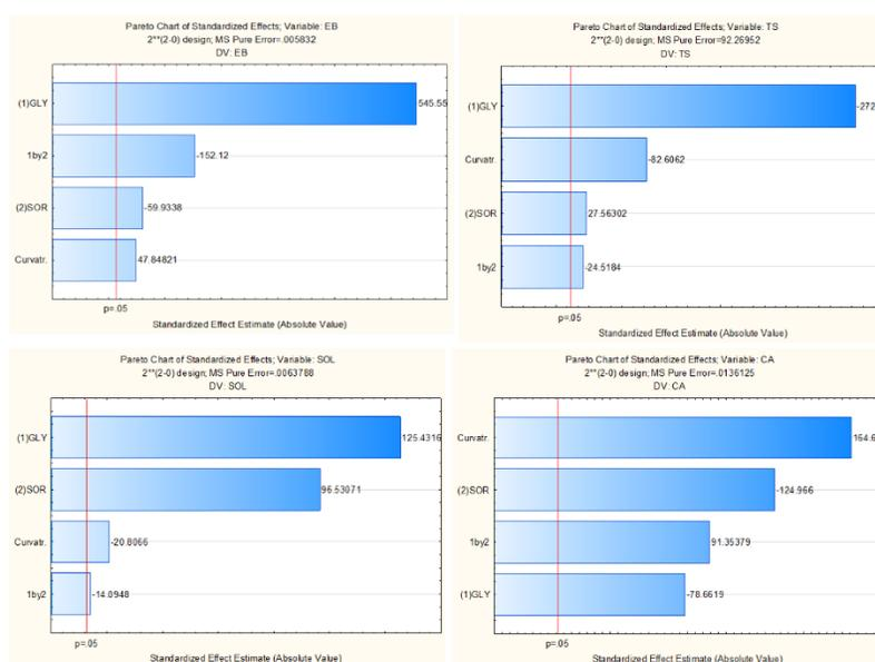
**Figure 22.** Pareto charts, significance effect of polyol and their interaction on mechanical and barrier properties of CSM films.
