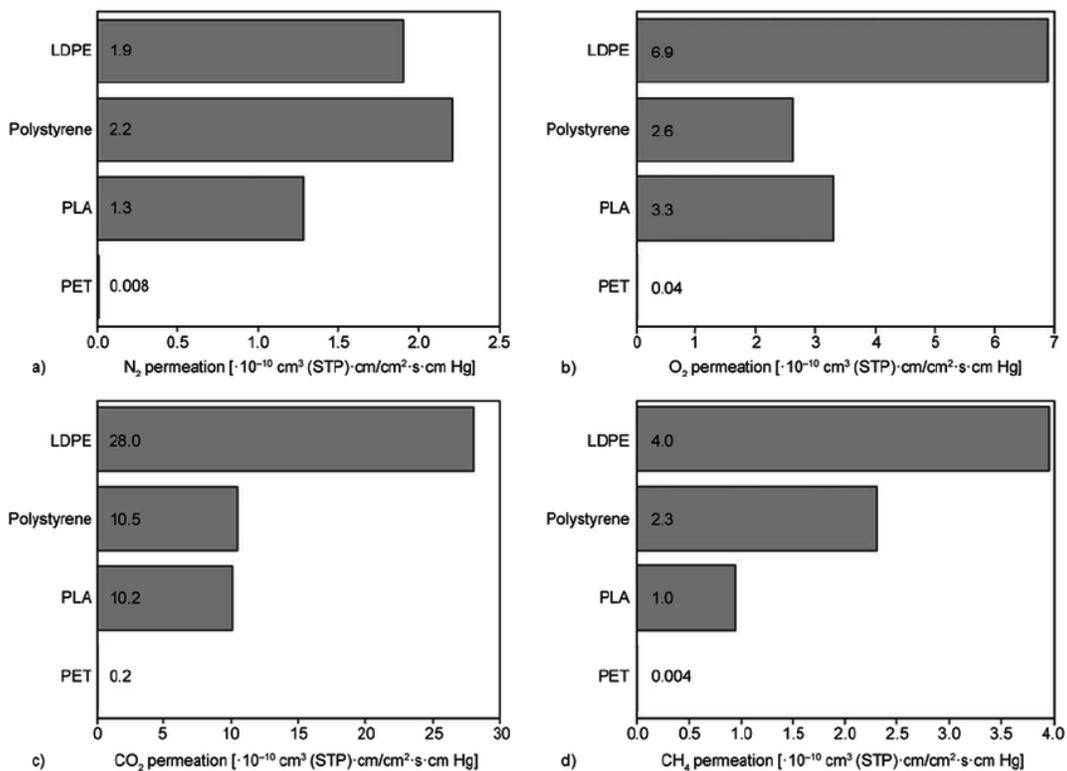
**Figure 9.** Barrier properties of PLA compared to conventional polymers at 30~C for (nitrogen, oxygen, Carbon dioxide and Methane) (Hamad et al., 2015).
