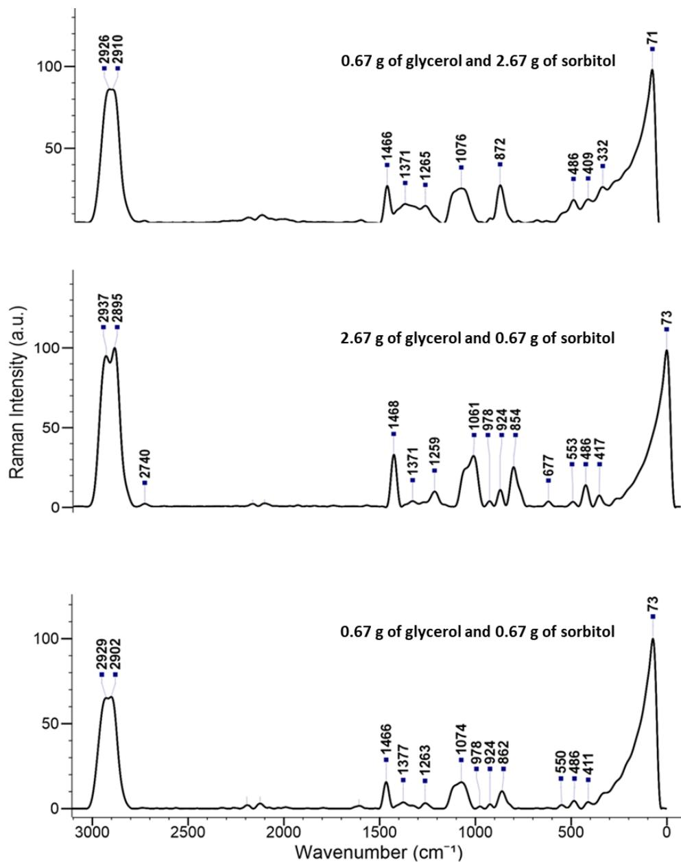
**Figure 19.** Raman spectra for edible films from chia seed mucilage at different polyol concentrations
