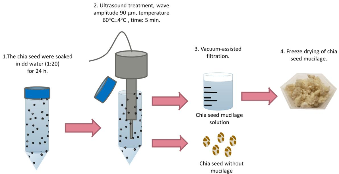
**Figure 10.** Diagram of mucilage separation (extraction) from chia seeds using ultrasonication and vacuum-assisted filtration.
