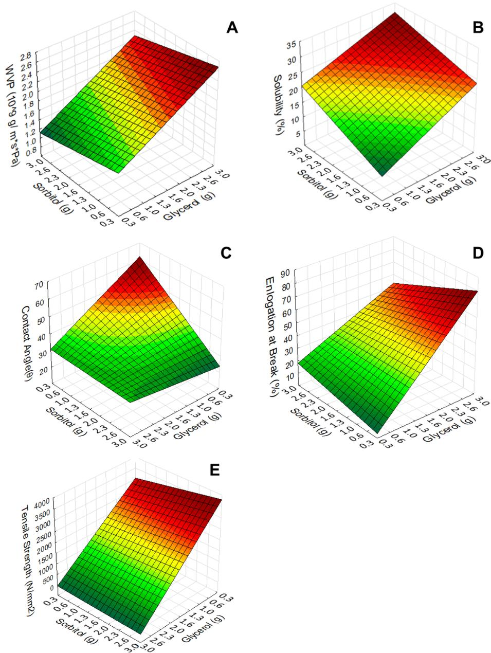
**Figure 17.** Response surface diagrams; Effect of glycerol (g) and sorbitol (g) per gram of chia seed mucilage (CSM) on the response variables: water vapor permeability (A), solubility (B), contact angle (C), elongation at break (D), tensile strength (E).
