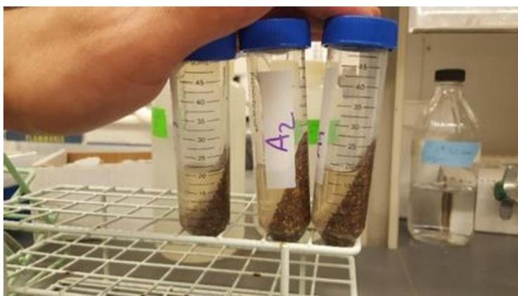
**Figure 24.** Centrifugation as a separation method for chia seed mucilage.
