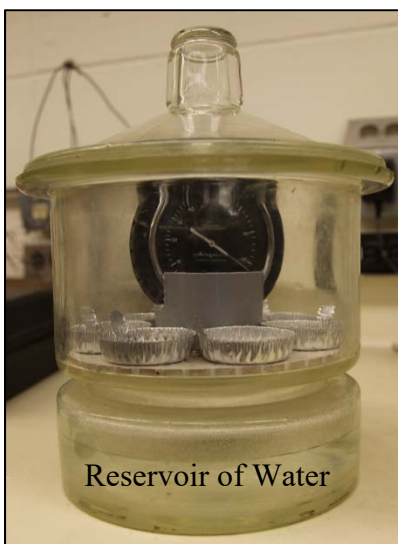
Figure 2.1. Atmospheric absorption test setup
