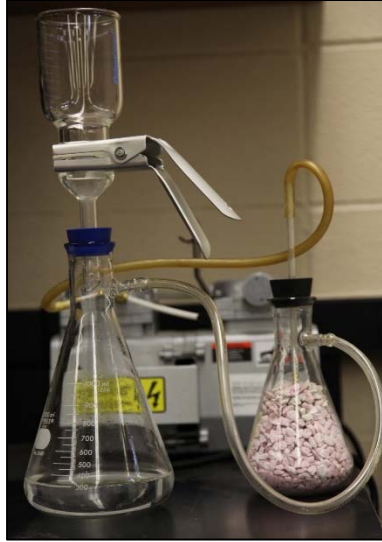
Figure 2.2. Vacuum filtration setup
