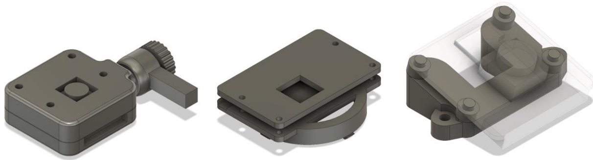
Figure 5. (Left) CAD model of camera housing and locking ball and socket joint. (Center) Raspberry Pi Zero W housing designed to mount on headphones. (Right) The wedge shaped camera mount for use with the HTC Vive.
