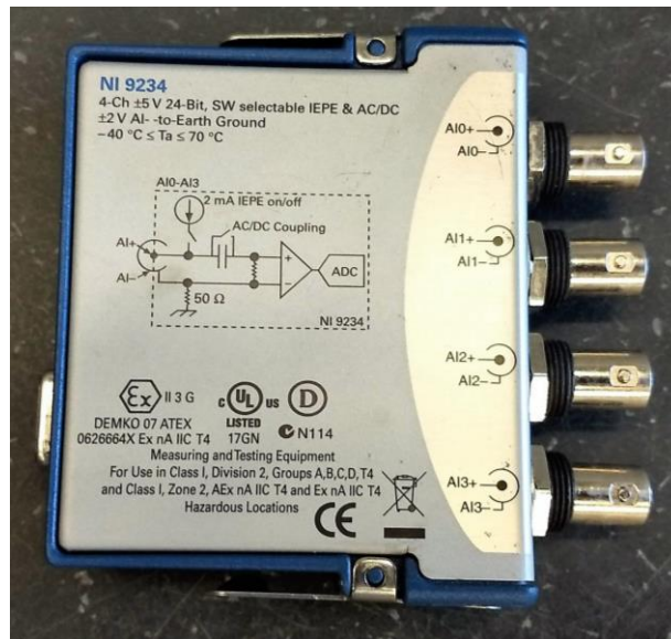
Figure 3.4 NI 9234 sound and vibration input module for collecting signal from accelerometer
