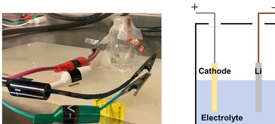
Figure 6.2 Scheme and photo for the two-electrode setup for electrochemical measurements.
