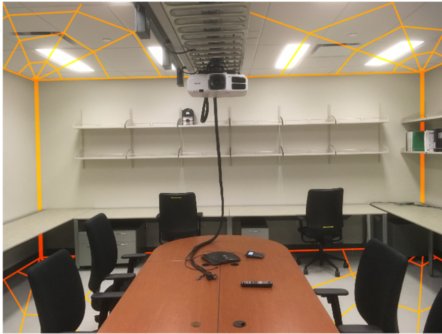
Fig. 4.3: Conceptual drawing demonstrating how two GLines could be placed at the two corners of the room. The figure displays the ground planes as wire meshes.
