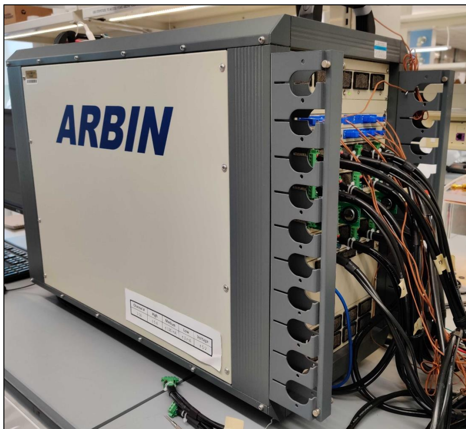
Fig 3.3: Arbin Battery Tester used for electrochemical testing
