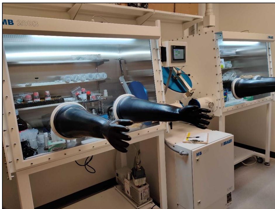
Fig 3.1: M-Braun Glovebox used to conduct coin cell fabrication, destructive physical analysis, and Optical Microscopy
