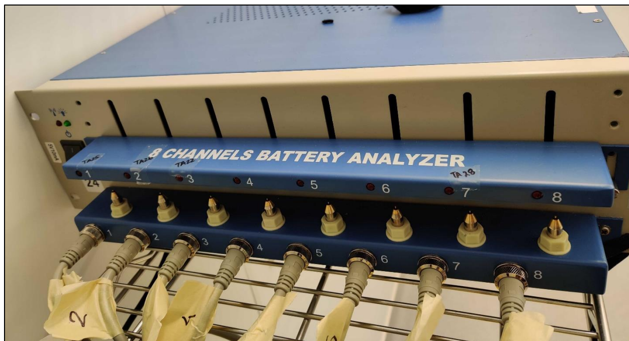
Fig 3.4: MTI BTS8-3 coin cell cyler used for Electrochemical Testing
