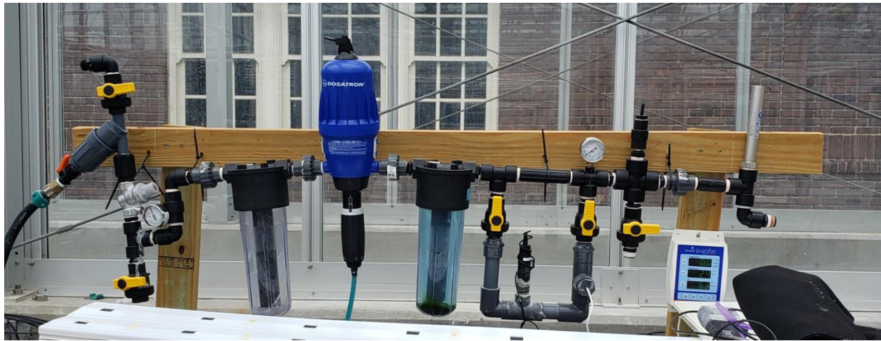
Figure 2.4: Picture of Dosatron which was assembled to mix together fertilizers at accurate concentrations.
