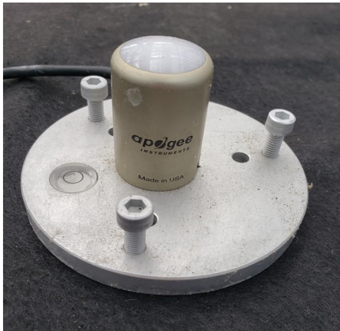
Figure 2.6: Image of the quantum sensor used to measure light intensity
