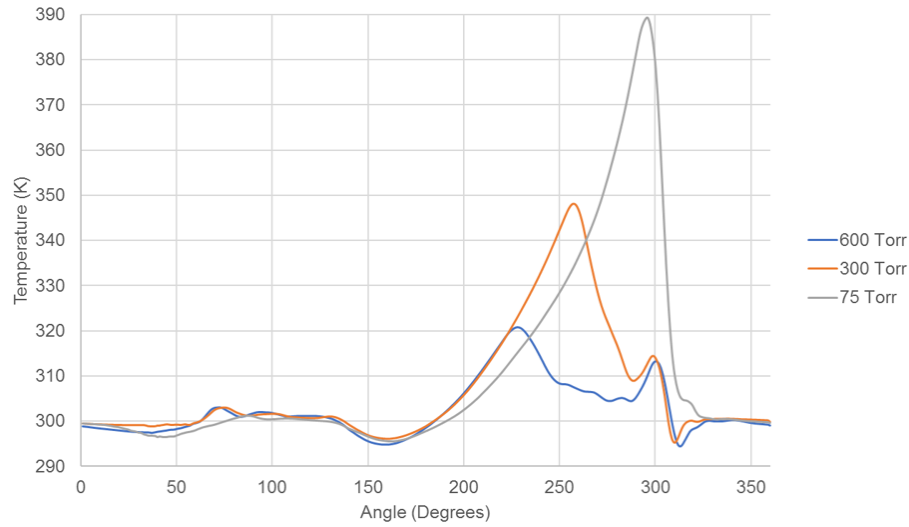
Fig. 4.26. Volume averaged air temperature in a region between the blades with angular coordinate (similar to Fig. 5.12) for P_{in}=600 , 300, 75 Torr for \omega=1750 RPM
