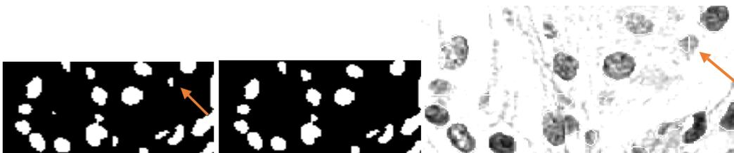
Figure 20. Before and after small region removal, and the display of removed region on raw image
