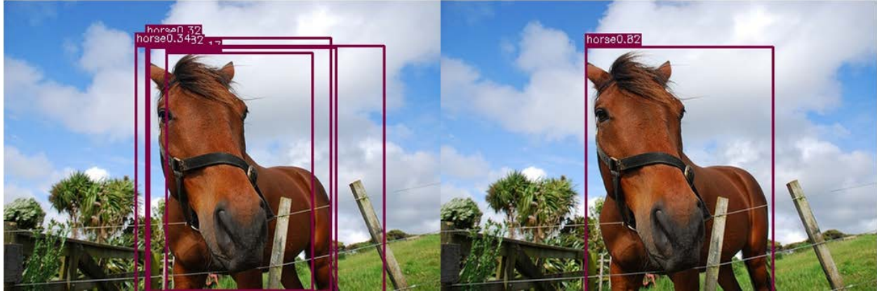
Figure 3.6 The Non-maximum example. The multiple bounding boxes (left), the optimal bounding box (right).
