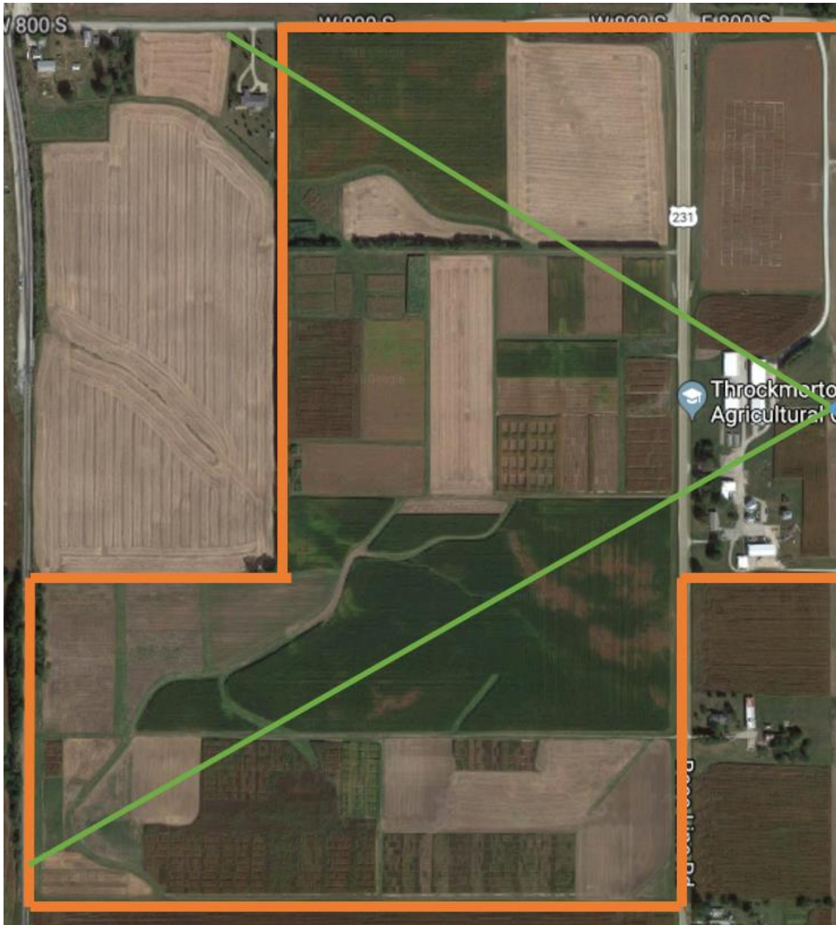
Figure 3.2: Terrawave 65° Degree Antenna Coverage
