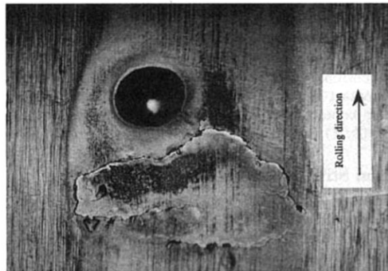
Figure 6.3: Experimental result for a dent-initiated spall in a dry contact [50]
