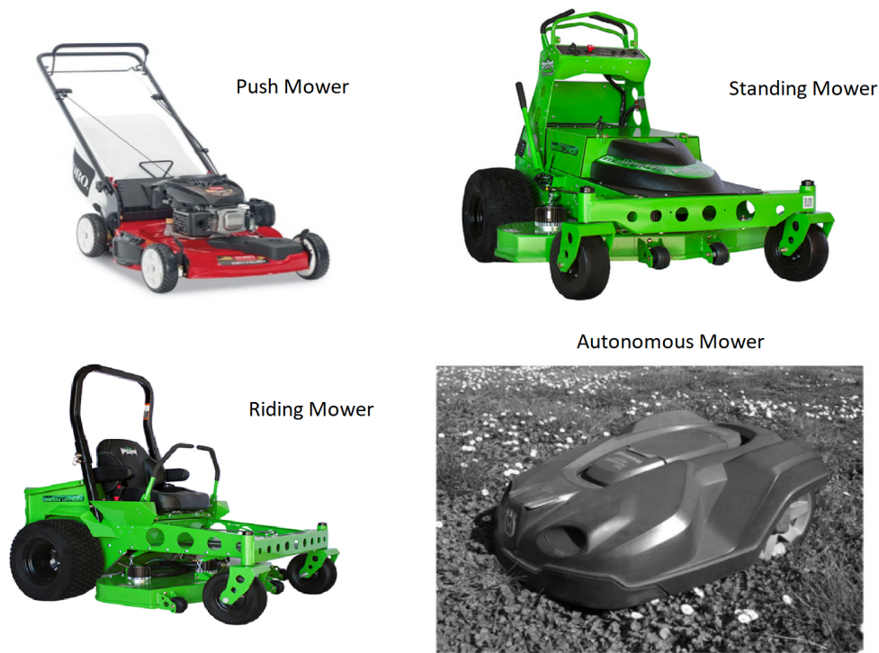
Figure 1.1. Mower classification based on operation mode
