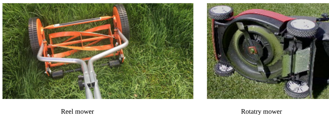
Figure 1.2. Mower classification based on blade rotation
