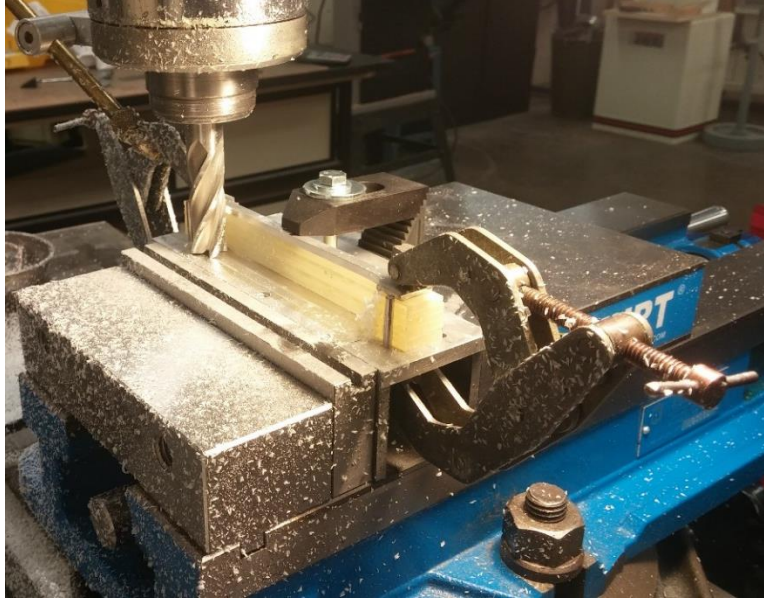
Figure 4.20. Machining of a stack of dogbone specimens
