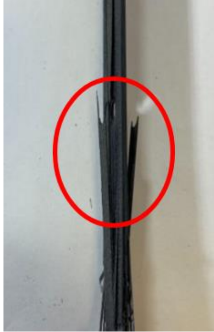
Figure 6.15: Delamination observed in [0_2 / \pm 45]_s laminate
