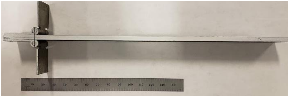
Figure 8.9: DCB specimen with hinges
