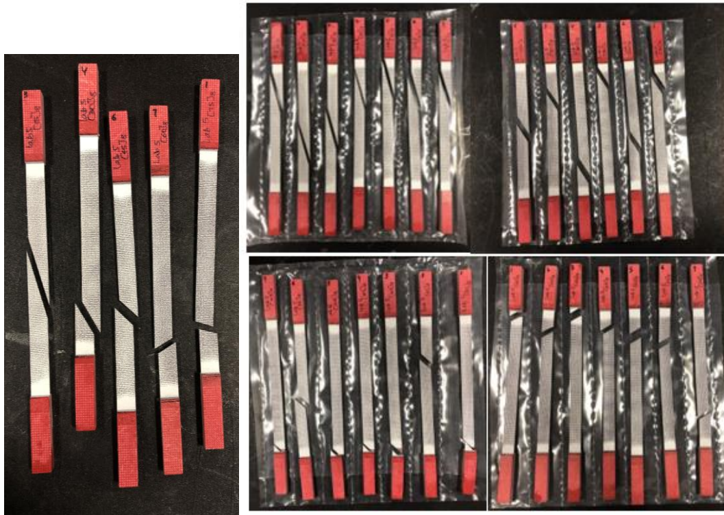
Figure 4.2: Failure angles of specimens
