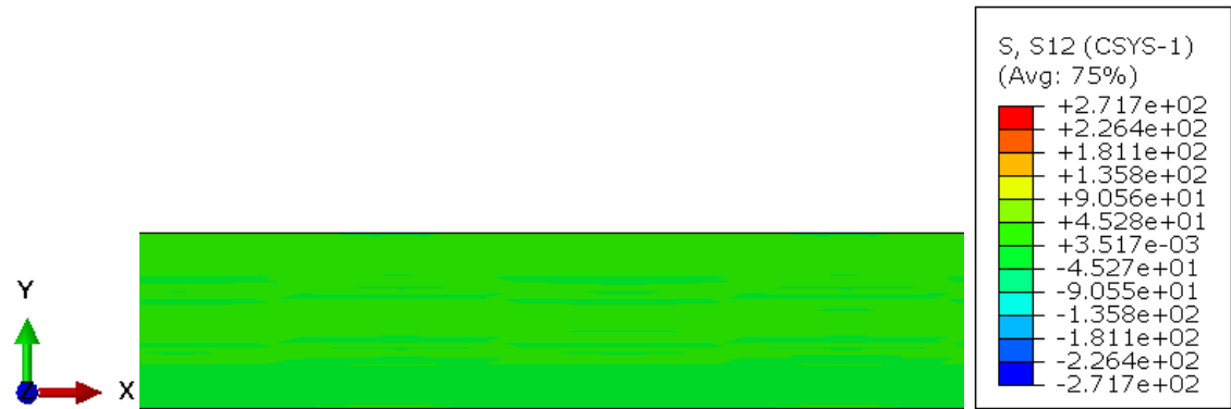
(ii) Interlaminar shearing stress \tau_{xz}
