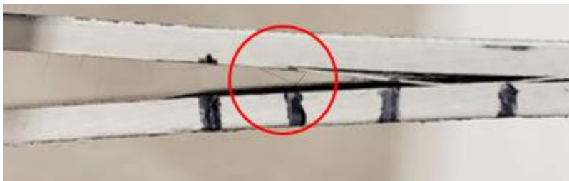
Figure 8.17: Fiber Bridging while testing the DCB samples
