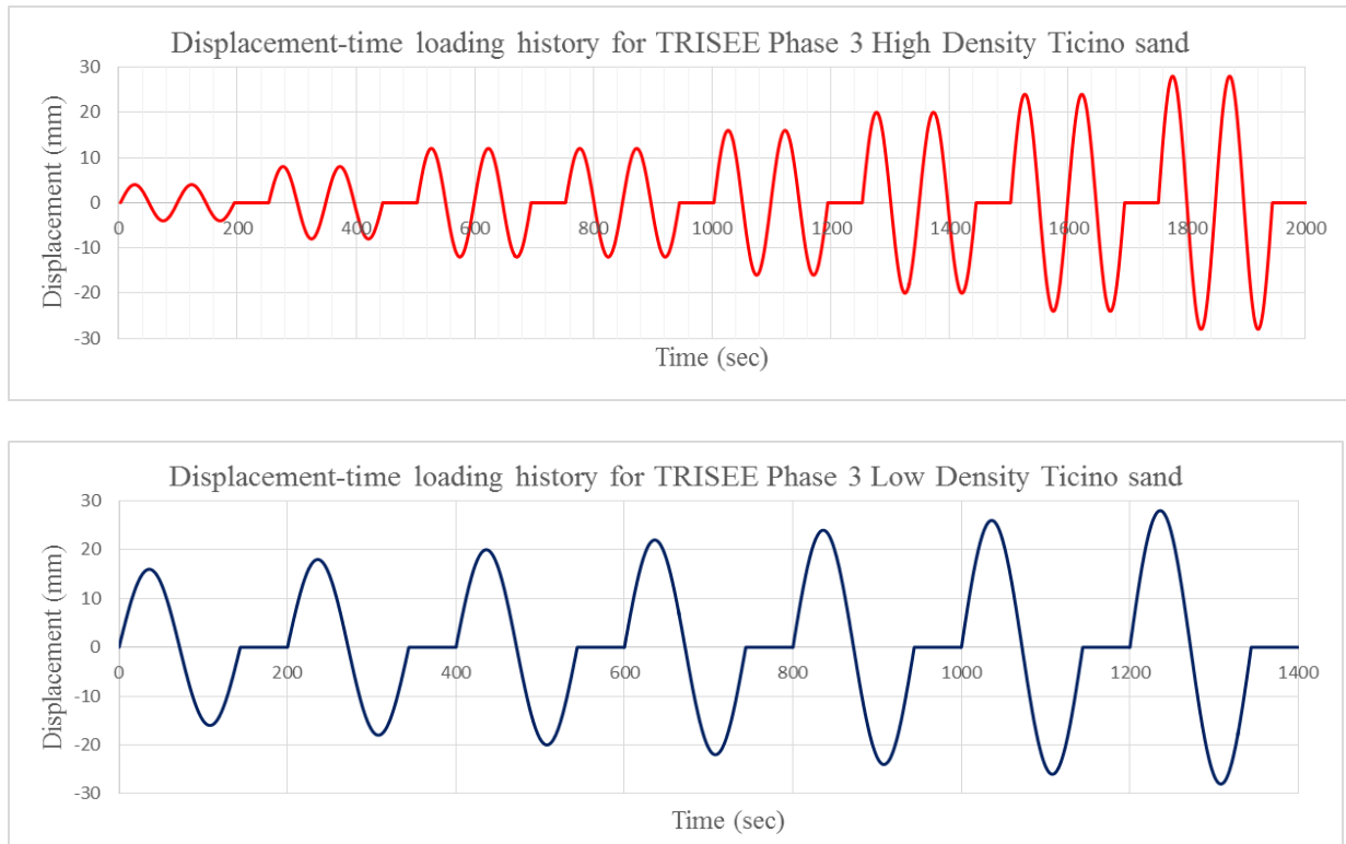
Fig 5.9: Displacement-time loading history for sliding of foundation on high density and low density Ticino sand
