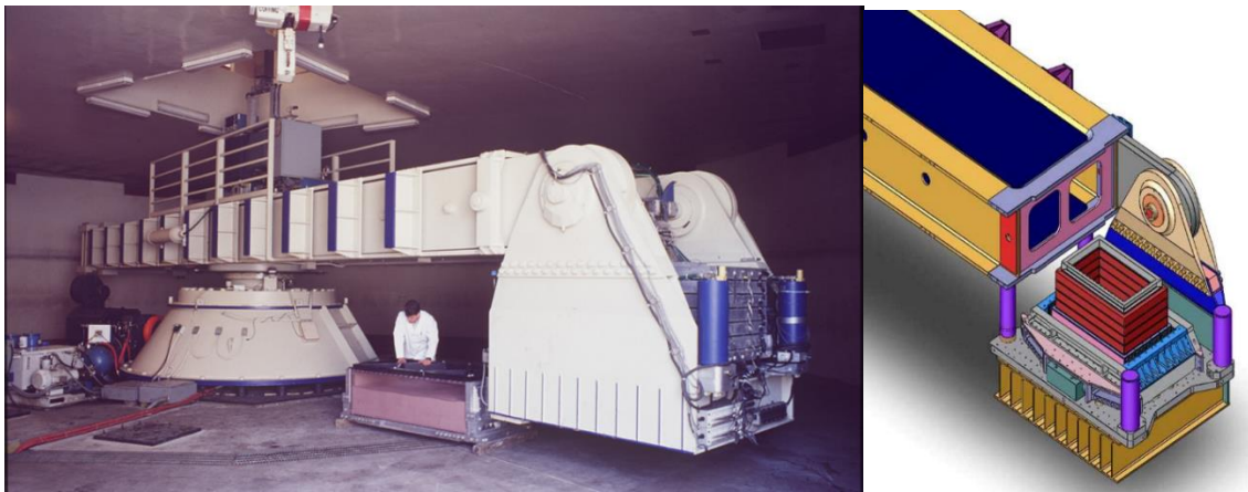
Fig 2.2: The NEES Centrifuge Facility at UC Davis supporting 2D seismic simulations in the vertical and horizontal direction
